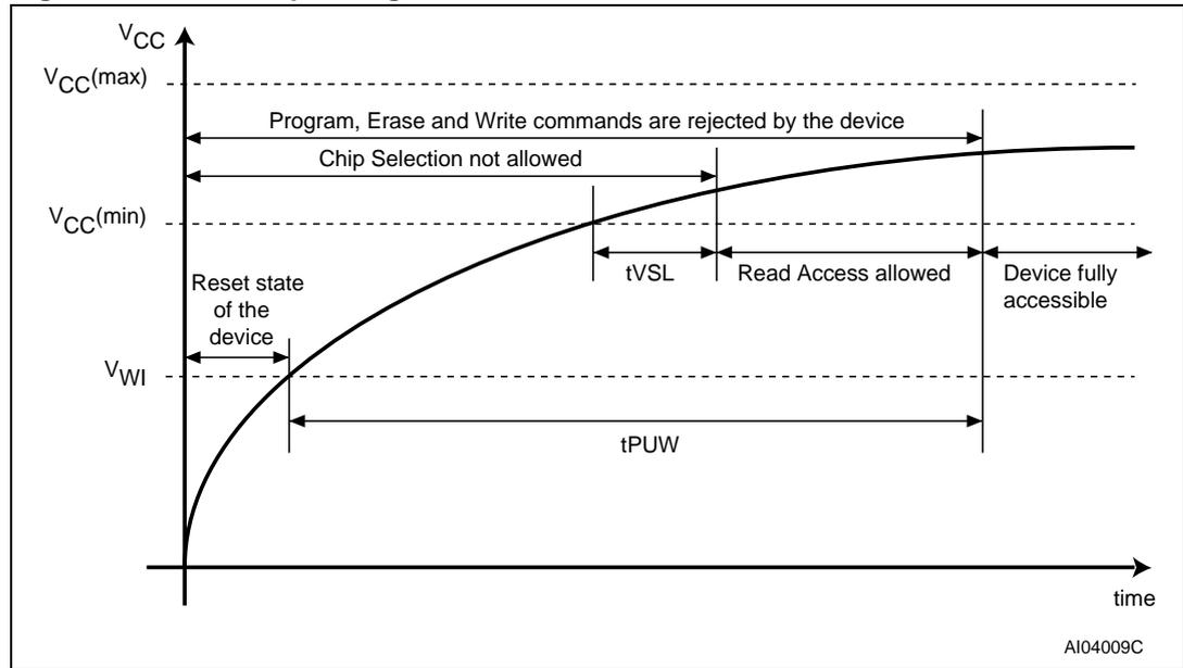
Table 11. Power-up timing and V<sub>WI</sub> threshold
