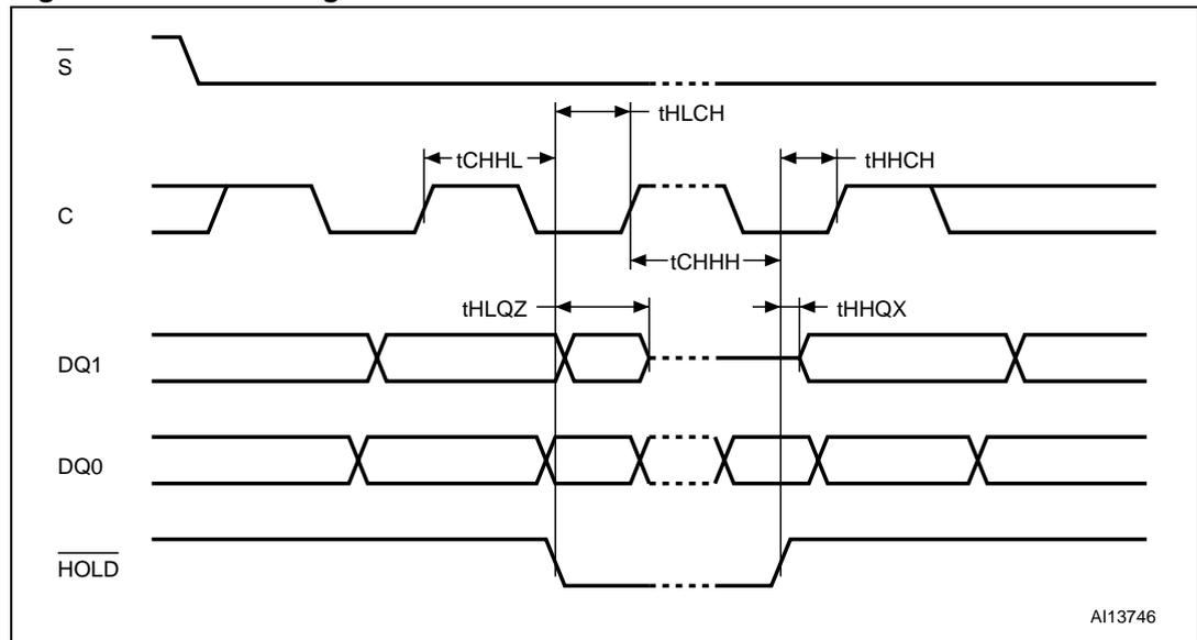
Figure 34. Output timing
