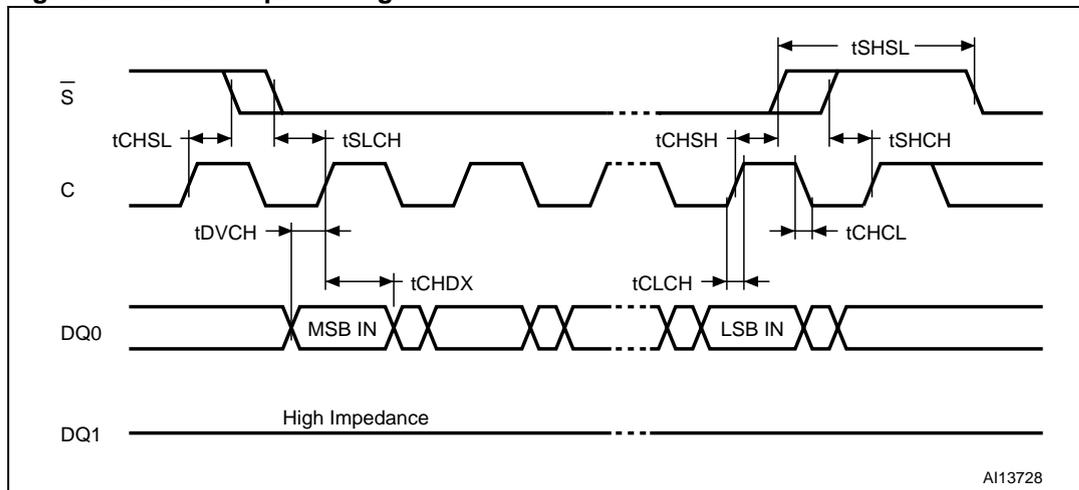
**Figure 32. Write Protect Setup and Hold timing during WRSR when SRWD=1**
