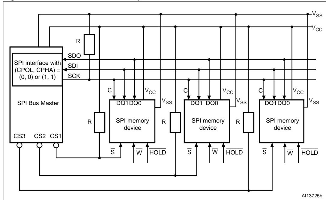
1. The Write Protect ( $\overline{W}$ ) and Hold ( $\overline{HOLD}$ ) signals should be driven, High or Low as appropriate.
