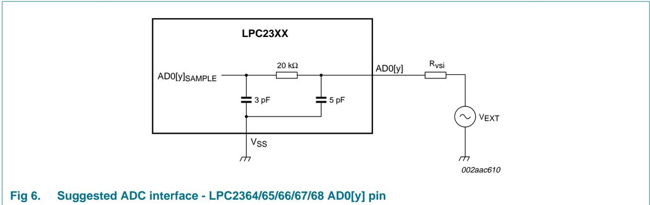
Fig 6. Suggested ADC interface - LPC2364/65/66/67/68  $AD0[y]$  pin
