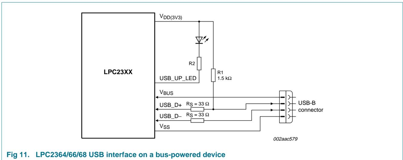
Fig 11. LPC2364/66/68 USB interface on a bus-powered device
