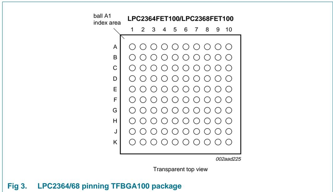
Fig 3. LPC2364/68 pinning TFBGA100 package
