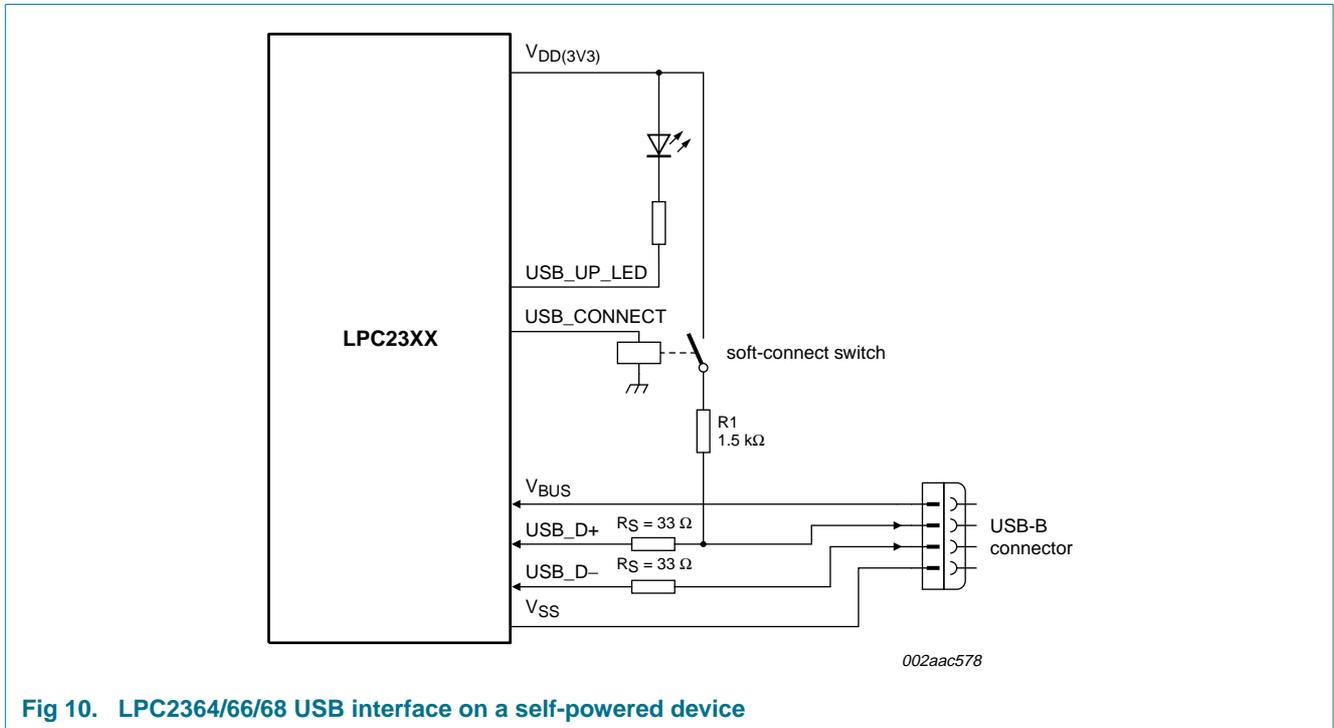
Fig 10. LPC2364/66/68 USB interface on a self-powered device
