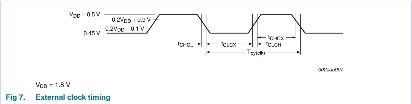
Fig 7. External clock timing
