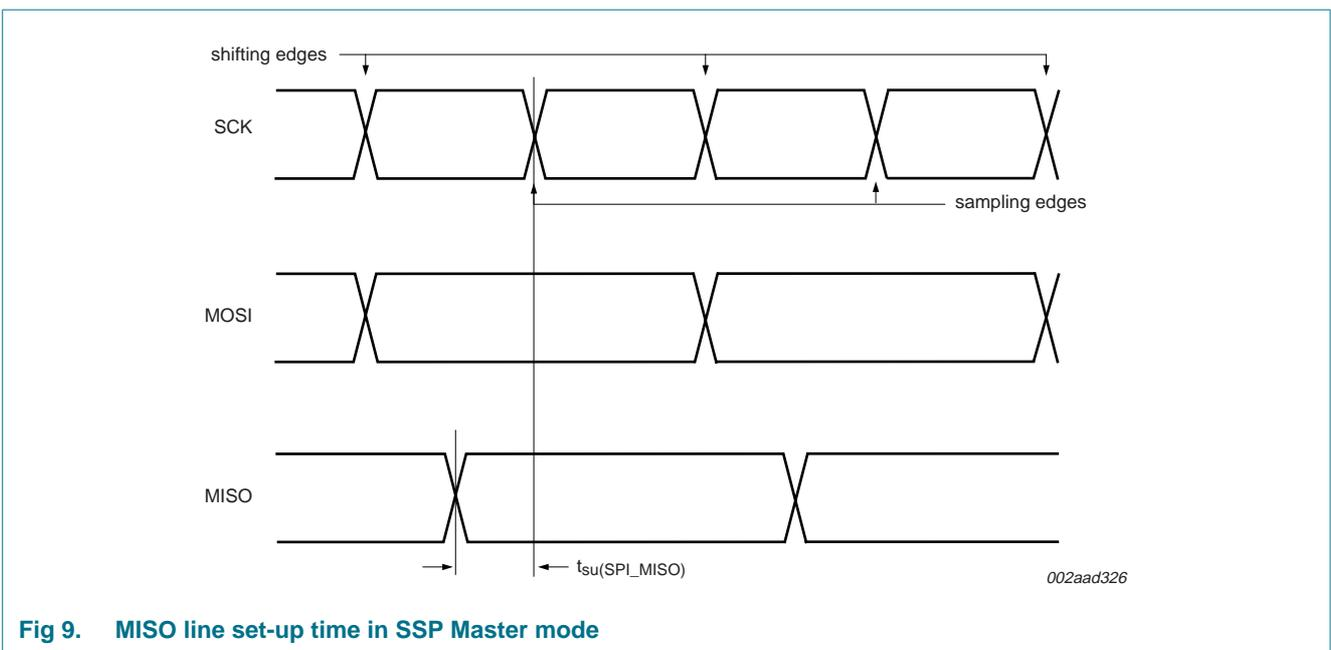
Fig 9. MISO line set-up time in SSP Master mode
