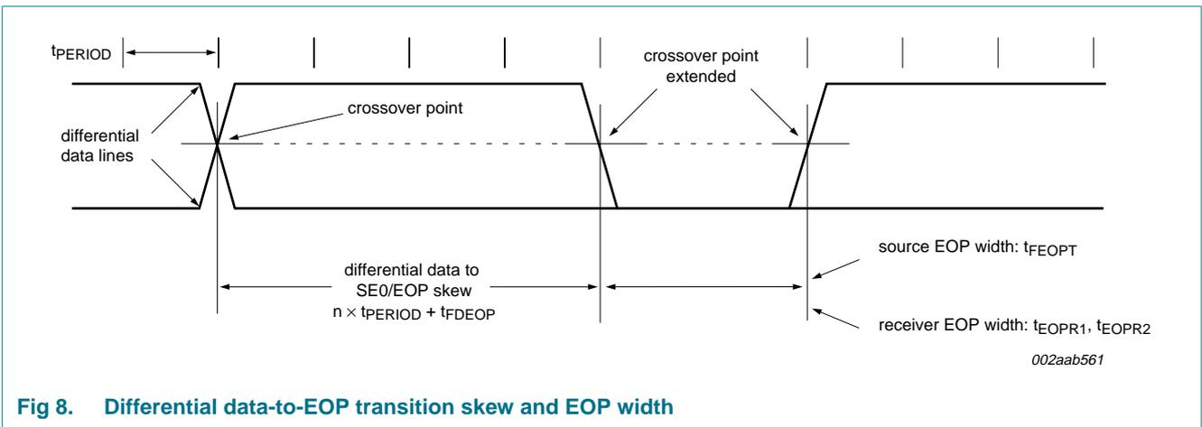
Fig 8. Differential data-to-EOP transition skew and EOP width
