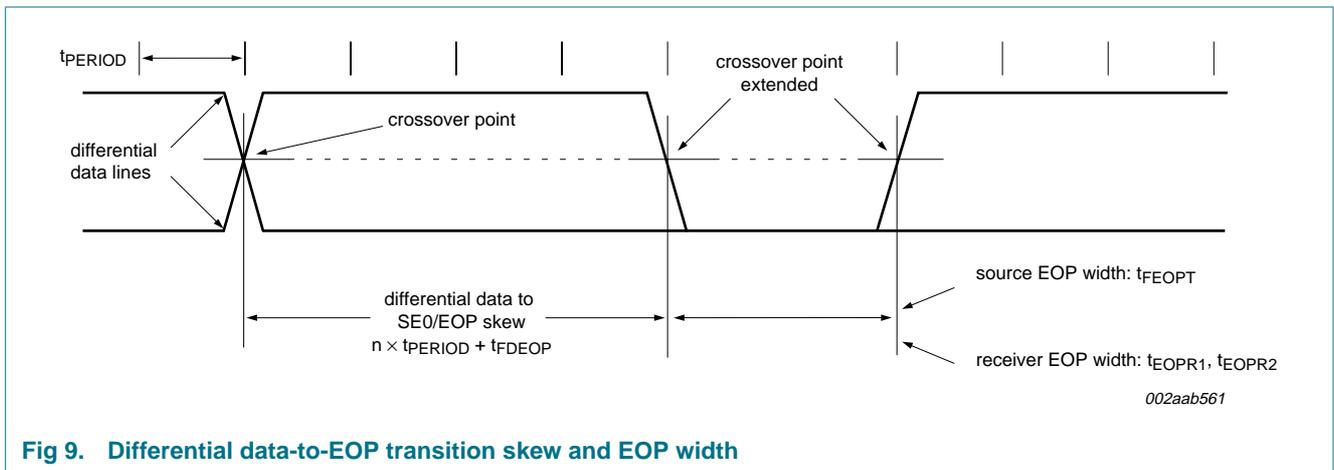
Fig 9. Differential data-to-EOP transition skew and EOP width
