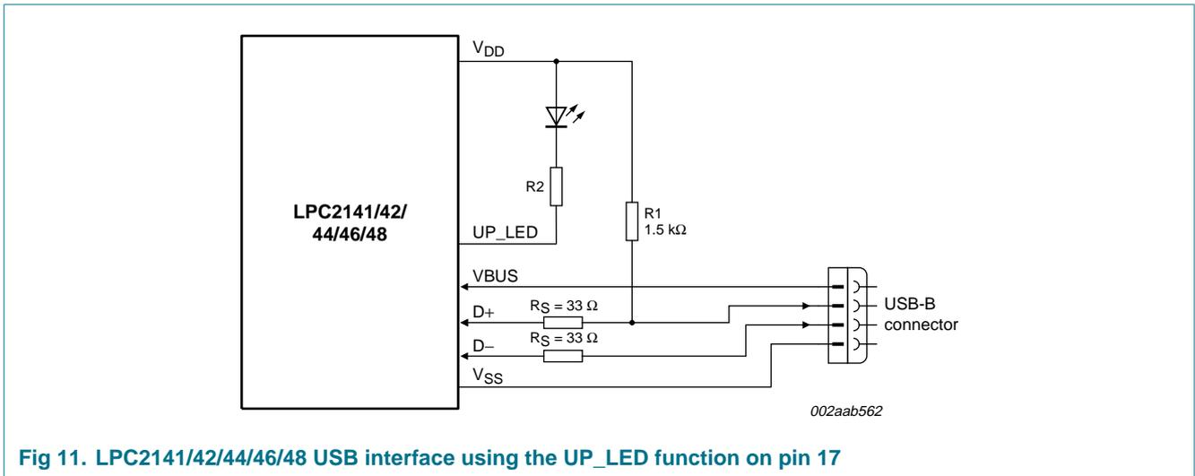
Fig 11. LPC2141/42/44/46/48 USB interface using the UP\_LED function on pin 17
