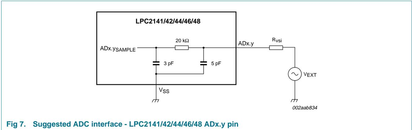
Fig 7. Suggested ADC interface - LPC2141/42/44/46/48 ADx.y pin
