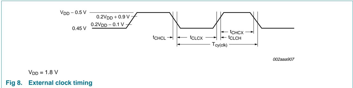
Fig 8. External clock timing
