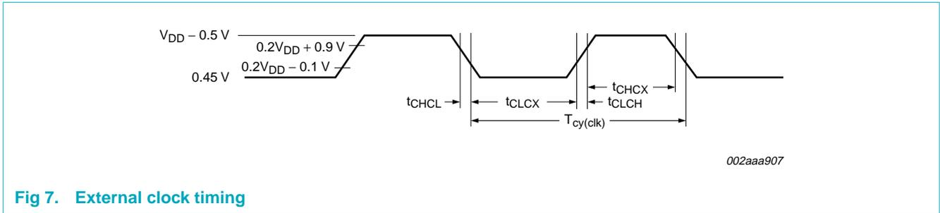
Fig 7. External clock timing
