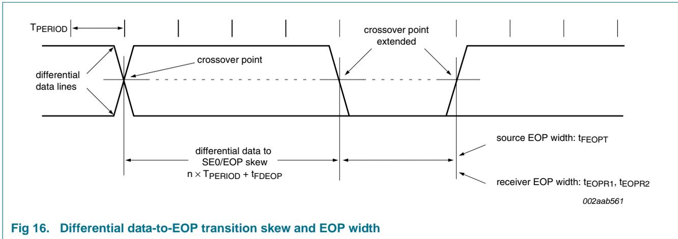
Fig 16. Differential data-to-EOP transition skew and EOP width
