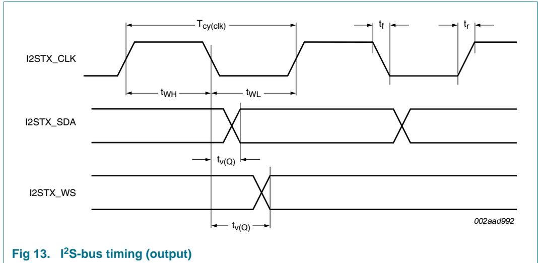
Fig 13. I<sup>2</sup>S-bus timing (output)
