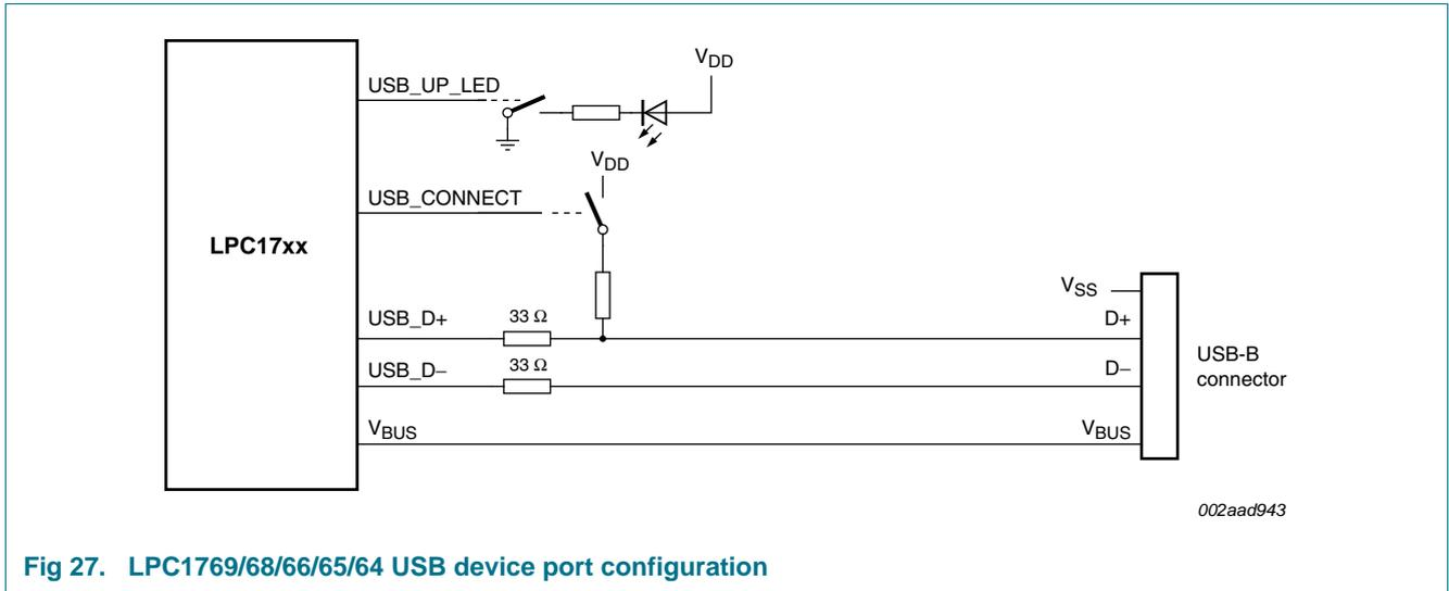
Fig 27. LPC1769/68/66/65/64 USB device port configuration
