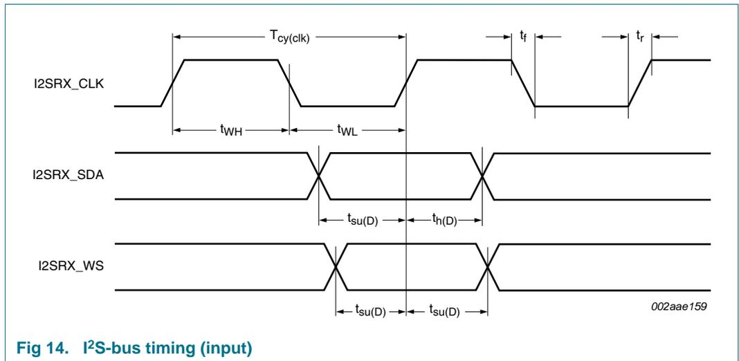
Fig 14. I<sup>2</sup>S-bus timing (input)
