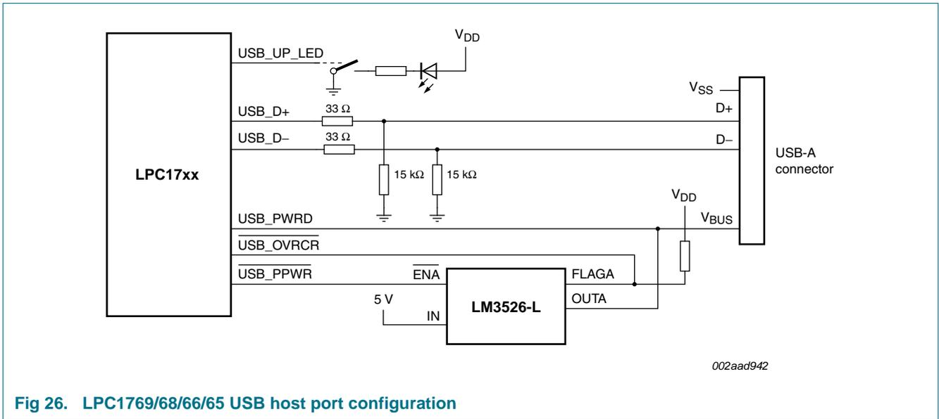
Fig 26. LPC1769/68/66/65 USB host port configuration
