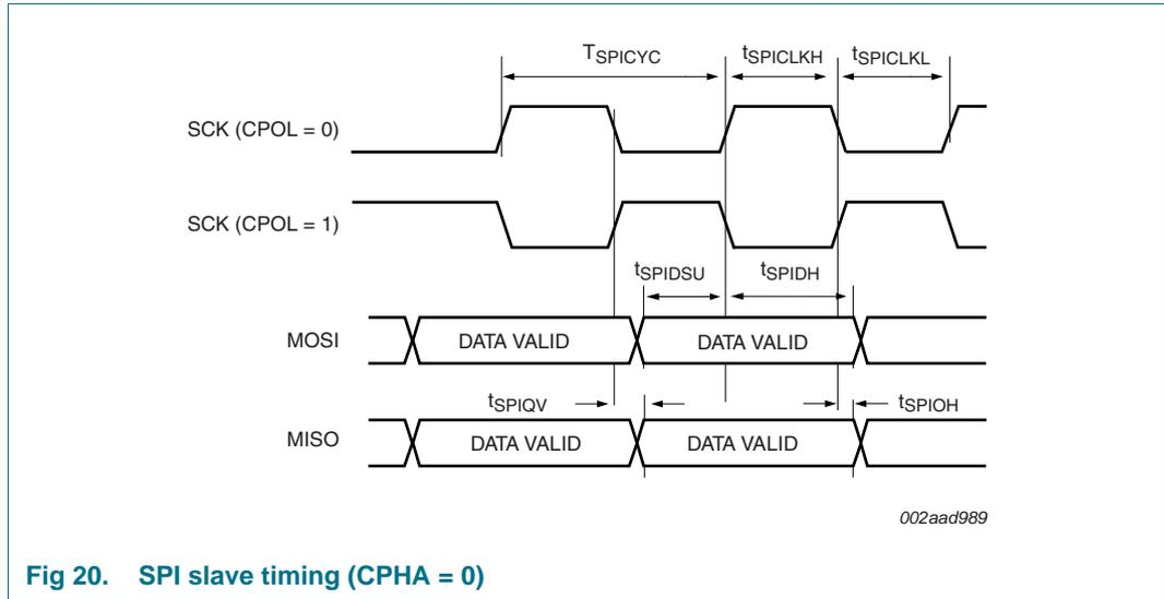
Fig 20. SPI slave timing (CPHA = 0)
