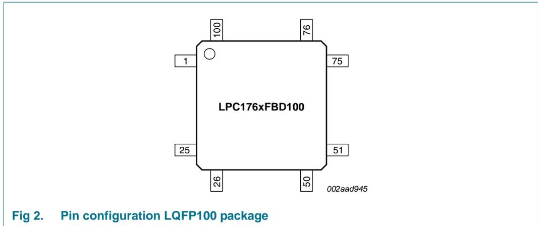
Fig 2. Pin configuration LQFP100 package
