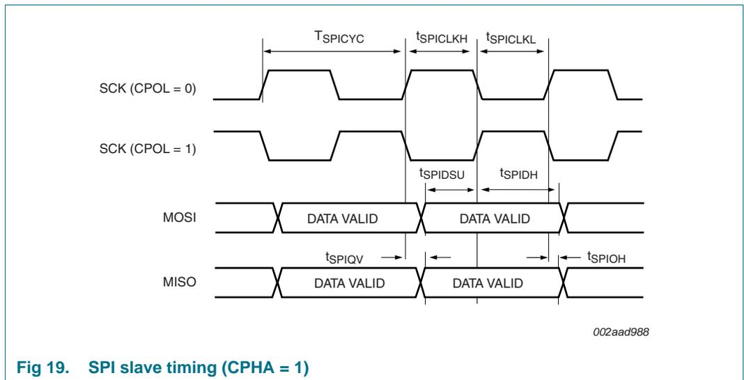
**Fig 19. SPI slave timing (CPHA = 1)**
