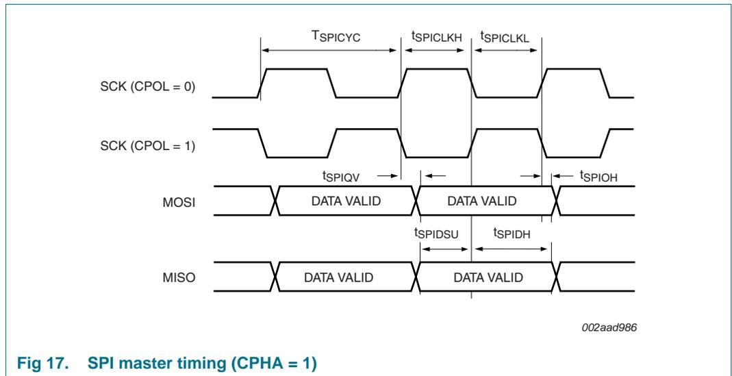
Fig 17. SPI master timing (CPHA = 1)
