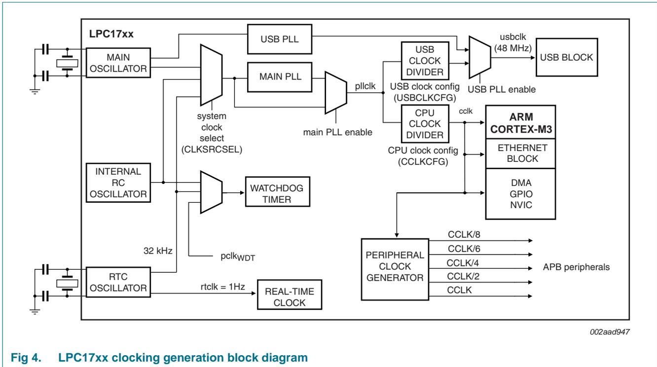
Fig 4. LPC17xx clocking generation block diagram
