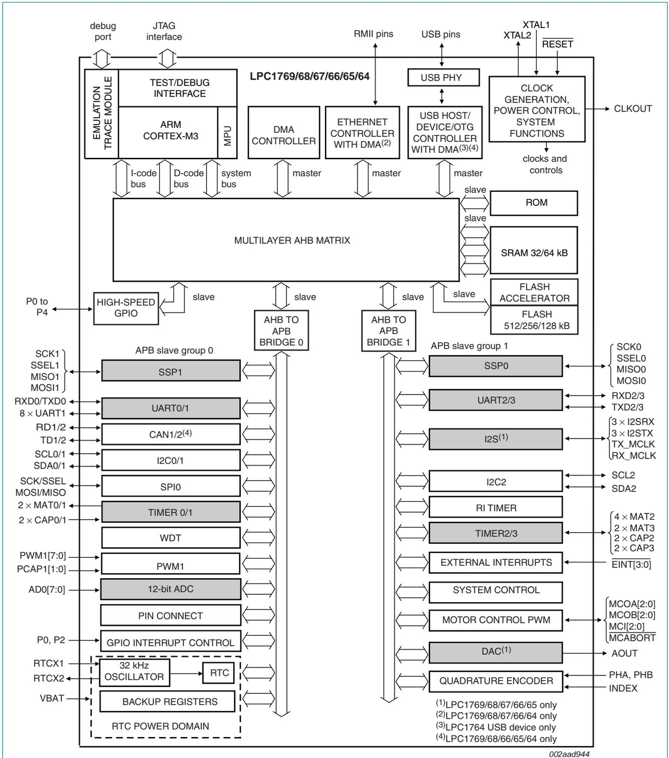
Grey-shaded blocks represent peripherals with connection to the GPDMA.
