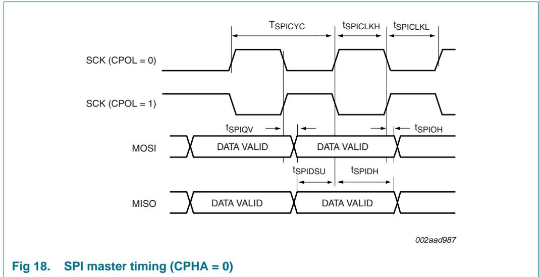
**Fig 18. SPI master timing (CPHA = 0)**
