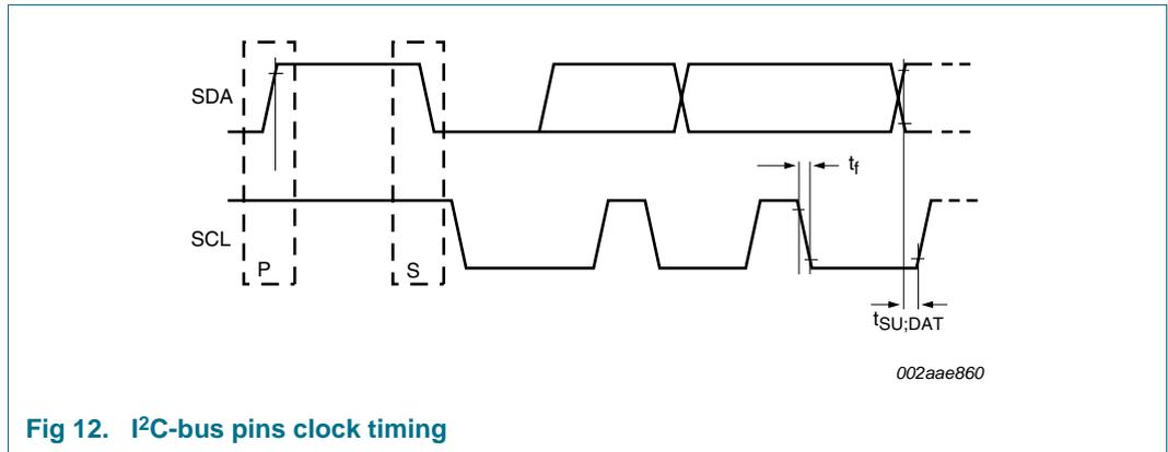
Fig 12. I<sup>2</sup>C-bus pins clock timing
