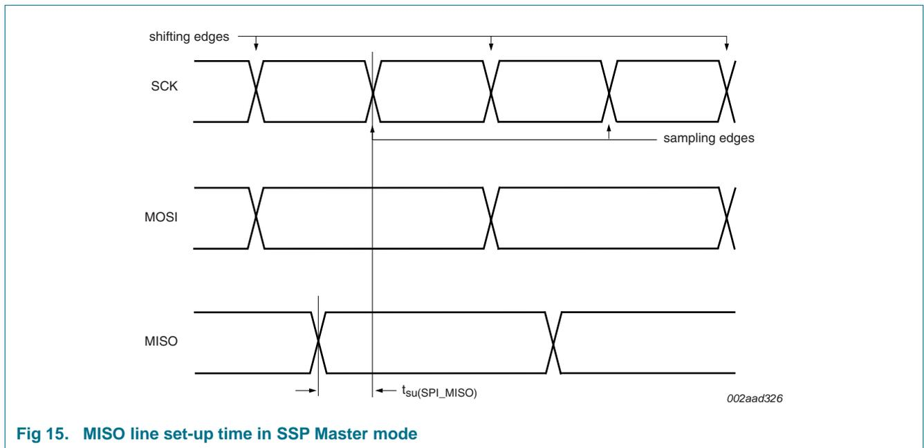
**Fig 15. MISO line set-up time in SSP Master mode**
