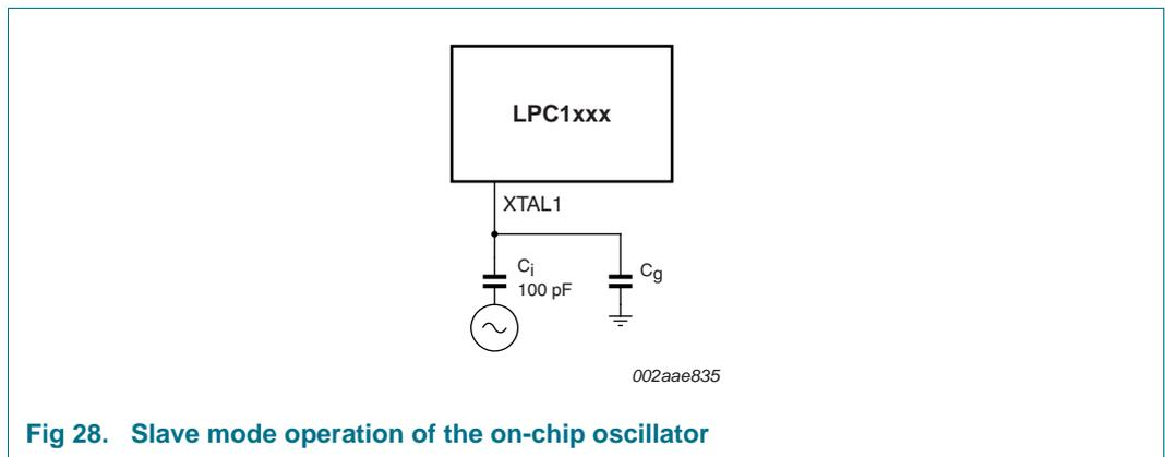
Fig 28. Slave mode operation of the on-chip oscillator
