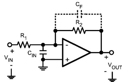
$$A_V = - \frac{V_{OUT}}{V_{IN}} = - \frac{R_2}{R_1}$$
