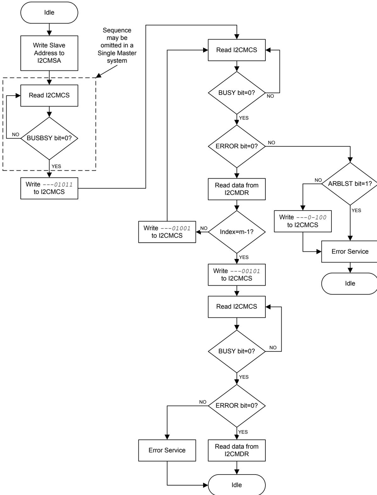
Figure 16-11. Master RECEIVE with Repeated START after TRANSMIT with Repeated START
