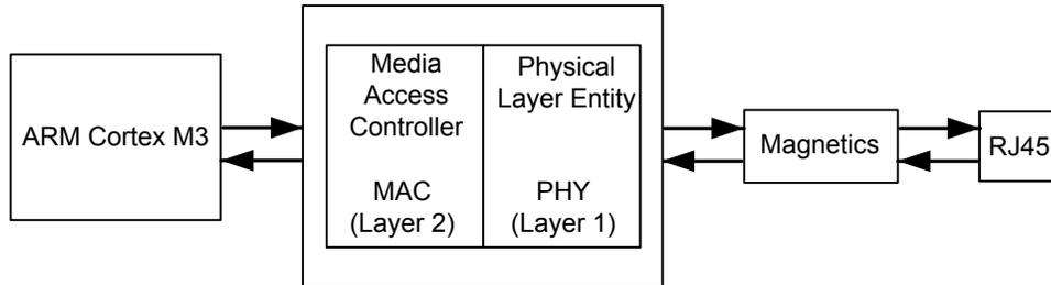
Figure 19-2 on page 781 shows more detail of the internal structure of the Ethernet Controller and how the register set relates to various functions.
