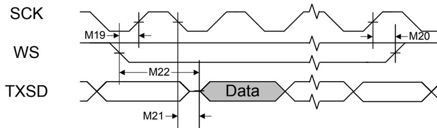
Figure 27-24. I<sup>2</sup>S Slave Mode Receive Timing
