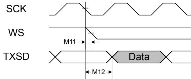
**Figure 27-22. I<sup>2</sup>S Master Mode Receive Timing**
