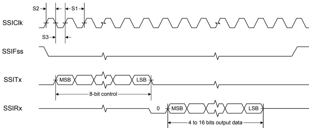
Figure 27-19. SSI Timing for SPI Frame Format (FRF=00), with SPH=1
