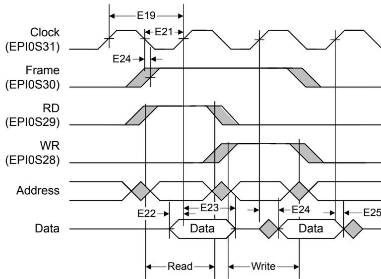
The above figure illustrates accesses where the `FRMCNT` field is 0x0, the `RD2CYC` bit is clear, and the `WR2CYC` bit is clear.
