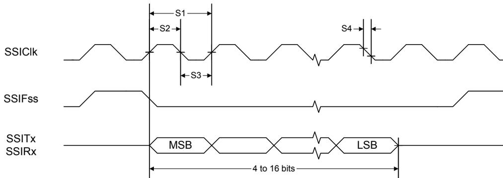
**Figure 27-18. SSI Timing for MICROWIRE Frame Format (FRF=10), Single Transfer**
