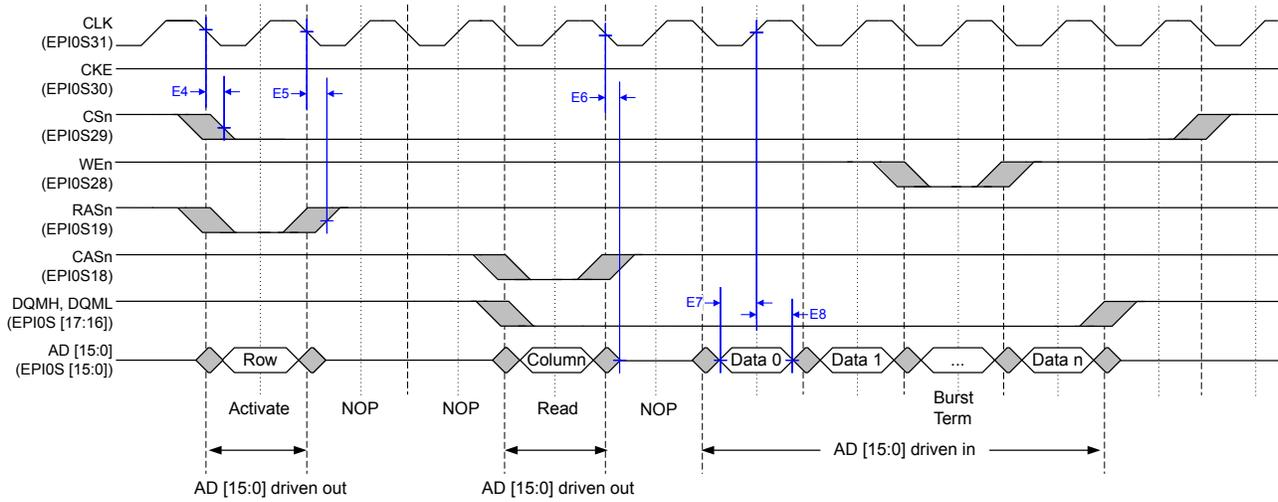
Figure 27-12. SDRAM Write Timing
