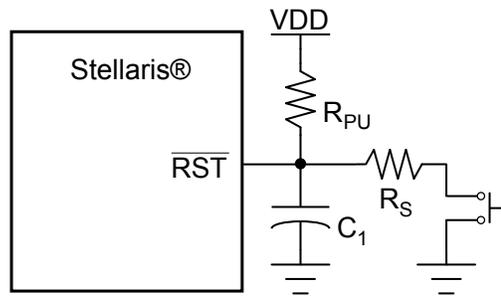
Typical  $R_{PU} = 10\text{ k}\Omega$
