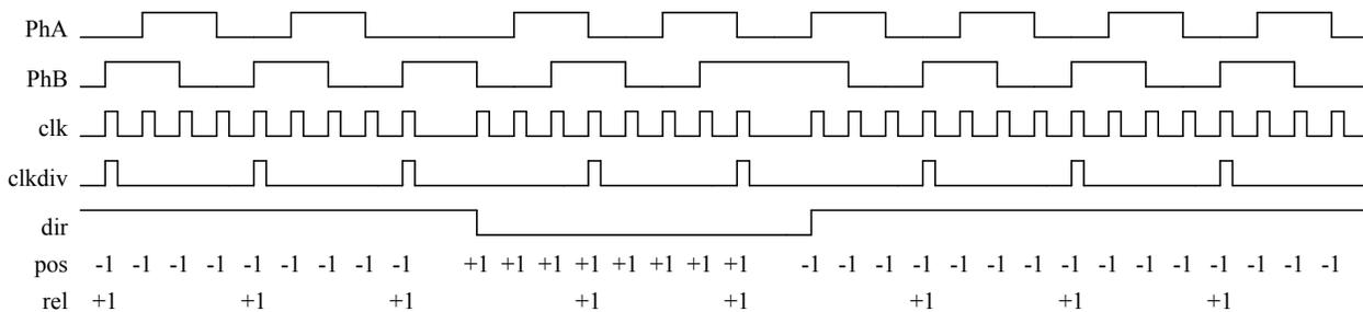
The period of the timer is configurable by specifying the load value for the timer in the **QEI Timer Load (QEILOAD)** register. When the timer reaches zero, an interrupt can be triggered, and the hardware reloads the timer with the **QEILOAD** value and continues to count down. At lower encoder speeds, a longer timer period is required to be able to capture enough edges to have a meaningful result. At higher encoder speeds, both a shorter timer period and/or the velocity predivider can be used.
