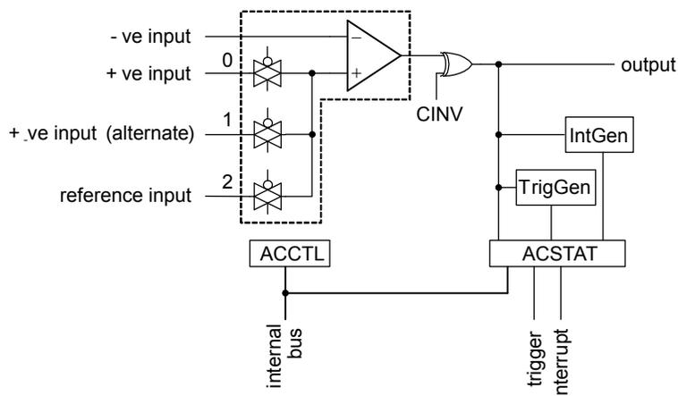
A comparator is configured through two status/control registers, **Analog Comparator Control (ACCTL)** and **Analog Comparator Status (ACSTAT)**. The internal reference is configured through one control register, **Analog Comparator Reference Voltage Control (ACREFCTL)**. Interrupt status and control are configured through three registers, **Analog Comparator Masked Interrupt**
