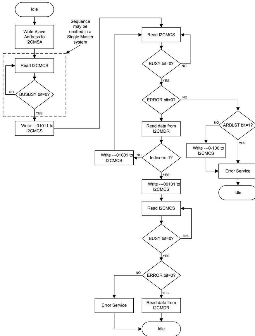
Figure 16-11. Master Burst RECEIVE after Burst SEND
