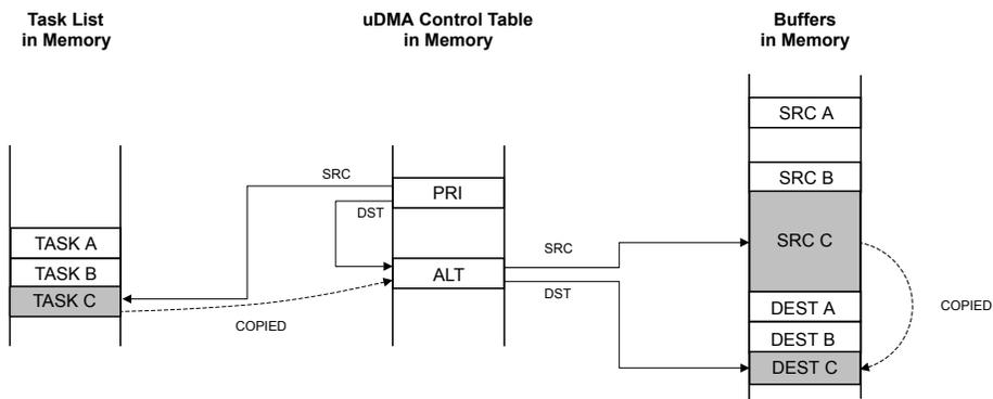
Using the channel's primary control structure, the uDMA controller copies task C configuration to the channel's alternate control structure.
