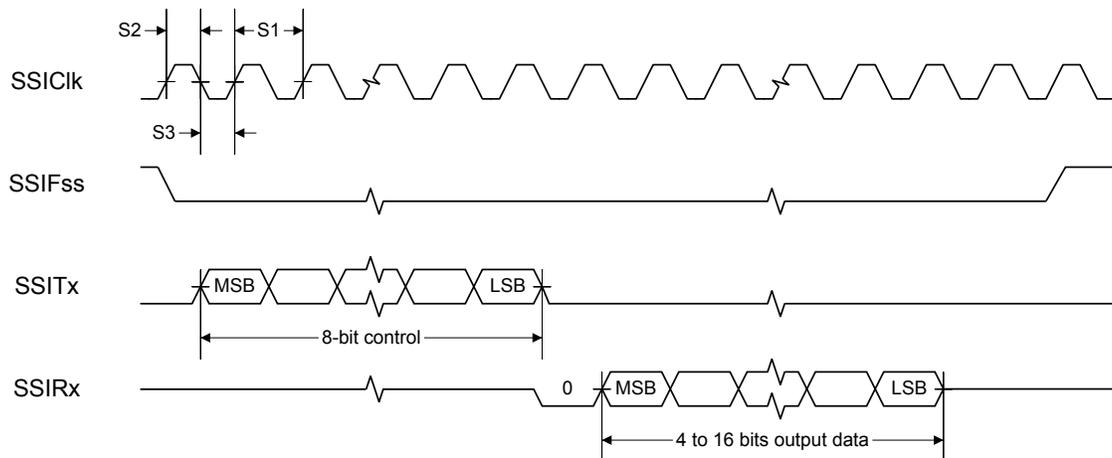
Figure 24-6. SSI Timing for SPI Frame Format (FRF=00), with SPH=1
