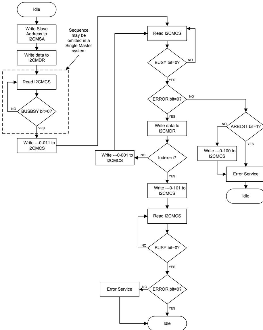
Figure 16-10. Master Burst RECEIVE
