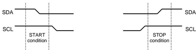
When operating in slave mode, two bits in the **I2CRIS** register indicate detection of start and stop conditions on the bus; while two bits in the **I2CSMIS** register allow start and stop conditions to be promoted to controller interrupts (when interrupts are enabled).
