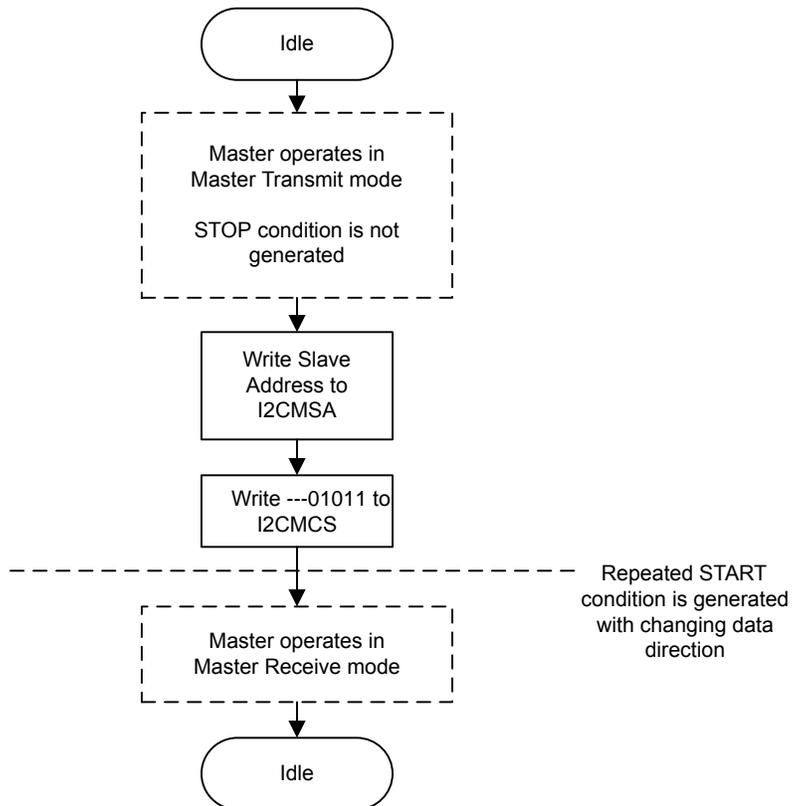
**Figure 16-12. Master Burst SEND after Burst RECEIVE**
