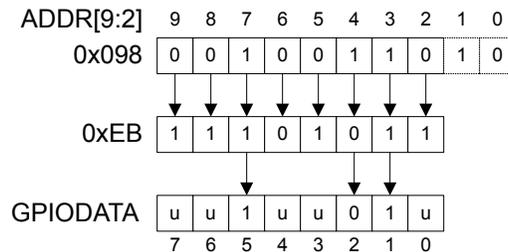
During a read, if the address bit associated with the data bit is set to 1, the value is read. If the address bit associated with the data bit is set to 0, it is read as a zero, regardless of its actual value. For example, reading address **GPIODATA + 0x0C4** yields as shown in Figure 10-4 on page 253.
