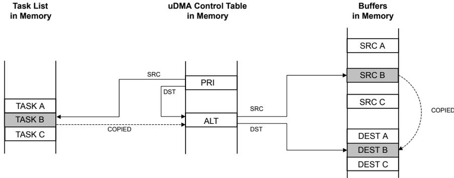
Using the channel's primary control structure, the uDMA controller copies task B configuration to the channel's alternate control structure.
