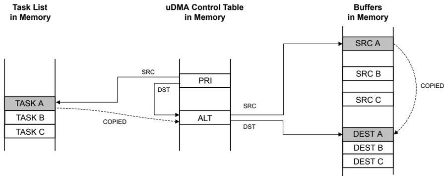
Using the channel's primary control structure, the uDMA controller copies task A configuration to the channel's alternate control structure.
