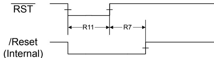
**Figure 24-10. Power-On Reset Timing**
