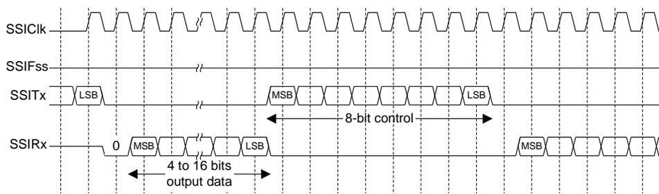
In the MICROWIRE mode, the SSI slave samples the first bit of receive data on the rising edge of SSIClk after SSIFss has gone Low. Masters that drive a free-running SSIClk must ensure that the SSIFss signal has sufficient setup and hold margins with respect to the rising edge of SSIClk.
