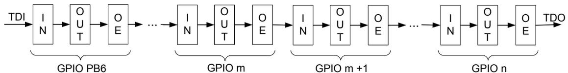
For detailed information on the order of the input, output, and output enable bits for each of the GPIO ports, please refer to the Stellaris® Family Boundary Scan Description Language (BSDL) files, downloadable from [www.luminarymicro.com](http://www.luminarymicro.com).
