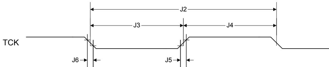
Figure 24-8. JTAG Test Access Port (TAP) Timing
