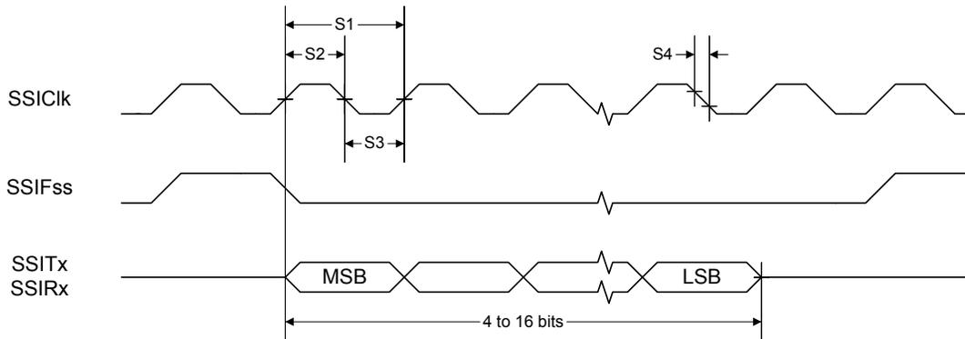
Figure 24-5. SSI Timing for MICROWIRE Frame Format (FRF=10), Single Transfer
