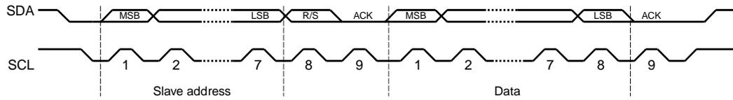
The first seven bits of the first byte make up the slave address (see Figure 16-5 on page 470). The eighth bit determines the direction of the message. A zero in the R/S position of the first byte means that the master will write (send) data to the selected slave, and a one in this position means that the master will receive data from the slave.
