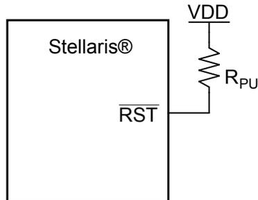
$R_{\text{PU}} = 0$  to 100 k $\Omega$
