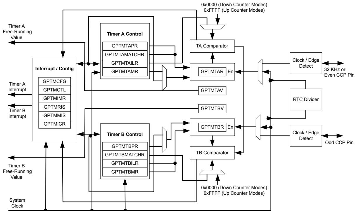
**Note:** In Figure 11-1 on page 339, the specific Capture Compare PWM (CCP) pins available depend on the Stellaris® device. See Table 11-1 on page 339 for the available CCP pins and their timer assignments
