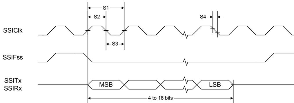
Figure 21-14. SSI Timing for MICROWIRE Frame Format (FRF=10), Single Transfer
