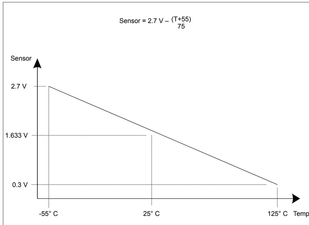
The temperature reading from the temperature sensor can also be given as a function of the ADC value. The following formula calculates temperature (in °C) based on the ADC reading:
