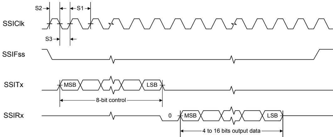
Figure 21-15. SSI Timing for SPI Frame Format (FRF=00), with SPH=1
