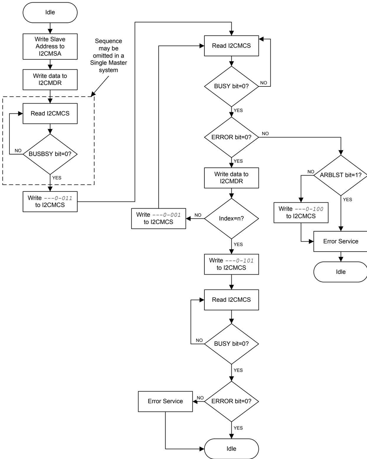
Figure 16-10. Master RECEIVE with Repeated START
