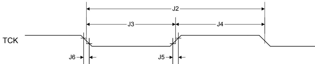
Figure 21-3. JTAG Test Access Port (TAP) Timing
