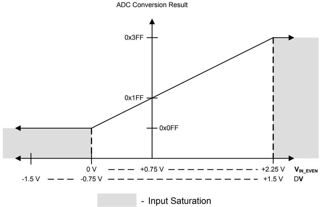
Figure 13-6. Differential Sampling Range,  $V_{IN\_ODD} = 2.25\text{ V}$
