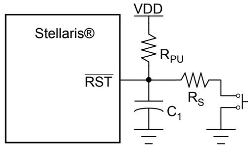
Typical  $R_{PU} = 10 \text{ k}\Omega$
