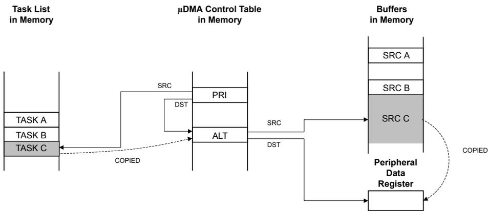
Using the channel's primary control structure, the  $\mu$ DMA controller copies task C configuration to the channel's alternate control structure.
