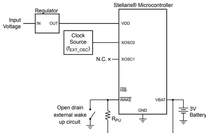
**Note:** R<sub>PU</sub> = Pull-up resistor is 1 MΩ
