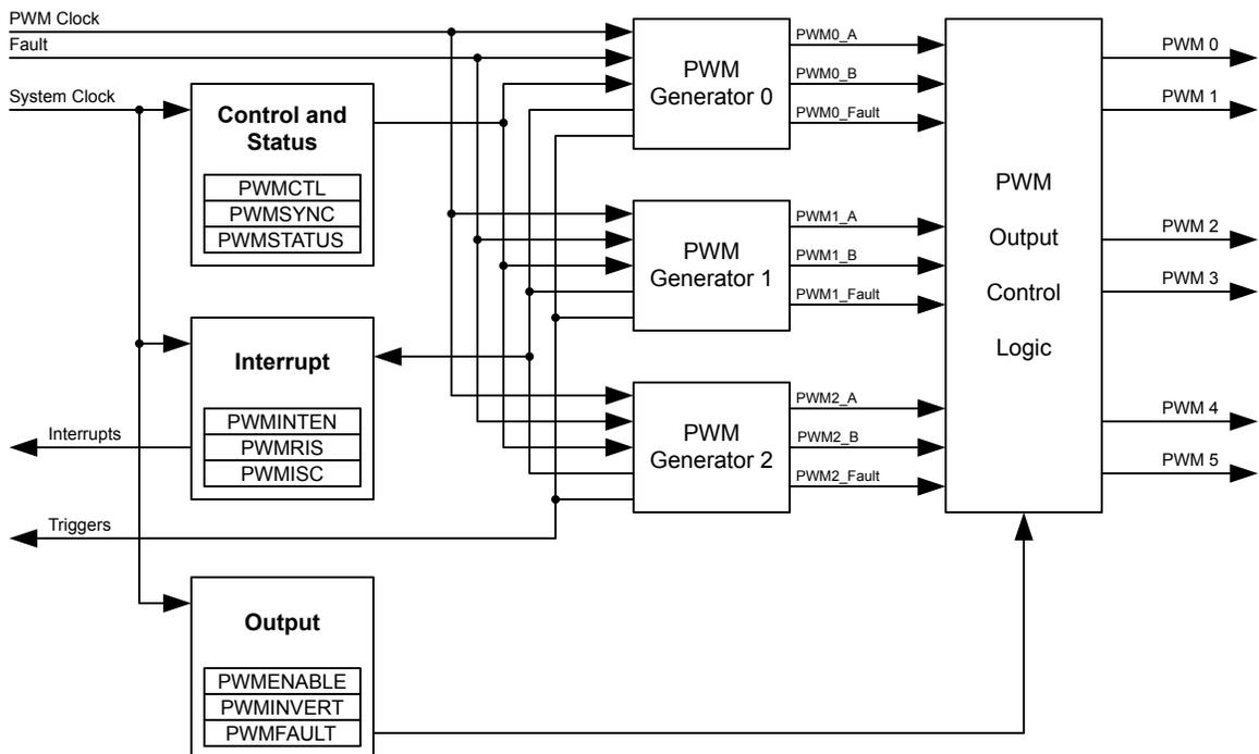
Figure 17-2. PWM Module Block Diagram
