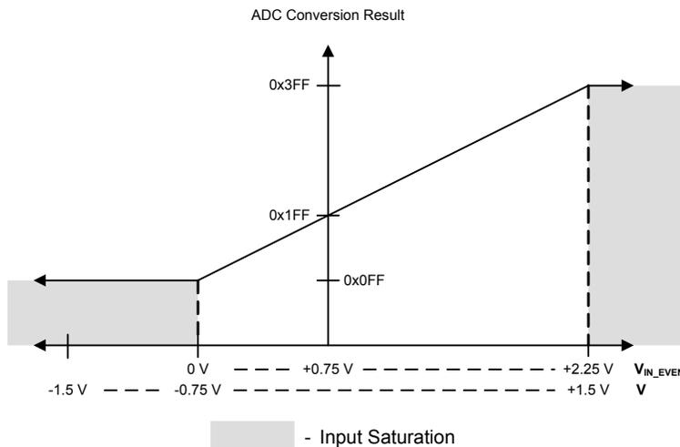
Figure 12-4. Differential Sampling Range,  $V_{IN\_ODD} = 2.25\text{ V}$
