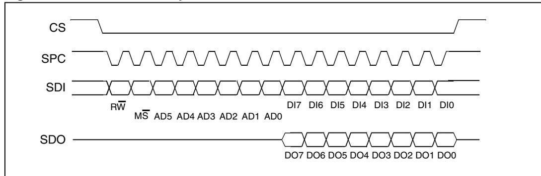
**CS** is the serial port enable and is controlled by the SPI master. It goes low at the start of the transmission and goes back high at the end. **SPC** is the serial port clock and is controlled by the SPI master. It is stopped high when **CS** is high (no transmission). **SDI** and **SDO** are, respectively, the serial port data input and output. These lines are driven at the falling edge of **SPC** and should be captured at the rising edge of **SPC**.
