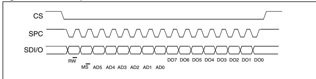
The SPI read command is performed with 16 clock pulses:
