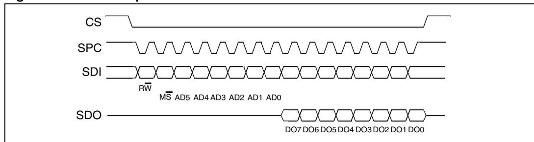
The SPI read command is performed with 16 clock pulses. A multiple byte read command is performed by adding blocks of 8 clock pulses to the previous one.
