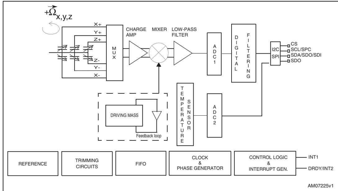
The vibration of the structure is maintained by drive circuitry in a feedback loop. The sensing signal is filtered and appears as a digital signal at the output.
