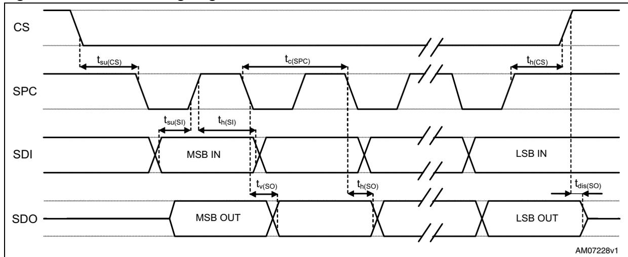
b. Measurement points are done at 0.2·Vdd\_IO and 0.8·Vdd\_IO, for both input and output ports.
