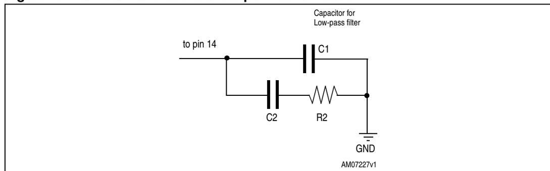
a. Pin 14 PLLFLT maximum voltage level is equal to Vdd.
