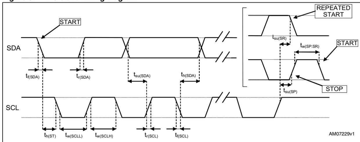
c. Measurement points are done at 0.2·Vdd\_IO and 0.8·Vdd\_IO, for both ports.
