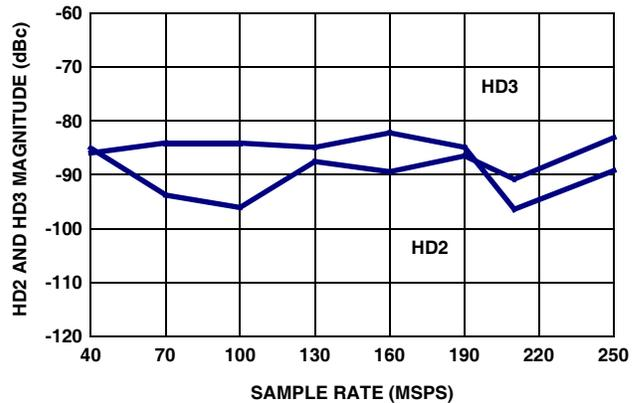
FIGURE 9. HD2 AND HD3 vs f<sub>SAMPLE</sub>
