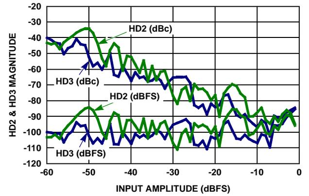
FIGURE 7. HD2 AND HD3 vs A<sub>IN</sub>
