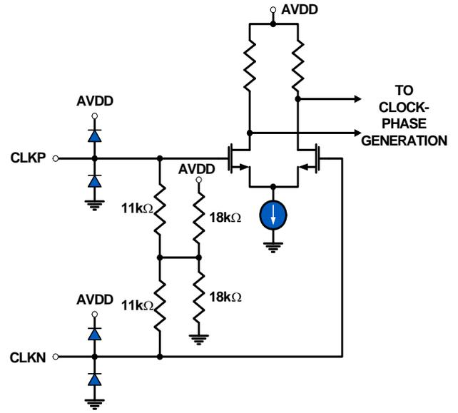
FIGURE 43. CLOCK INPUTS
