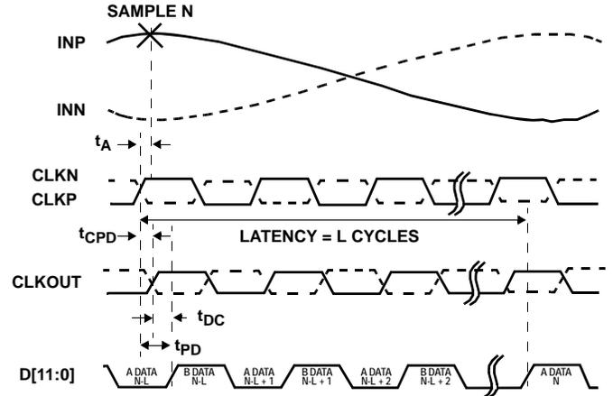
FIGURE 2. CMOS TIMING DIAGRAM—DDR (“Digital Outputs” on page 17)
