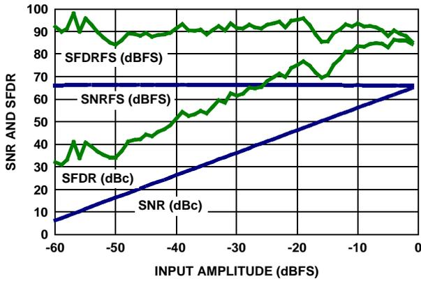
FIGURE 6. SNR AND SFDR vs A<sub>IN</sub>
