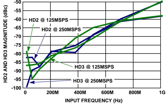
FIGURE 5. HD2 AND HD3 vs f<sub>IN</sub>
