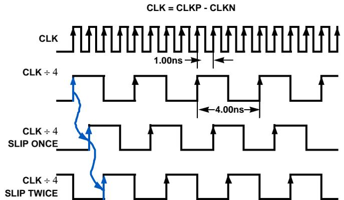
FIGURE 40. PHASE SLIP: CLK ÷ 4 MODE, f<sub>CLK</sub> = 1000MHZ
