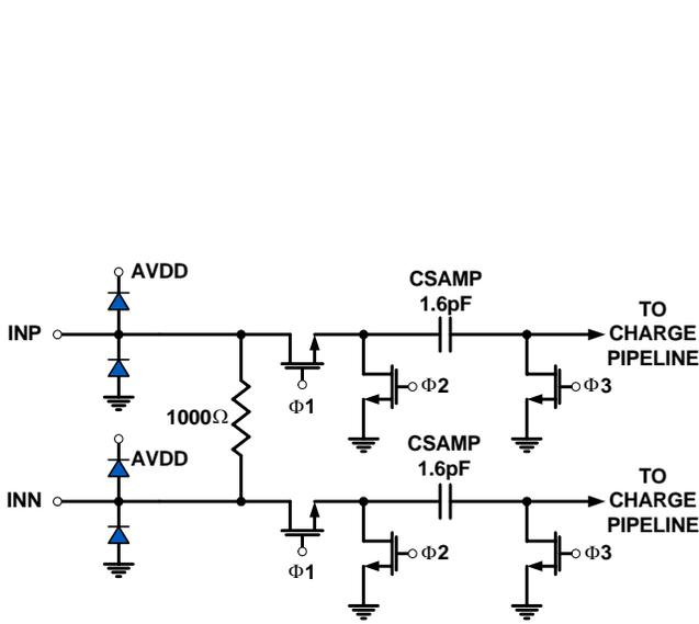
FIGURE 42. ANALOG INPUTS
