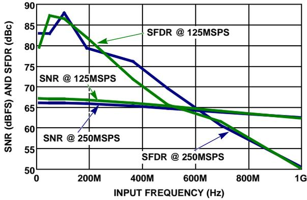
FIGURE 4. SNR AND SFDR vs f<sub>IN</sub>
