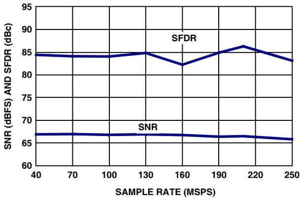
FIGURE 8. SNR AND SFDR vs f<sub>SAMPLE</sub>
