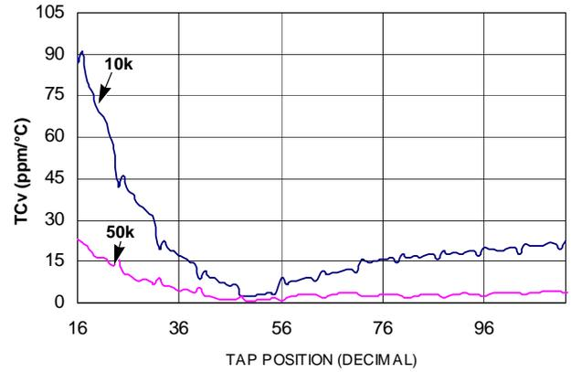
FIGURE 8. TC FOR VOLTAGE DIVIDER MODE IN ppm
