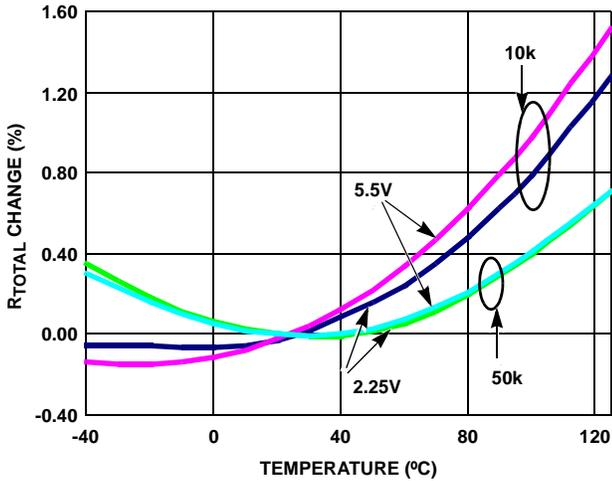
FIGURE 9. END TO END  $R_{TOTAL}$  % CHANGE vs TEMPERATURE
