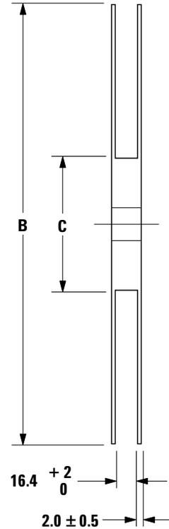
Figure 6. Tape and Reel Dimensions
