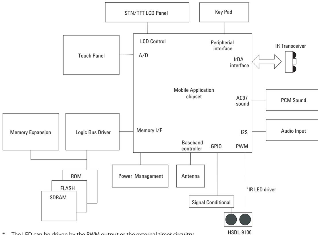
\* The LED can be driven by the PWM output or the external timer circuitry.
