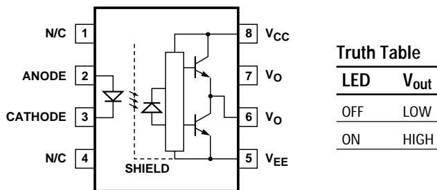
A 0.1  $\mu$ F bypass capacitor must be connected between pins 5 and 8.
