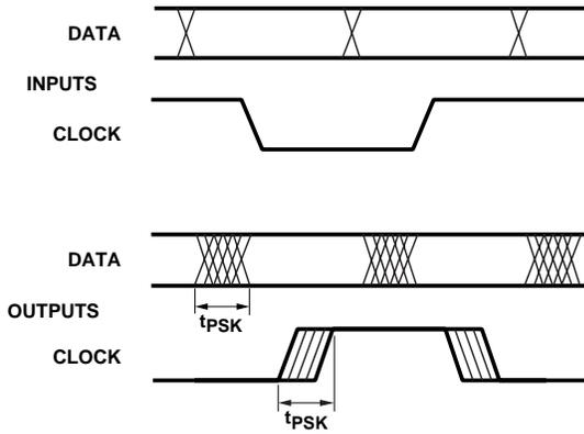
Figure 16. Parallel Data Transmission Example.
