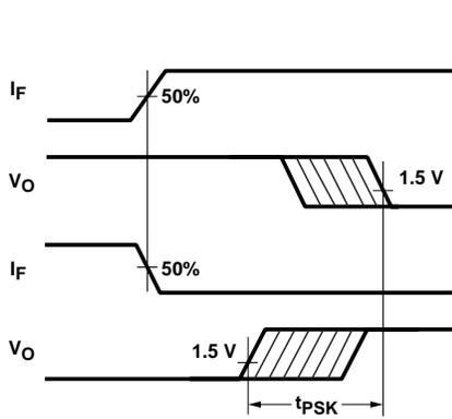
Figure 15. Illustration of Propagation Delay Skew -  $t_{PSK}$ .
