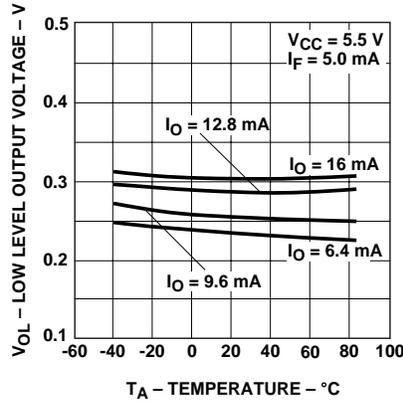
**Figure 2. Low Level Output Voltage vs. Temperature.**
