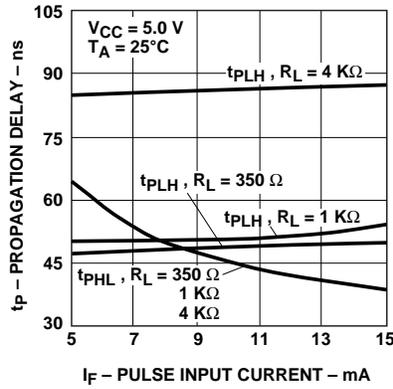
**Figure 8. Propagation Delay vs. Pulse Input Current.**
