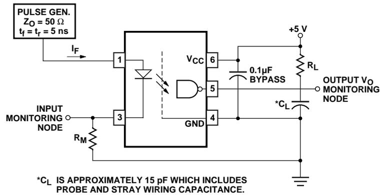
**Figure 5. Test Circuit for  $t_{PHL}$  and  $t_{PLH}$ .**
