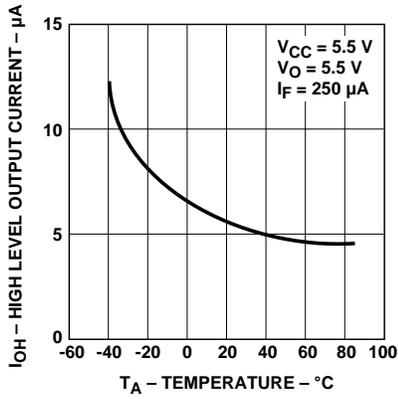
**Figure 1. High Level Output Current vs. Temperature.**
