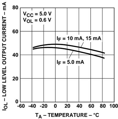
**Figure 6. Low Level Output Current vs. Temperature.**
