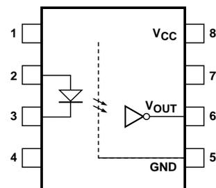
The connection of a 0.1  $\mu$ F bypass capacitor between  $V_{CC}$  and GND is recommended.
