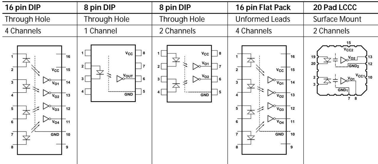
Note: All DIP and flat pack devices have common  $V_{CC}$  and ground. LCCC (leadless ceramic chip carrier) package has isolated channels with separate  $V_{CC}$  and ground connections.
