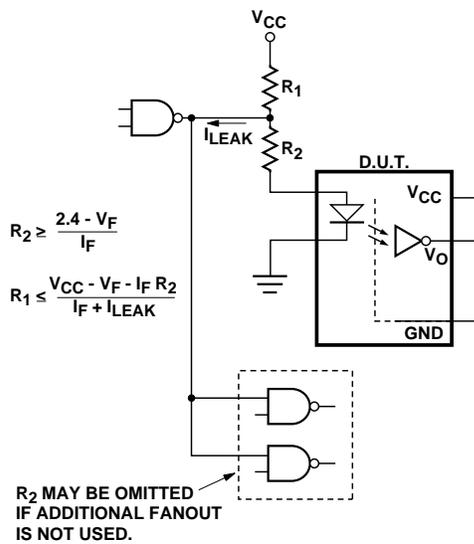
Figure 10. Recommended Drive Circuitry Using TTL Open-Collector Logic.
