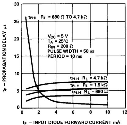
Figure 7. Propagation Delay vs. Input Diode Forward Current.
