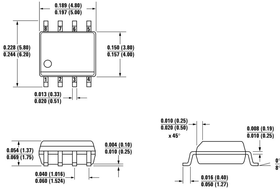
DIMENSIONS: INCHES (MILLIMETERS) **MIN**
