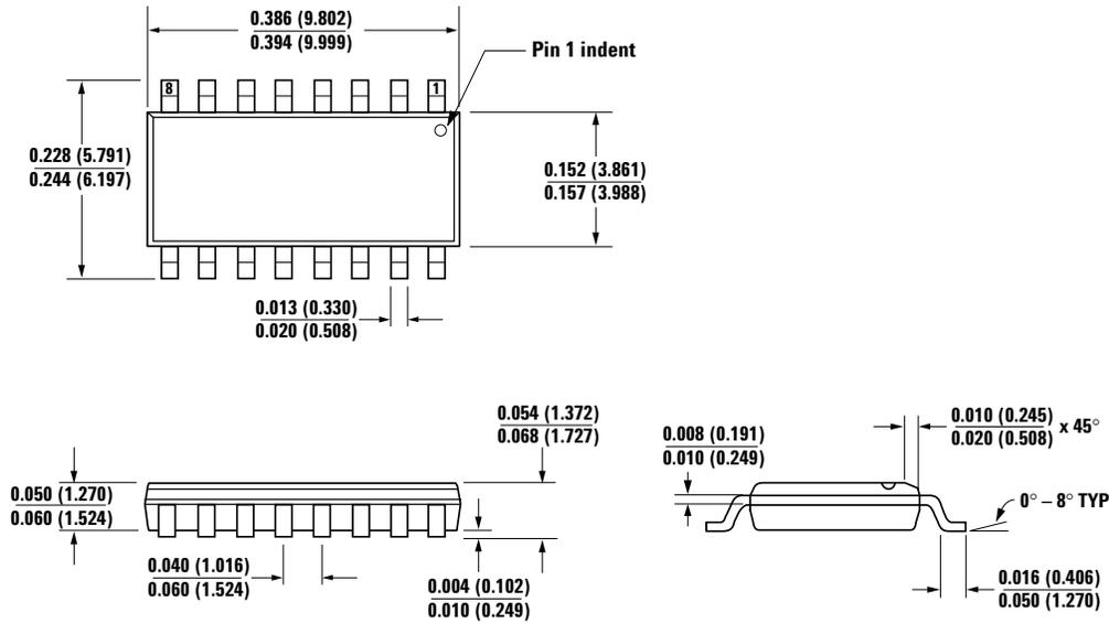
DIMENSIONS: INCHES (MILLIMETERS)  $\frac{\text{MIN}}{\text{MAX}}$
