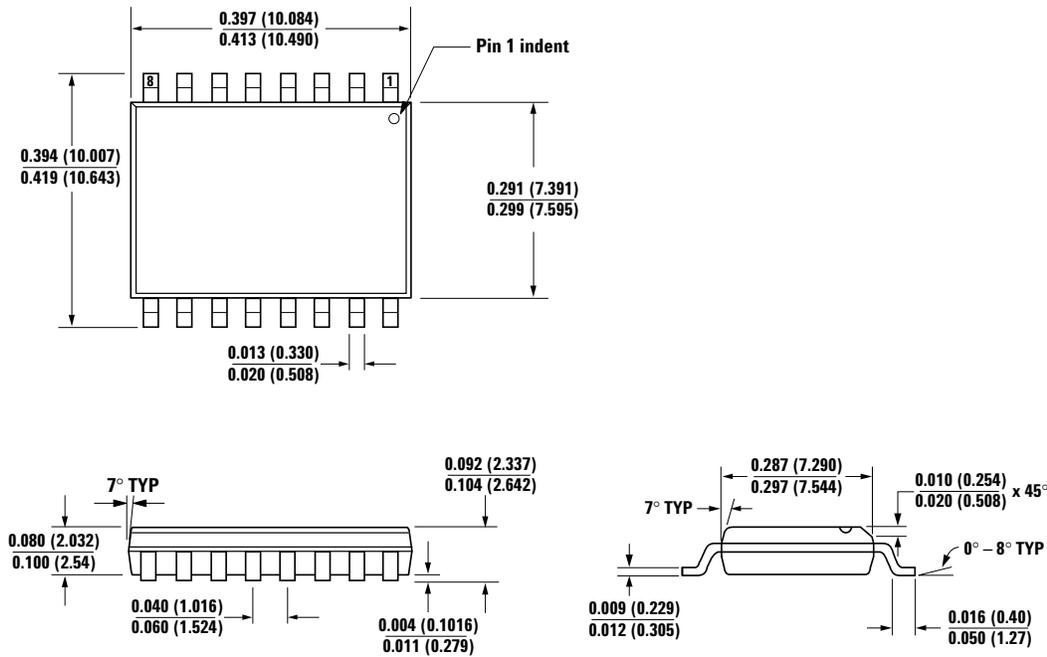
DIMENSIONS: INCHES (MILLIMETERS) **MIN**
