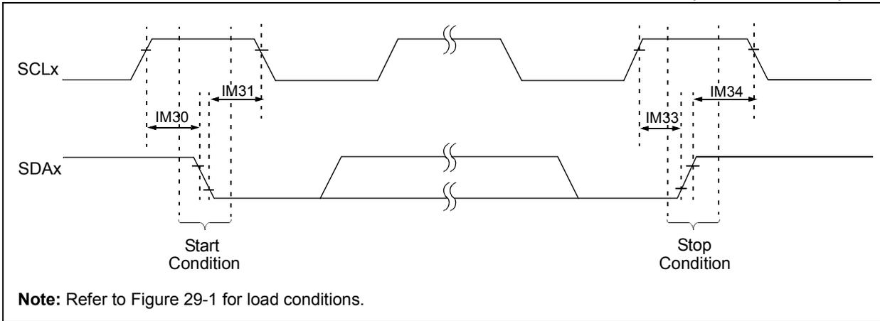
FIGURE 29-14: I2Cx BUS DATA TIMING CHARACTERISTICS (MASTER MODE)
