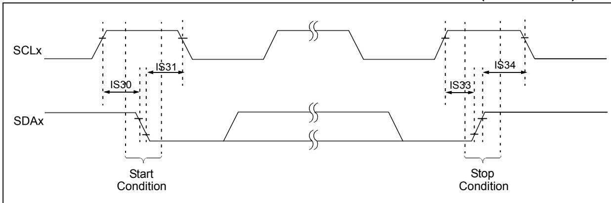
**FIGURE 29-16: I2Cx BUS DATA TIMING CHARACTERISTICS (SLAVE MODE)**
