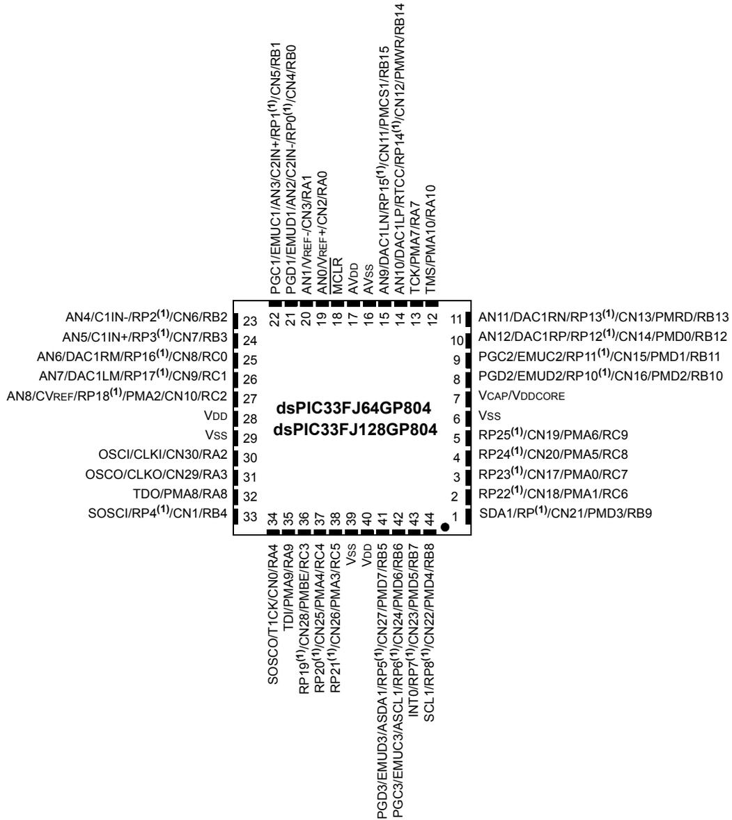
Note 1: The RPx pins can be used by any remappable peripheral. See the table “dsPIC33FJ32GP302/304, dsPIC33FJ64GPX02/X04, and dsPIC33FJ128GPX02/X04 Controller Families” in this section for the list of available peripherals.
