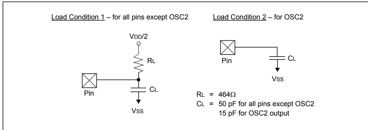
**TABLE 29-15: CAPACITIVE LOADING REQUIREMENTS ON OUTPUT PINS**
