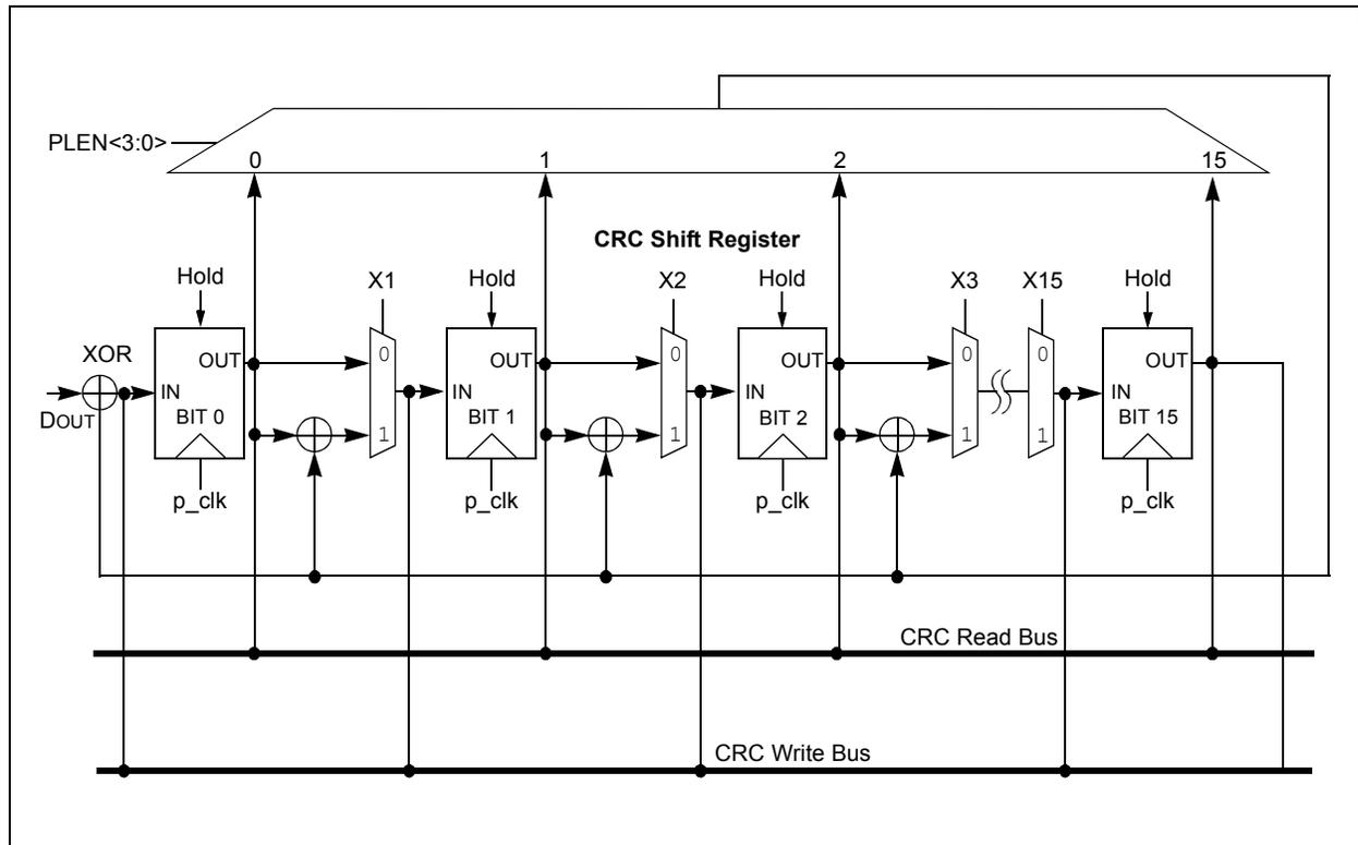
FIGURE 24-2: CRC GENERATOR RECONFIGURED FOR  $x^{16} + x^{12} + x^5 + 1$
