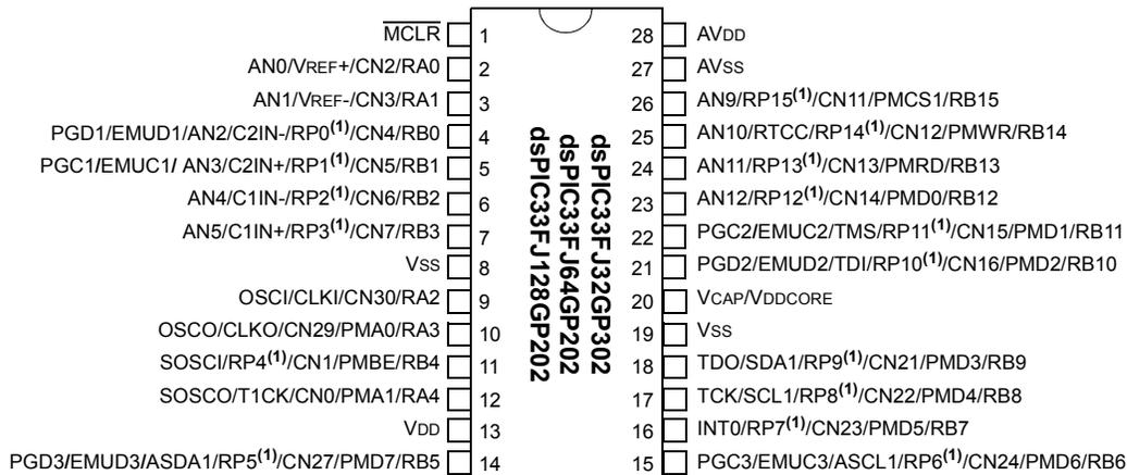
**Note 1:** The RPx pins can be used by any remappable peripheral. See the table “dsPIC33FJ32GP302/304, dsPIC33FJ64GPX02/X04, and dsPIC33FJ128GPX02/X04 Controller Families” in this section for the list of available peripherals.
