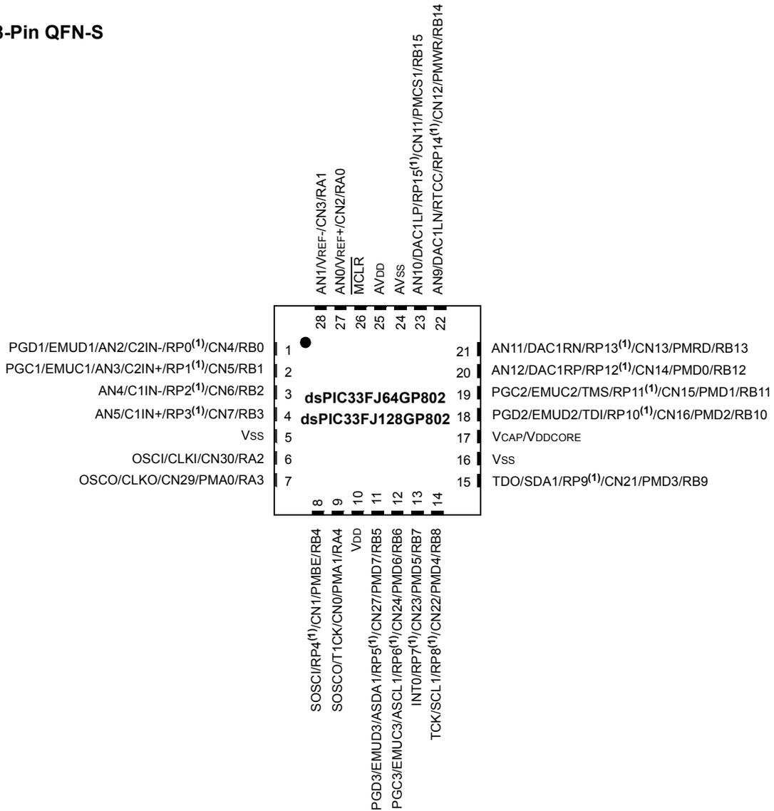
**Note 1:** The RPx pins can be used by any remappable peripheral. See the table “dsPIC33FJ32GP302/304, dsPIC33FJ64GPX02/X04, and dsPIC33FJ128GPX02/X04 Controller Families” in this section for the list of available peripherals.
