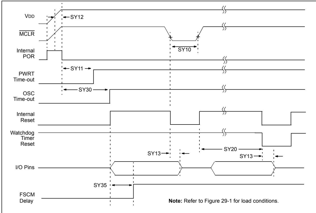
**TABLE 29-21: RESET, WATCHDOG TIMER, OSCILLATOR START-UP TIMER, POWER-UP TIMER TIMING REQUIREMENTS**
