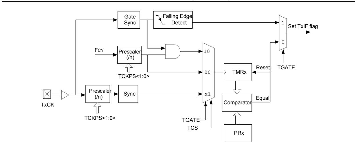
**FIGURE 12-2: TYPE C TIMER BLOCK DIAGRAM (x = 3 or 5)**
