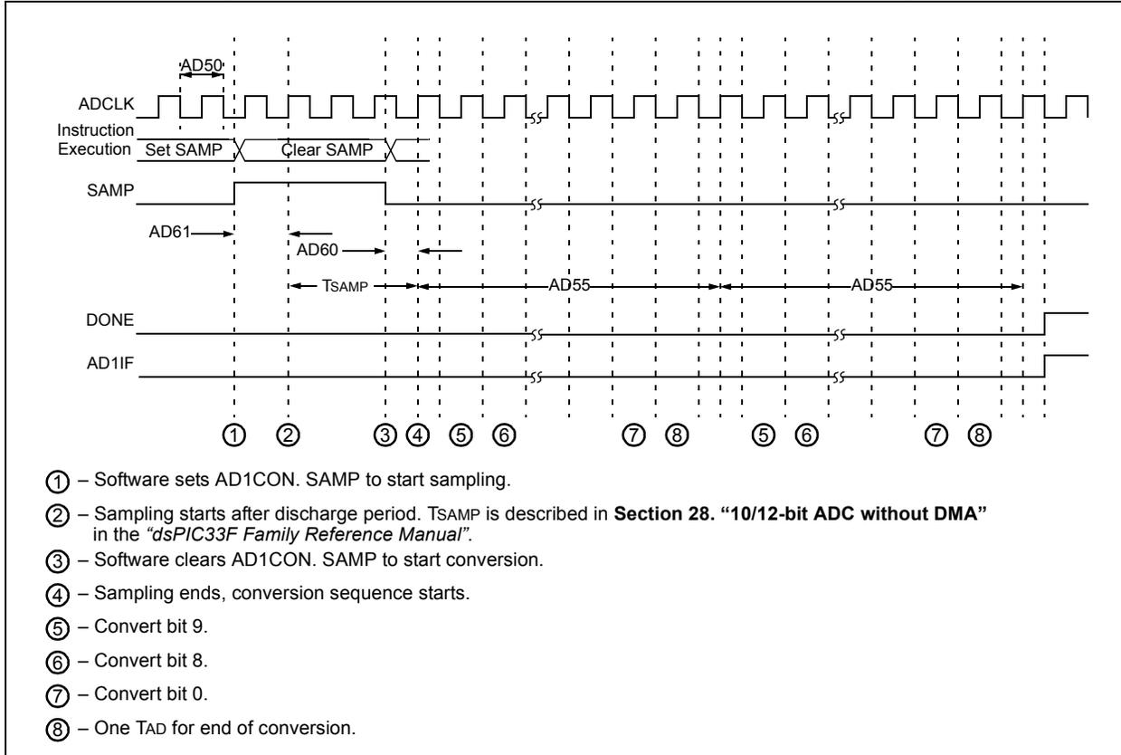
**FIGURE 29-22: ADC CONVERSION (10-BIT MODE) TIMING CHARACTERISTICS (CHPS<1:0> = 01, SIMSAM = 0, ASAM = 1, SSRC<2:0> = 111, SAMC<4:0> = 00001)**
