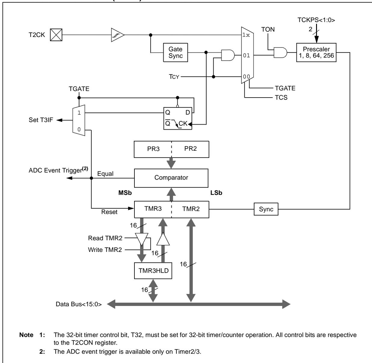
**FIGURE 11-2: TIMER2 (16-BIT) BLOCK DIAGRAM**
