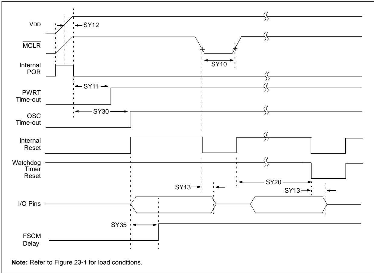
**TABLE 23-21: RESET, WATCHDOG TIMER, OSCILLATOR START-UP TIMER, POWER-UP TIMER TIMING REQUIREMENTS**
