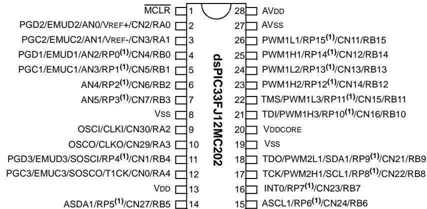
**Note 1:** The RPN pins can be used by any remappable peripheral. See Table 1 for the list of available peripherals.
