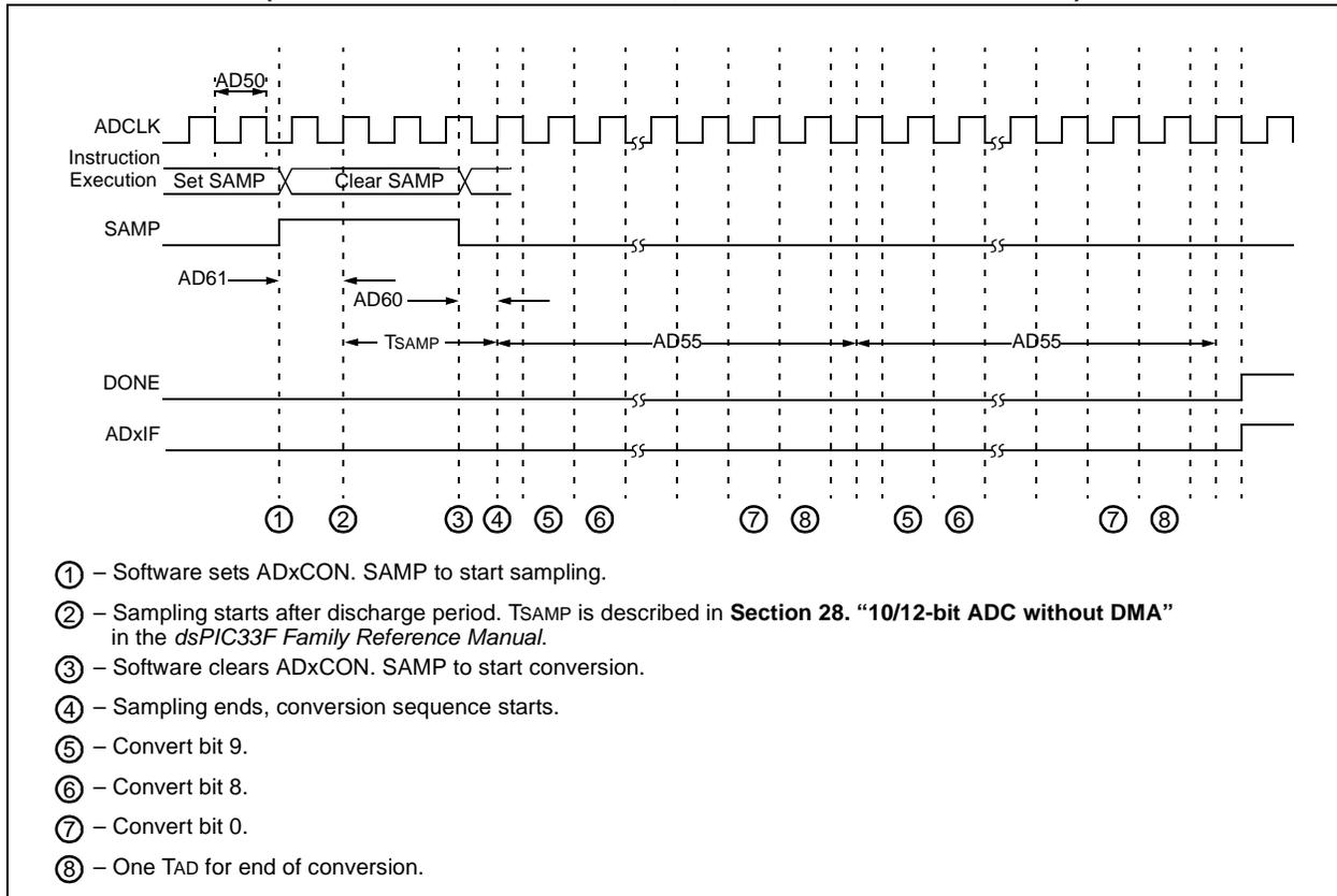
**FIGURE 23-24: ADC CONVERSION (10-BIT MODE) TIMING CHARACTERISTICS (CHPS<1:0> = 01, SIMSAM = 0, ASAM = 1, SSRC<2:0> = 111, SAMC<4:0> = 00001)**
