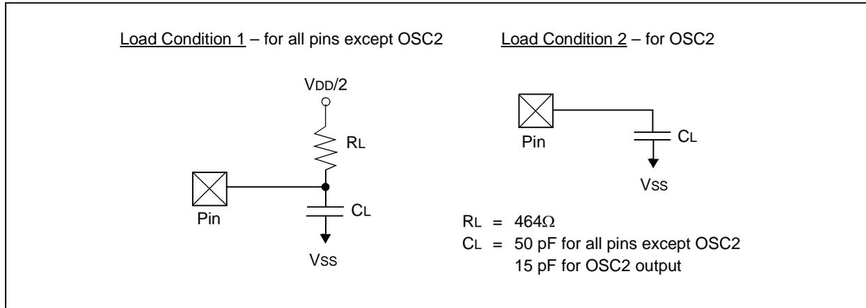
**TABLE 23-15: CAPACITIVE LOADING REQUIREMENTS ON OUTPUT PINS**
