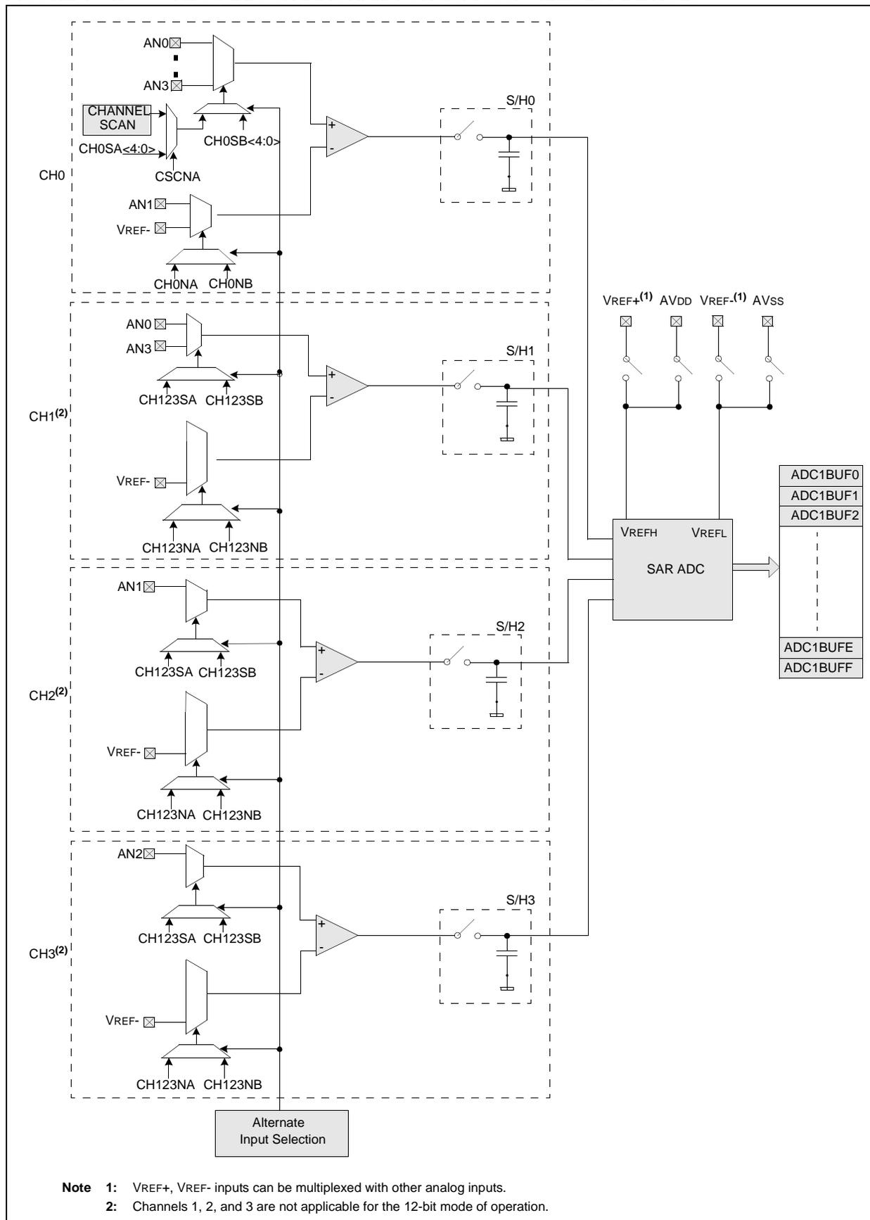
**FIGURE 19-2: ADC1 BLOCK DIAGRAM FOR dsPIC33FJ12MC202 DEVICES**
