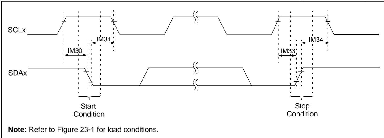
**FIGURE 23-19: I2Cx BUS DATA TIMING CHARACTERISTICS (MASTER MODE)**
