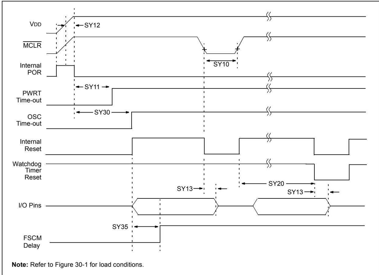
**TABLE 30-21: RESET, WATCHDOG TIMER, OSCILLATOR START-UP TIMER, POWER-UP TIMER TIMING REQUIREMENTS**
