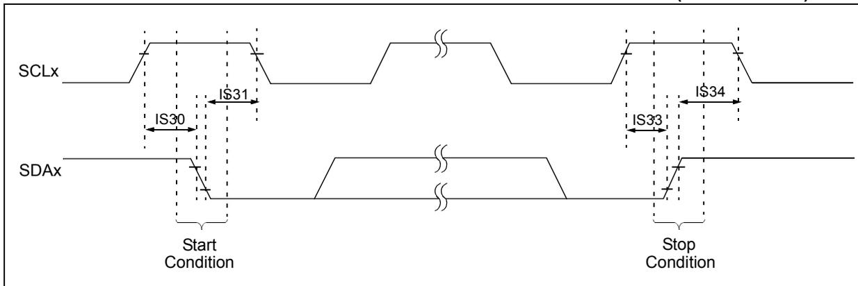
**FIGURE 30-21: I2Cx BUS DATA TIMING CHARACTERISTICS (SLAVE MODE)**
