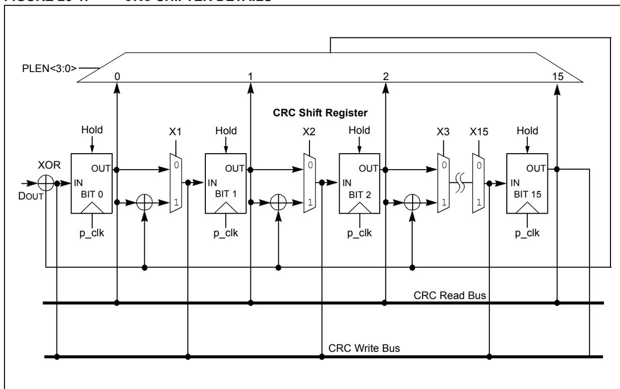
FIGURE 25-2: CRC GENERATOR RECONFIGURED FOR  $x^{16} + x^{12} + x^5 + 1$
