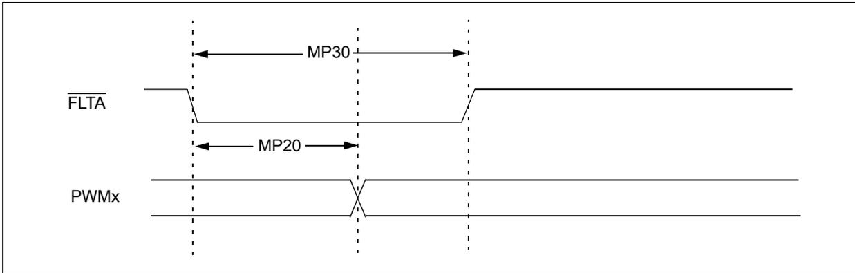
FIGURE 30-11: MOTOR CONTROL PWM MODULE TIMING CHARACTERISTICS
