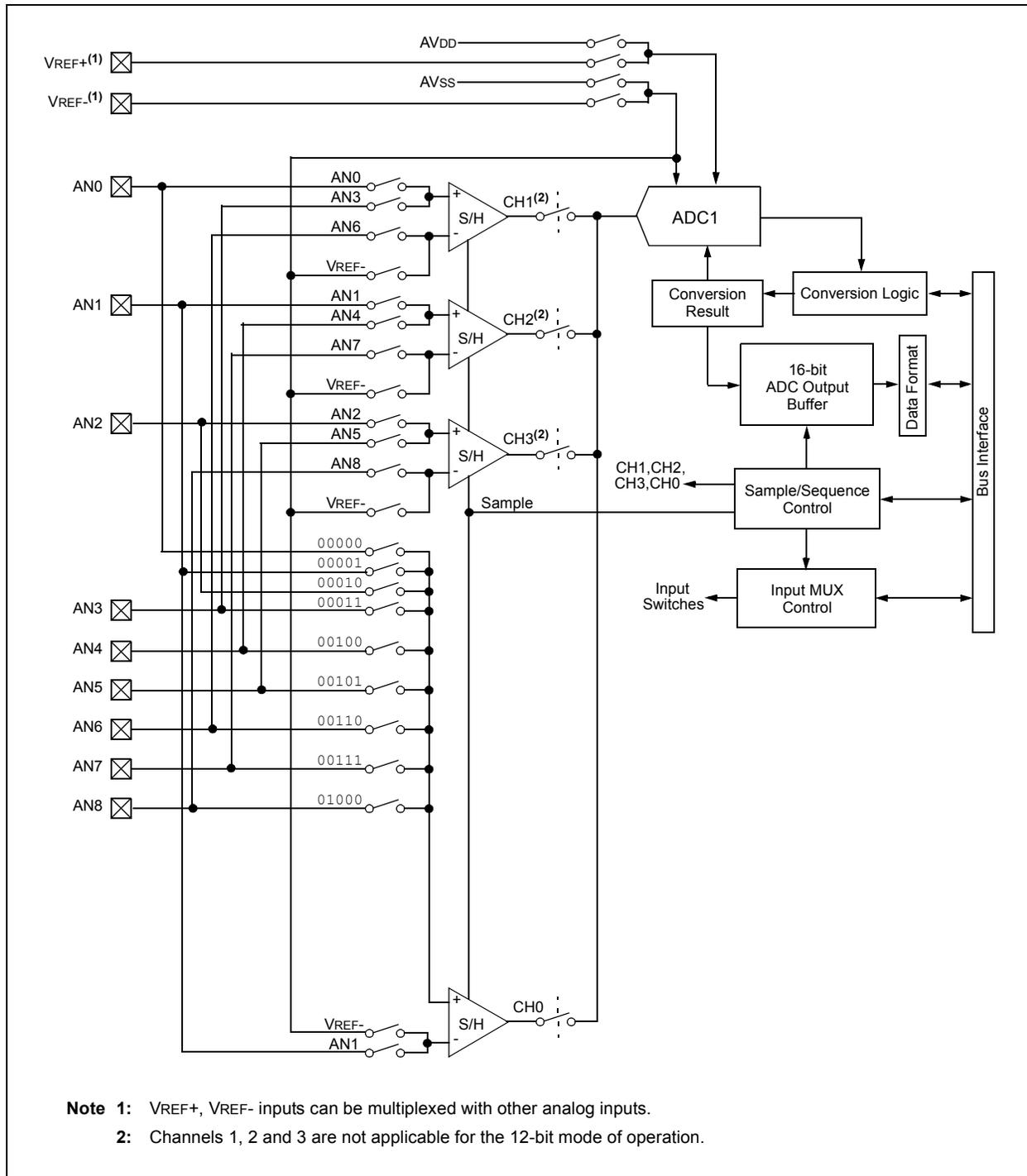
**FIGURE 21-2: ADC1 MODULE BLOCK DIAGRAM FOR dsPIC33FJ32MC302, dsPIC33FJ64MC202/802, AND dsPIC33FJ128MC202/802 DEVICES**
