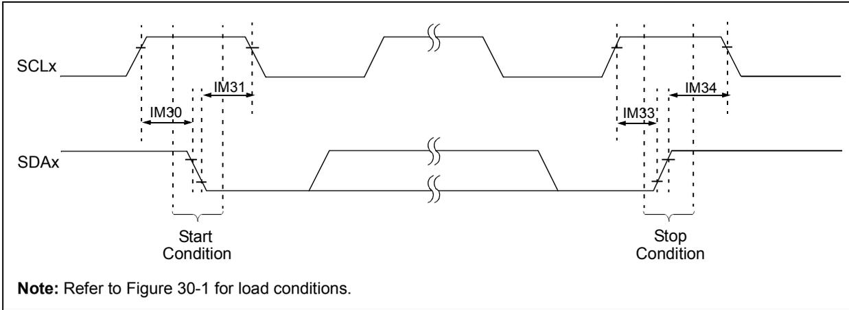
**FIGURE 30-19: I2Cx BUS DATA TIMING CHARACTERISTICS (MASTER MODE)**
