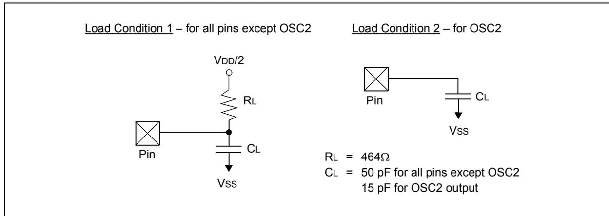
**TABLE 30-15: CAPACITIVE LOADING REQUIREMENTS ON OUTPUT PINS**
