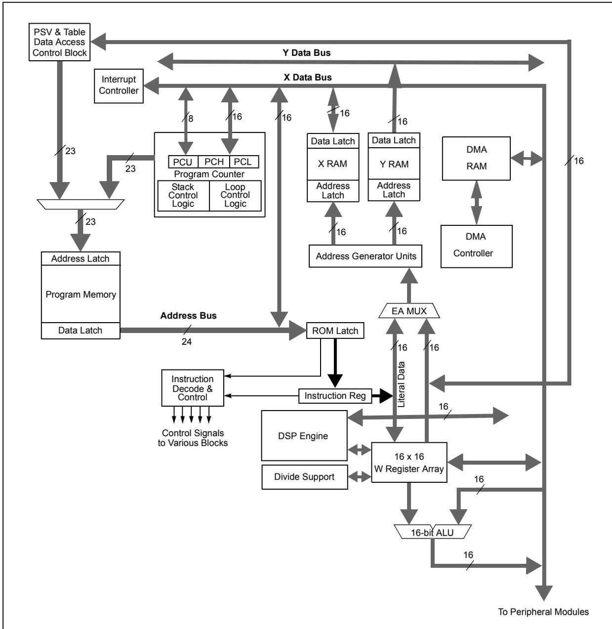
FIGURE 2-2: dsPIC33FJ32MC302/304, dsPIC33FJ64MCX02/X04, AND dsPIC33FJ128MCX02/X04 PROGRAMMER'S MODEL
