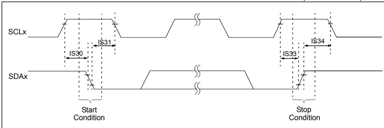
**FIGURE 25-21: I2Cx BUS DATA TIMING CHARACTERISTICS (SLAVE MODE)**
