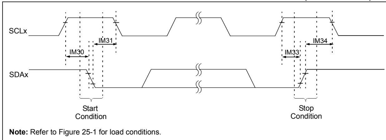
**FIGURE 25-19: I2Cx BUS DATA TIMING CHARACTERISTICS (MASTER MODE)**
