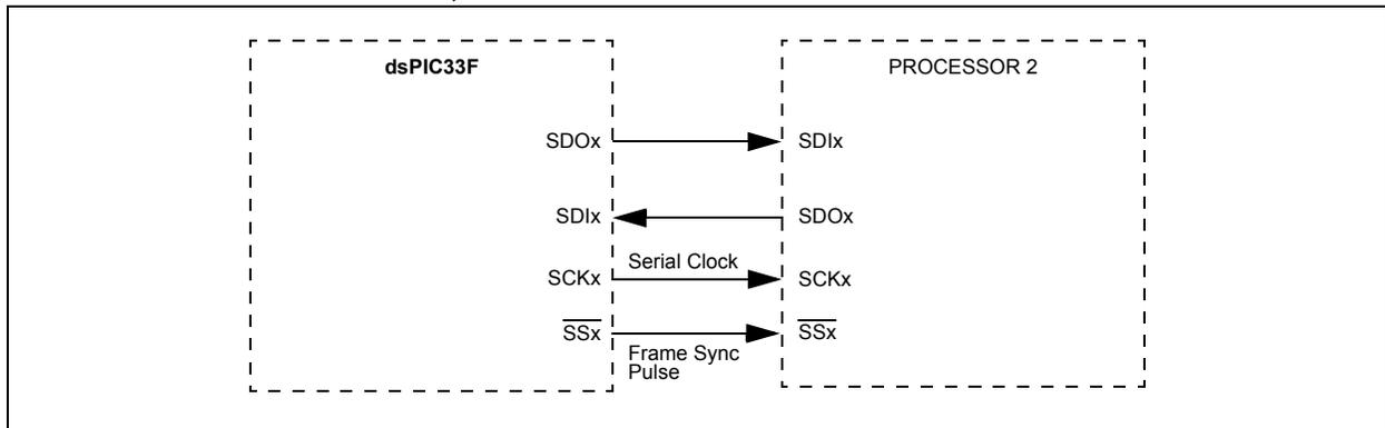
FIGURE 17-4: SPI MASTER, FRAME SLAVE CONNECTION DIAGRAM
