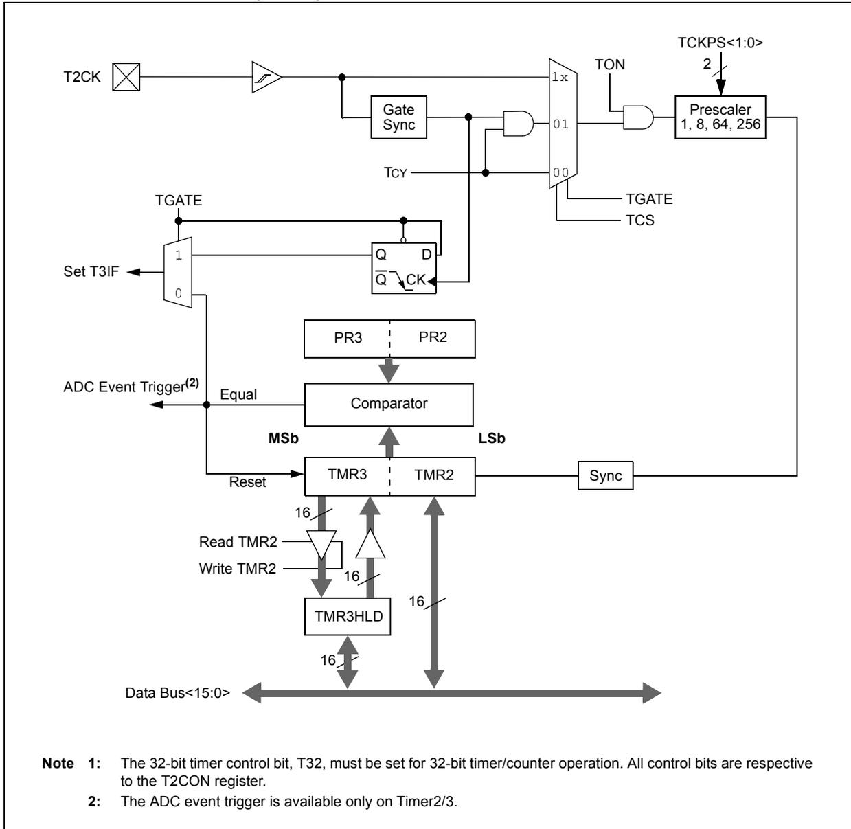
FIGURE 12-2: TIMER2 (16-BIT) BLOCK DIAGRAM
