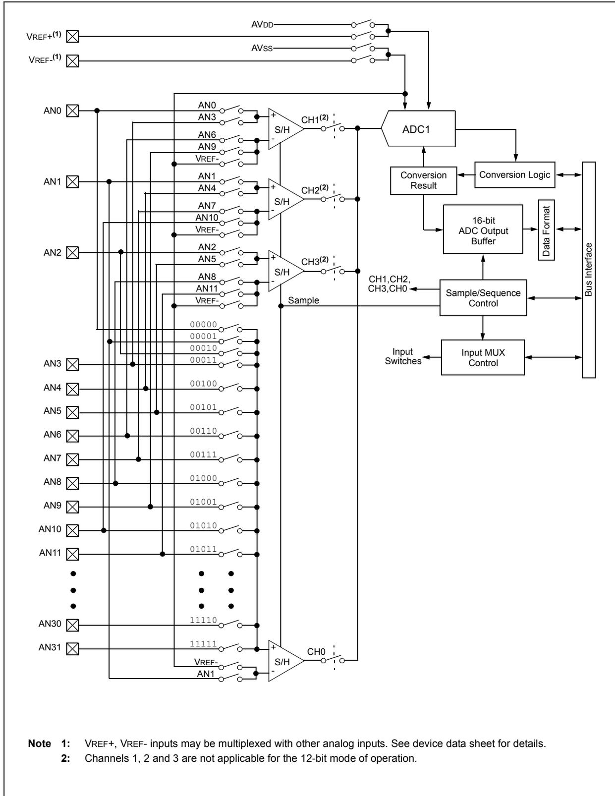
FIGURE 21-2: ADC2 MODULE BLOCK DIAGRAM<sup>(1)</sup>
