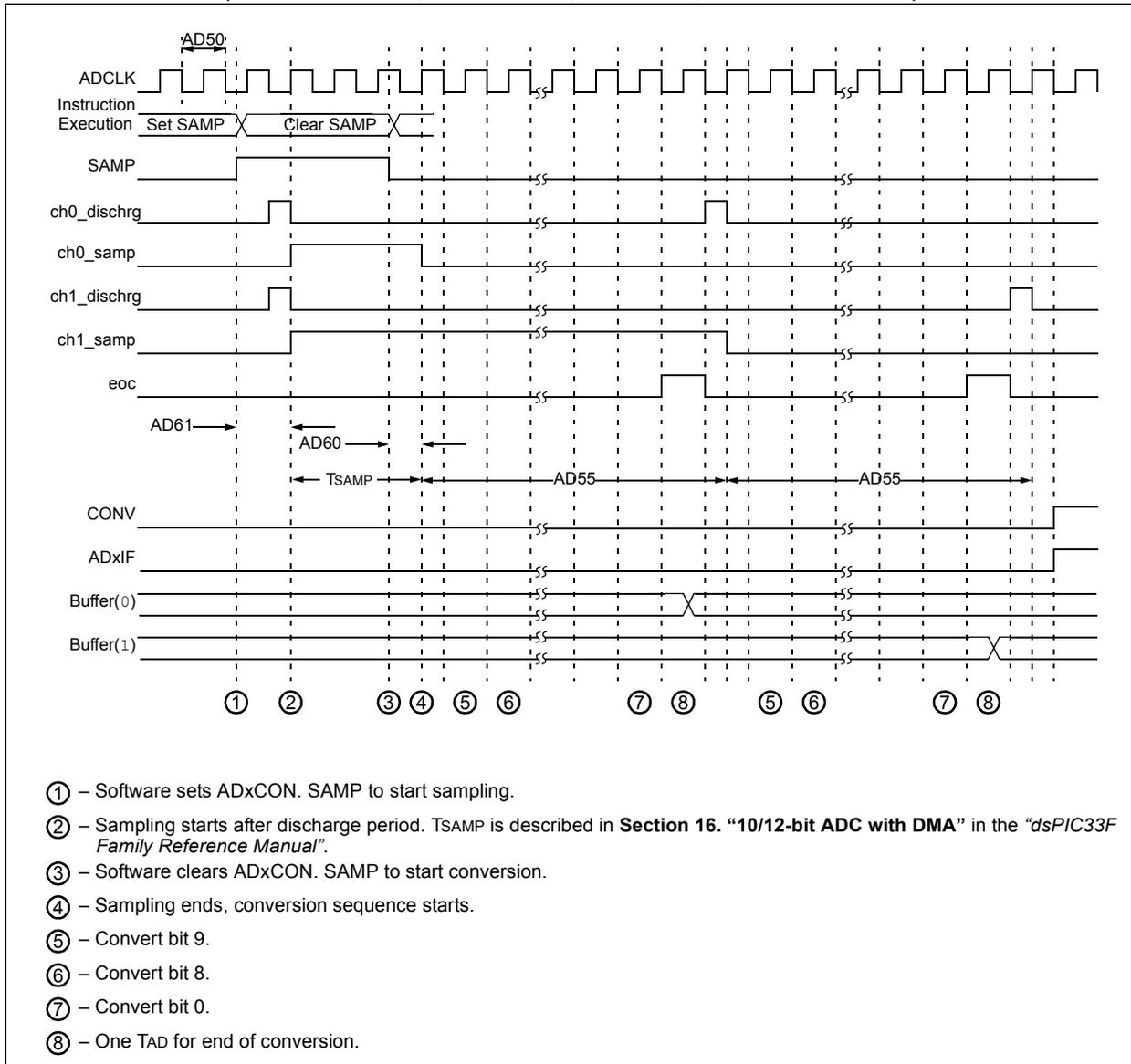
**FIGURE 25-25: ADC CONVERSION (10-BIT MODE) TIMING CHARACTERISTICS (CHPS<1:0> = 01, SIMSAM = 0, ASAM = 1, SSRC<2:0> = 111, SAMC<4:0> = 00001)**
