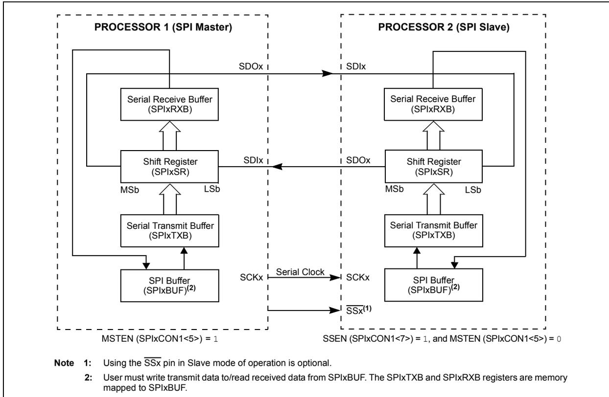
FIGURE 17-3: SPI MASTER, FRAME MASTER CONNECTION DIAGRAM
