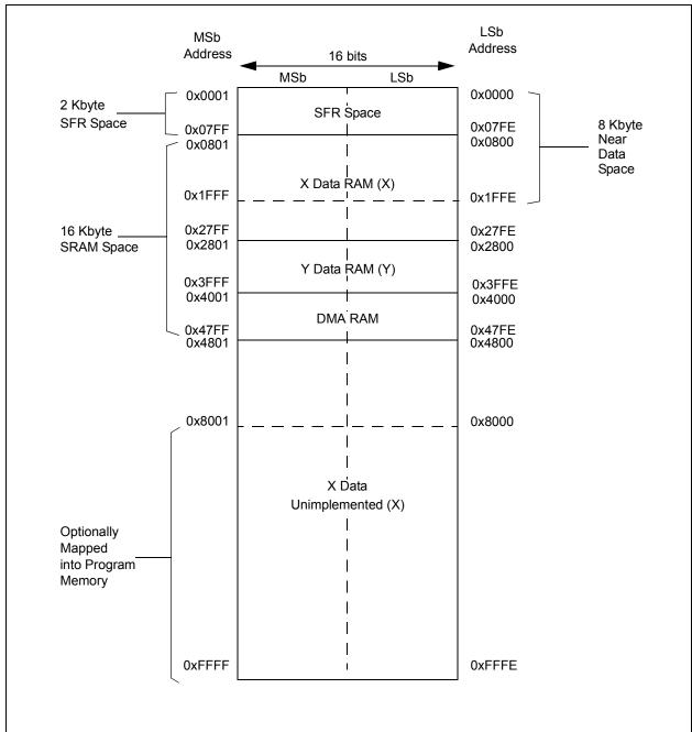
FIGURE 3-5: DATA MEMORY MAP FOR dsPIC33FJXXXGPX06/X08/X10 DEVICES WITH 30 KB RAM
