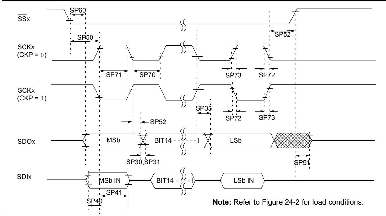
**TABLE 24-36: SPI MODULE SLAVE MODE (CKE = 1) TIMING REQUIREMENTS**
