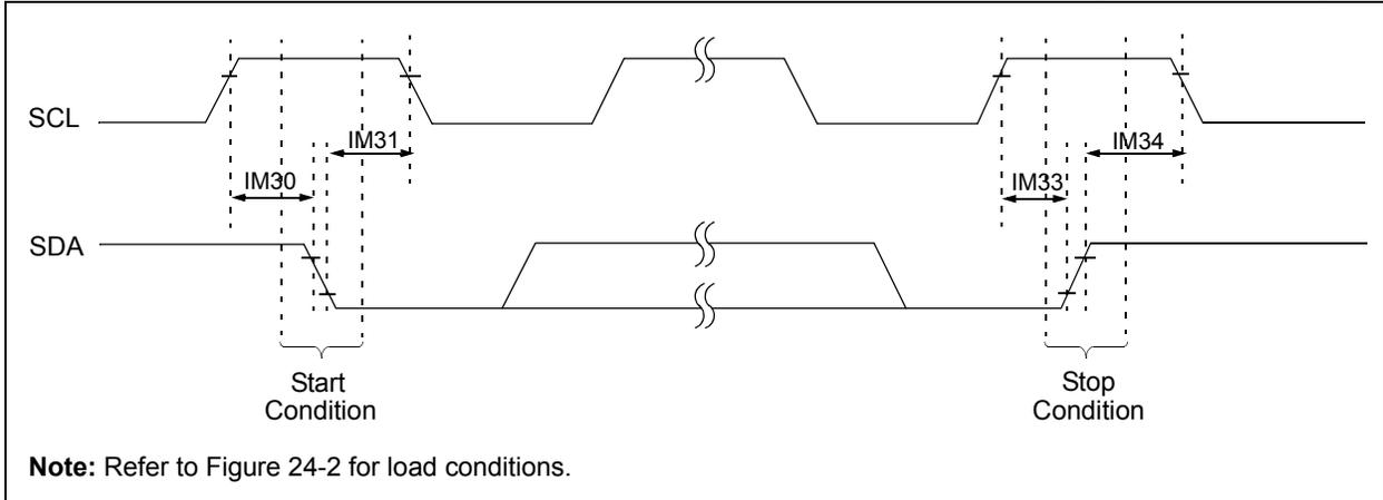
**FIGURE 24-21: I<sup>2</sup>C™ BUS DATA TIMING CHARACTERISTICS (MASTER MODE)**
