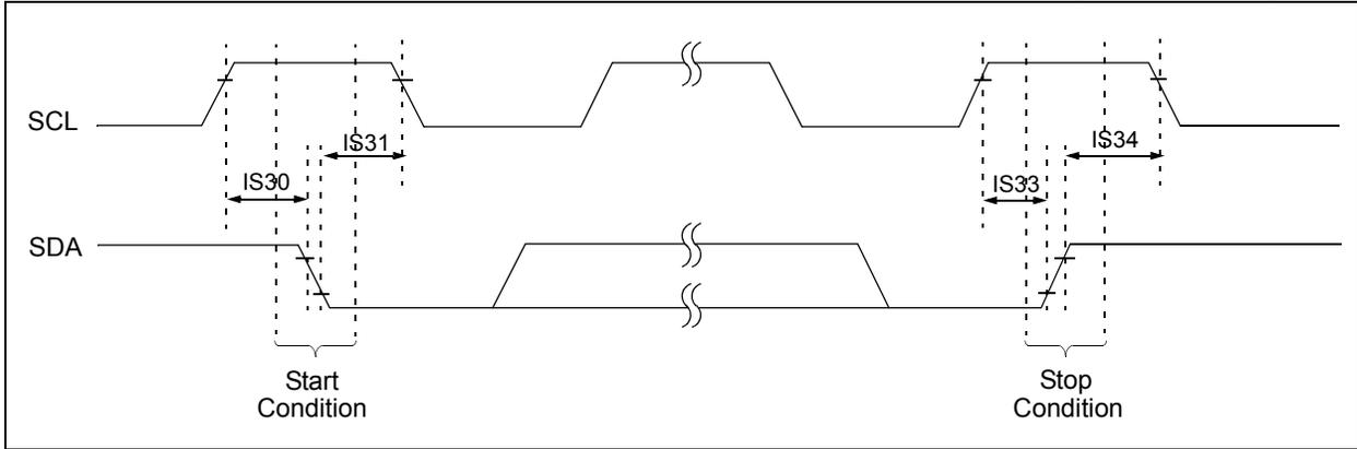
**FIGURE 24-23: I<sup>2</sup>C™ BUS DATA TIMING CHARACTERISTICS (SLAVE MODE)**
