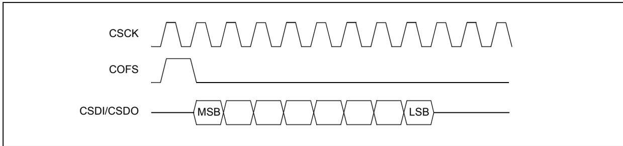
**FIGURE 18-3: FRAME SYNC TIMING, AC-LINK START OF FRAME**
