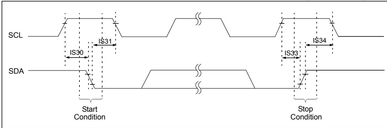
FIGURE 23-21: I<sup>2</sup>C™ BUS DATA TIMING CHARACTERISTICS (SLAVE MODE)
