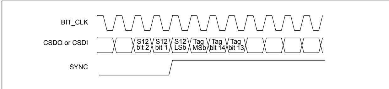
**FIGURE 18-4: I<sup>2</sup>S INTERFACE FRAME SYNC TIMING**
