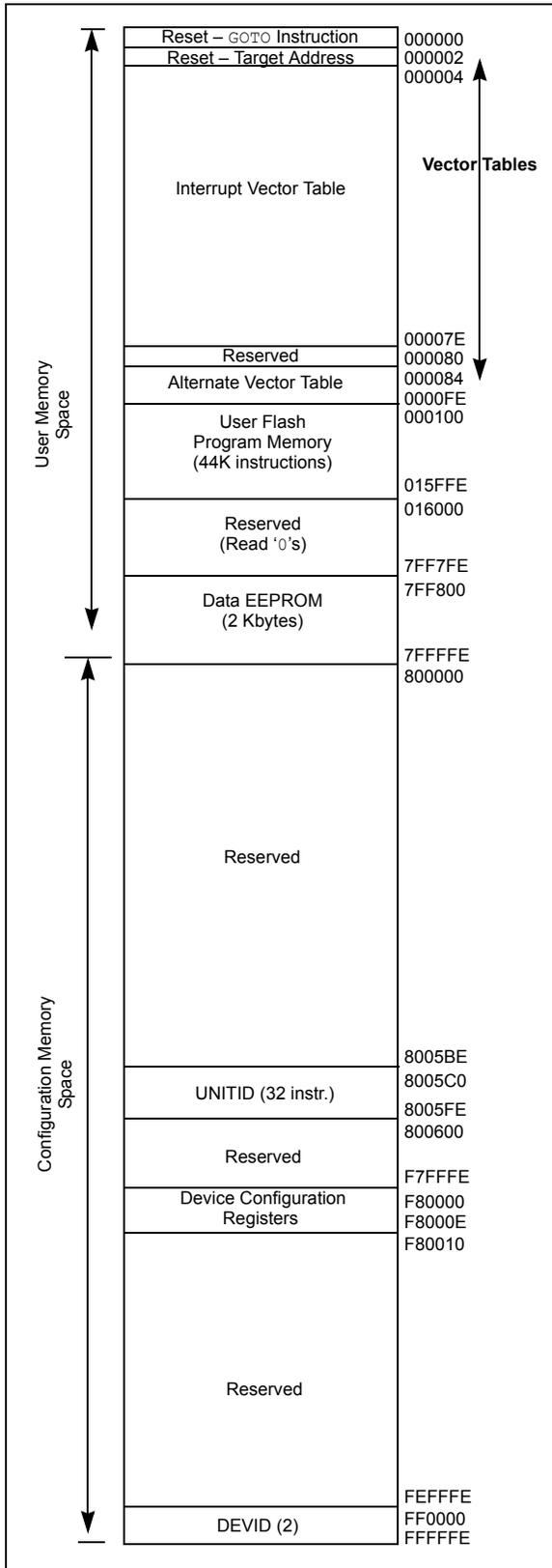
**FIGURE 3-2: PROGRAM SPACE MEMORY MAP FOR dsPIC30F6012A/6014A**
