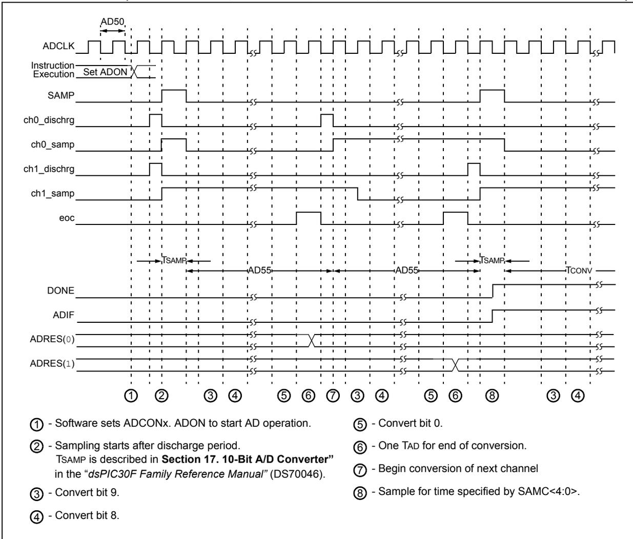
**TABLE 24-40: 10-BIT HIGH-SPEED A/D CONVERSION TIMING REQUIREMENTS**
