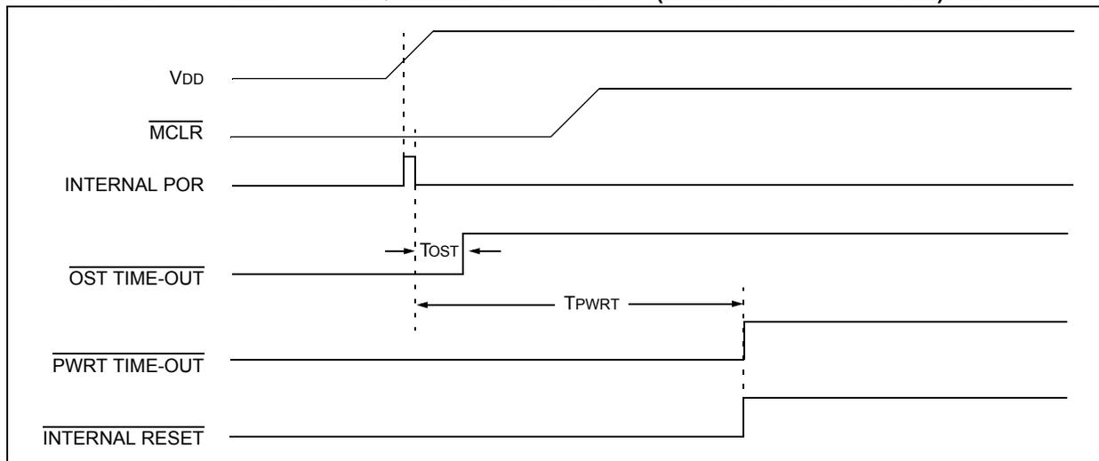
**FIGURE 21-5: TIME-OUT SEQUENCE ON POWER-UP ( $\overline{\text{MCLR}}$  NOT TIED TO  $V_{\text{DD}}$ ): CASE 2**
