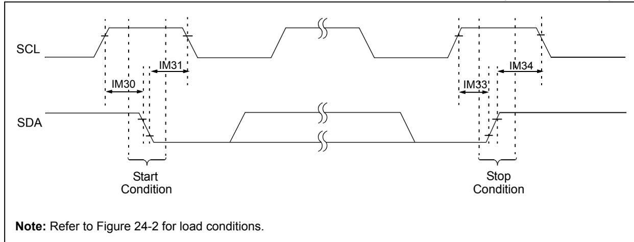
FIGURE 24-21: I<sup>2</sup>C™ BUS DATA TIMING CHARACTERISTICS (MASTER MODE)
