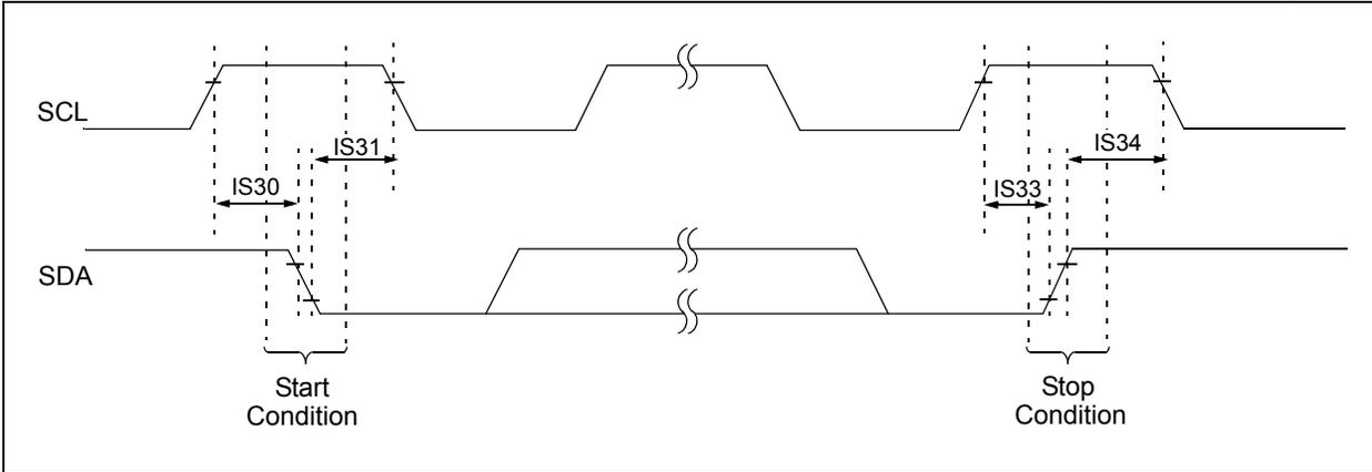
**FIGURE 24-23: I<sup>2</sup>C™ BUS DATA TIMING CHARACTERISTICS (SLAVE MODE)**
