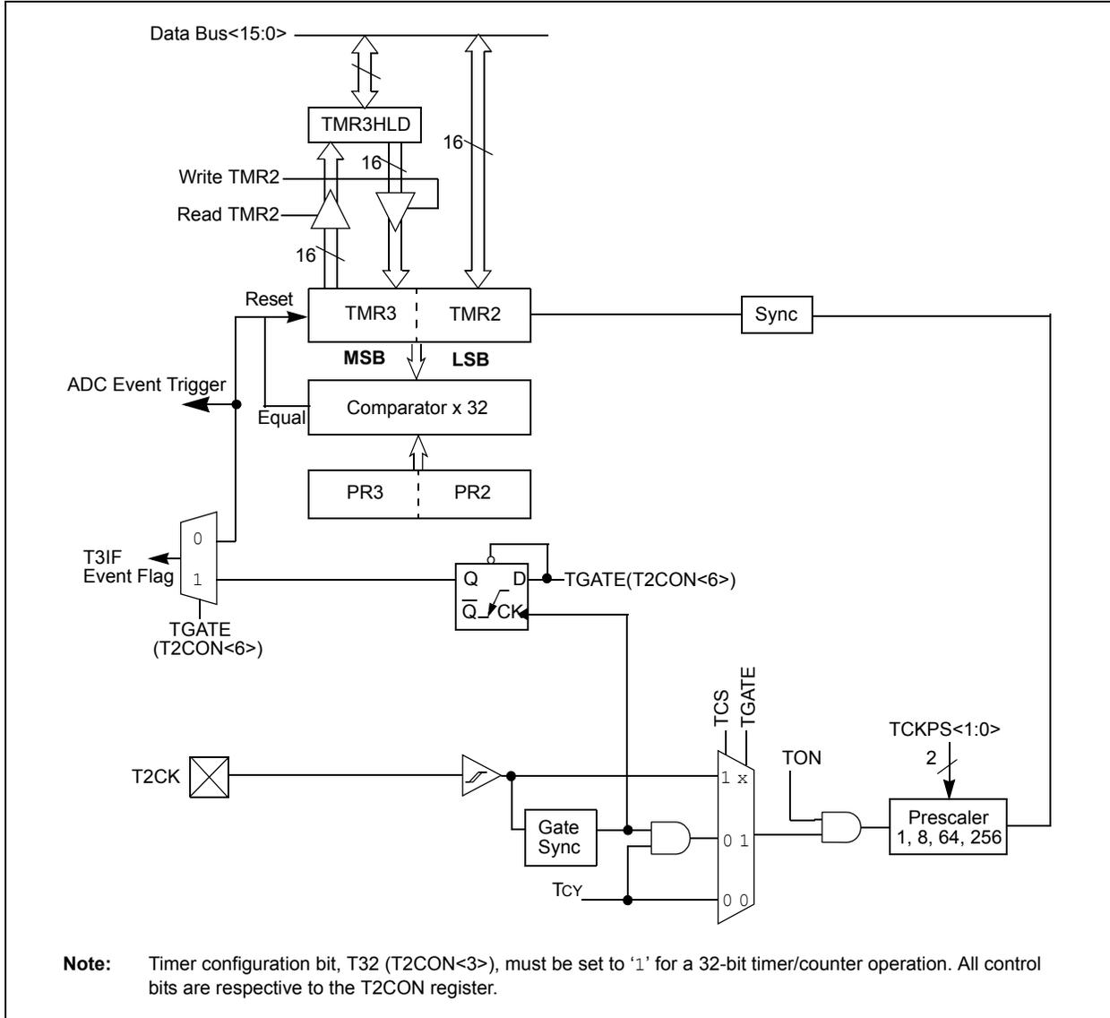
**FIGURE 10-2: 16-BIT TIMER2 BLOCK DIAGRAM**
