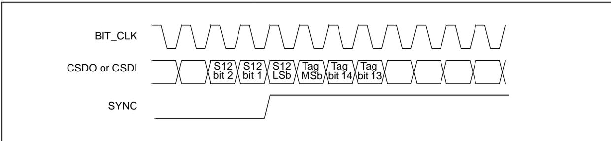
**FIGURE 18-4: I<sup>2</sup>S INTERFACE FRAME SYNC TIMING**
