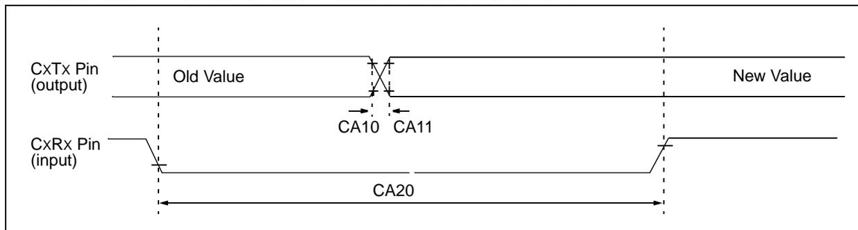
**TABLE 23-36: CAN MODULE I/O TIMING REQUIREMENTS**
