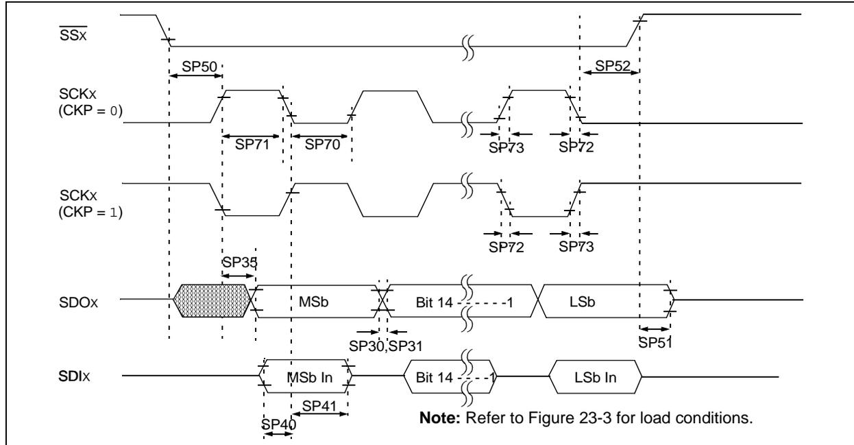
**TABLE 23-32: SPI MODULE SLAVE MODE (CKE = 0) TIMING REQUIREMENTS**
