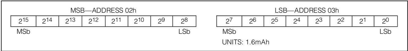
Figure 16. Remaining Active Absolute Capacity (RAAC) [mAh]
