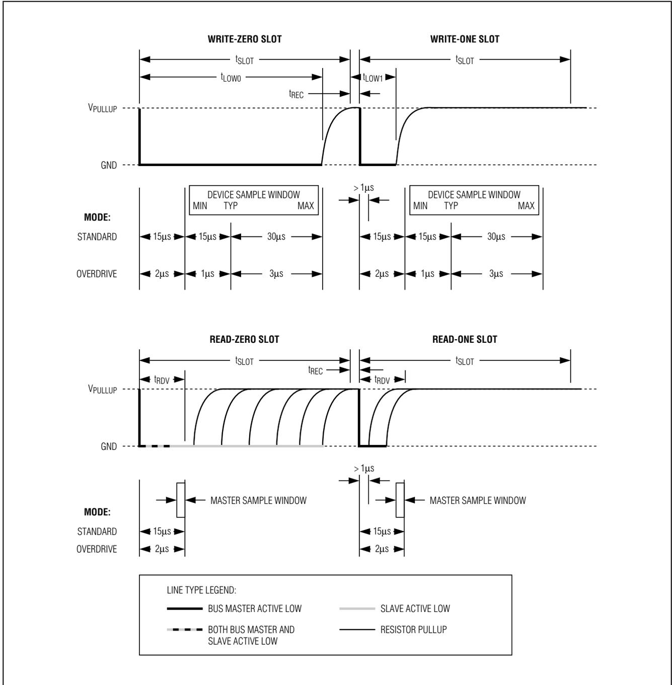
Figure 30. 1-Wire Write and Read Time Slots
