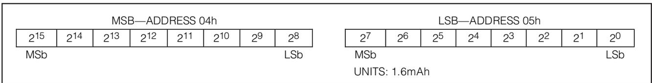
Figure 17. Remaining Standby Absolute Capacity (RSAC) [mAh]
