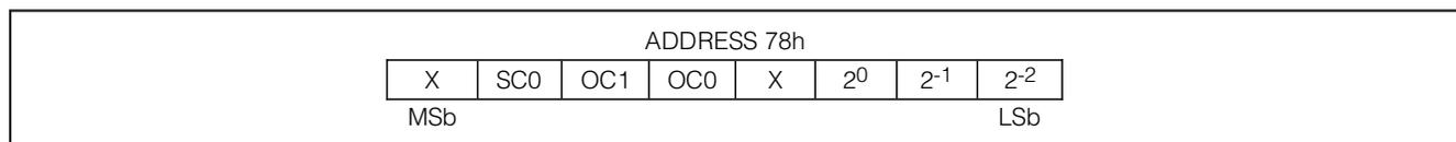
Figure 20. Overcurrent and Short-Circuit Threshold Bits Format
