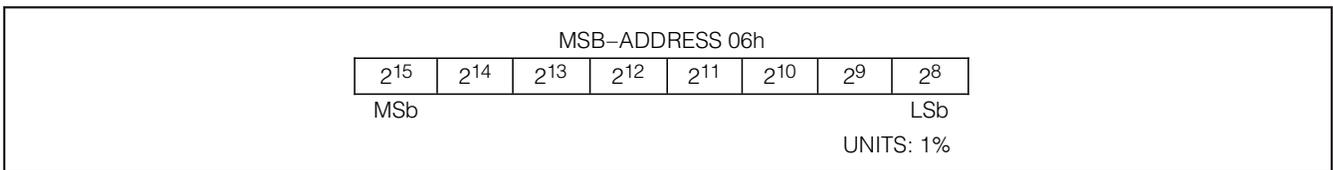
Figure 18. Remaining Active Relative Capacity (RARC) [%]
