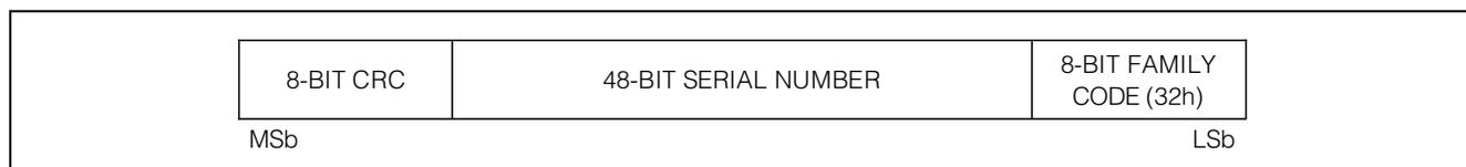
Figure 22. 1-Wire Net Address Format (ROM ID)
