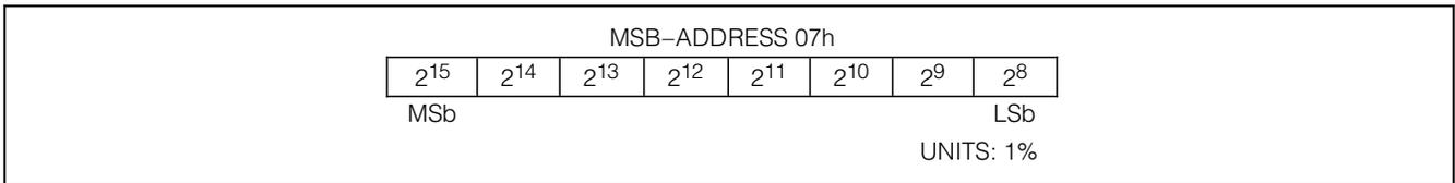
Figure 19. Remaining Standby Relative Capacity (RSRC) [%]
