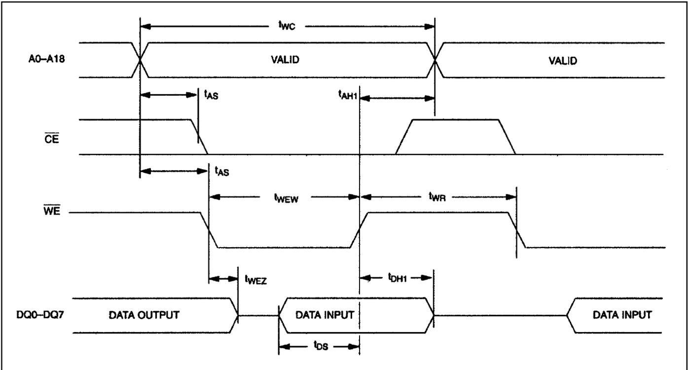
Figure 7. Write Cycle Timing, Chip-Enable Controlled
