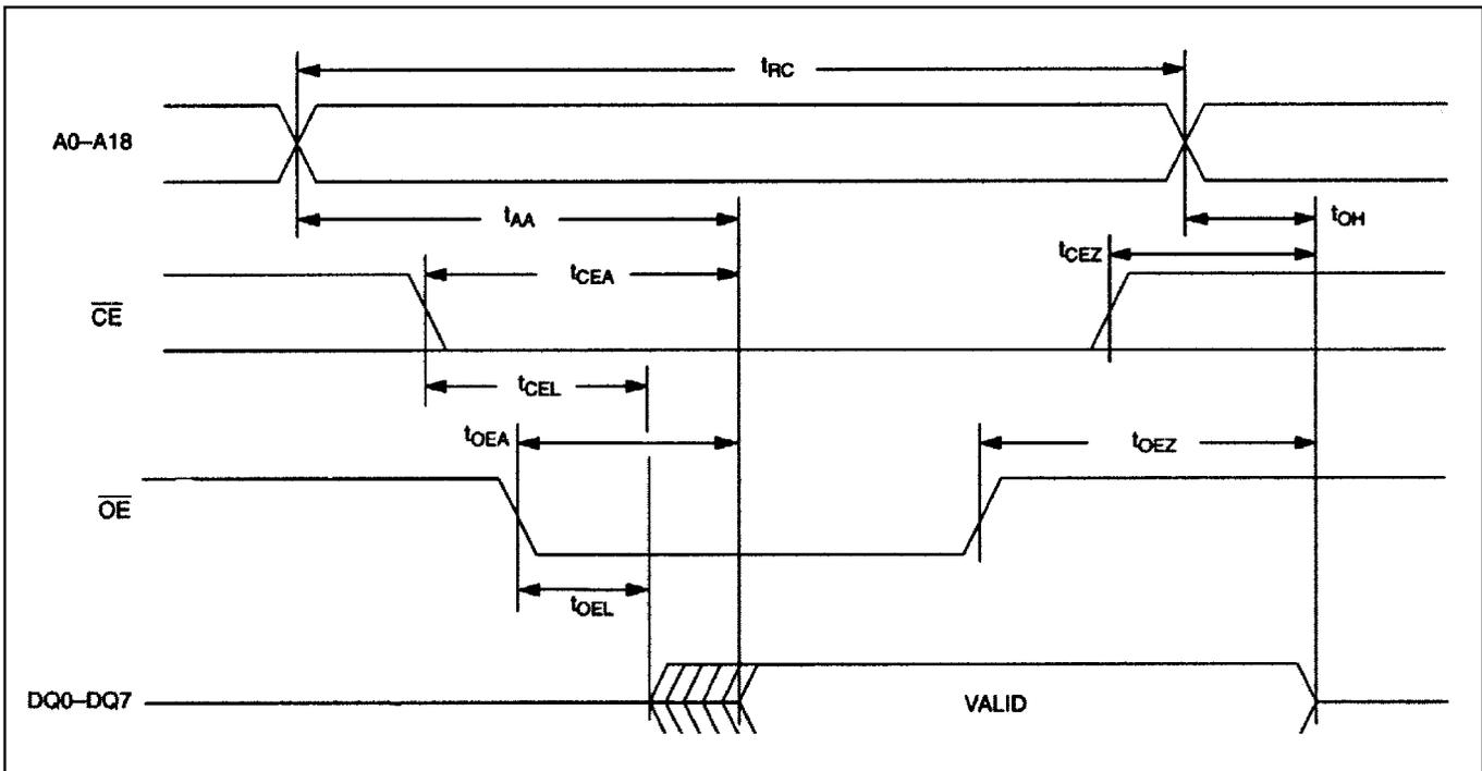
**AC CHARACTERISTICS—READ CYCLE**(T<sub>A</sub> = Over the Operating Range)
