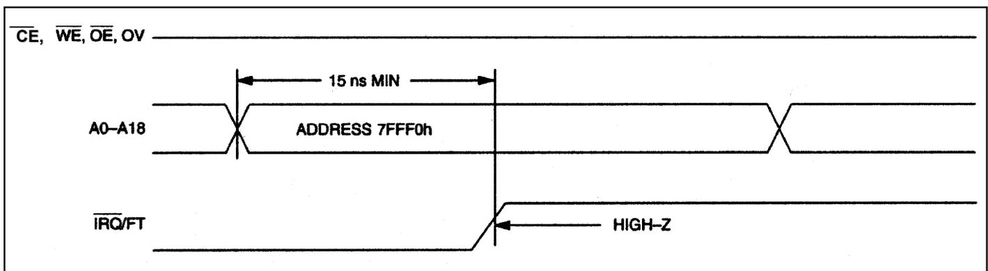
**Figure 3. Clearing  $\overline{\text{IRQ}}$  Waveforms**
