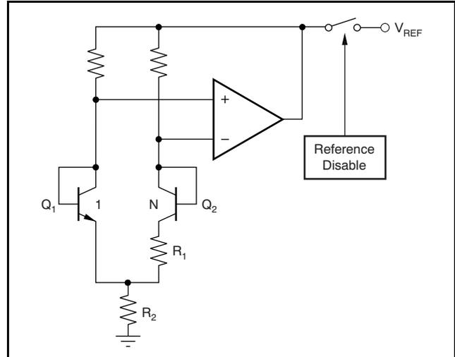
Figure 94. Simplified Schematic of the Bandgap Reference
