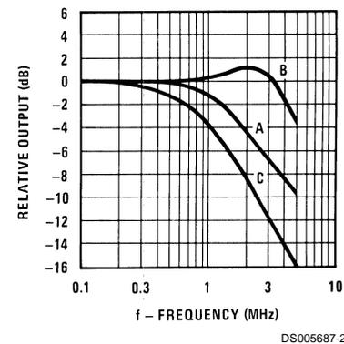
Unless otherwise specified:  $R_{14} = R_{15} = 1\text{ k}\Omega$ ,  $C = 15\text{ pF}$ , pin 16 to  $V_{EE}$ ;  $R_L = 50\Omega$ , pin 4 to ground.
