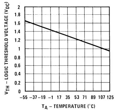
**Typical Performance Characteristics**  $V_{CC} = 5V$ ,  $V_{EE} = -15V$ ,  $T_A = 25^\circ C$ , unless otherwise noted (Continued)
