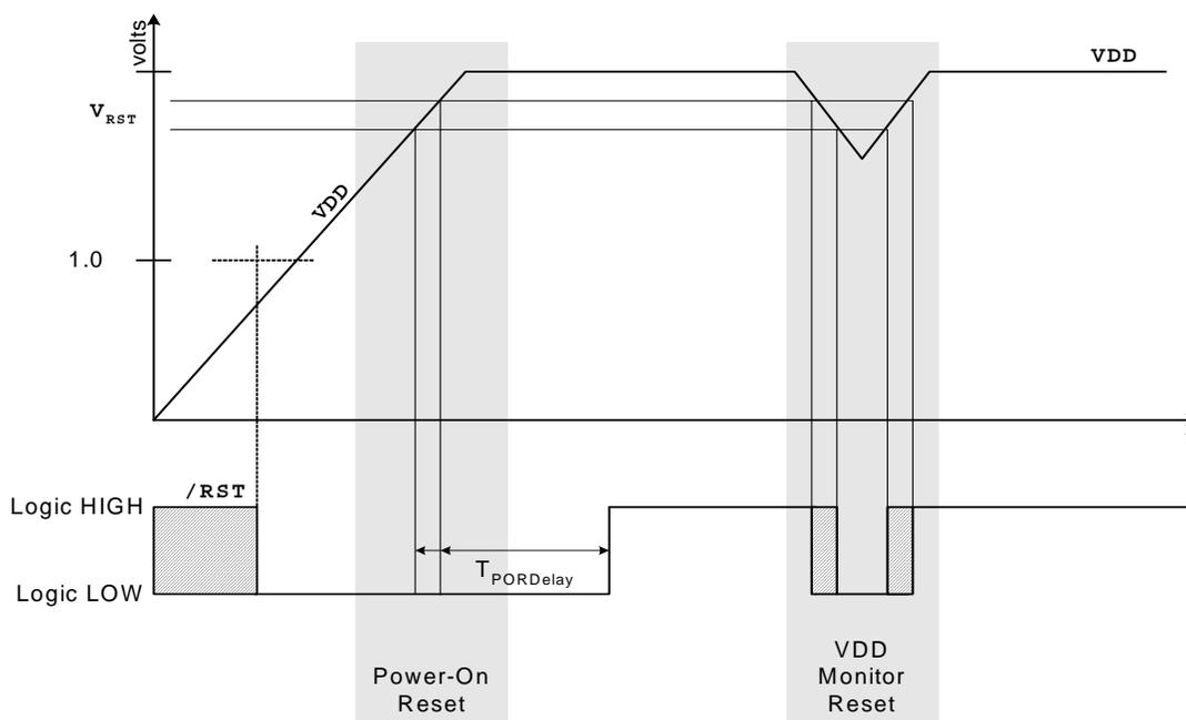
Figure 12.2. Power-On and  $V_{\text{DD}}$  Monitor Reset Timing
