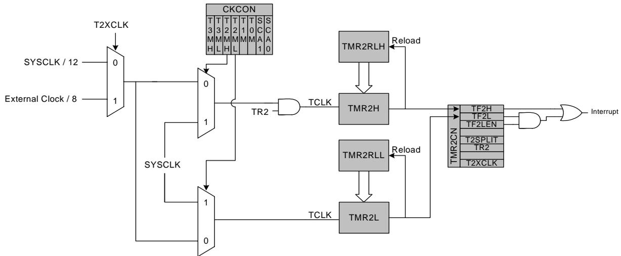
Figure 19.5. Timer 2 8-Bit Mode Block Diagram
