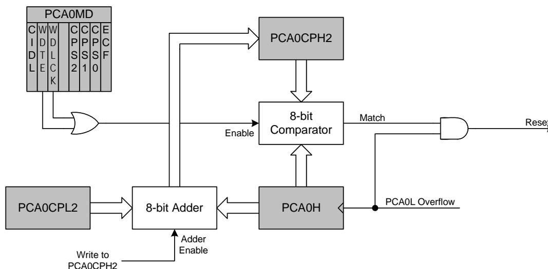
Figure 20.10. PCA Module 2 with Watchdog Timer Enabled
