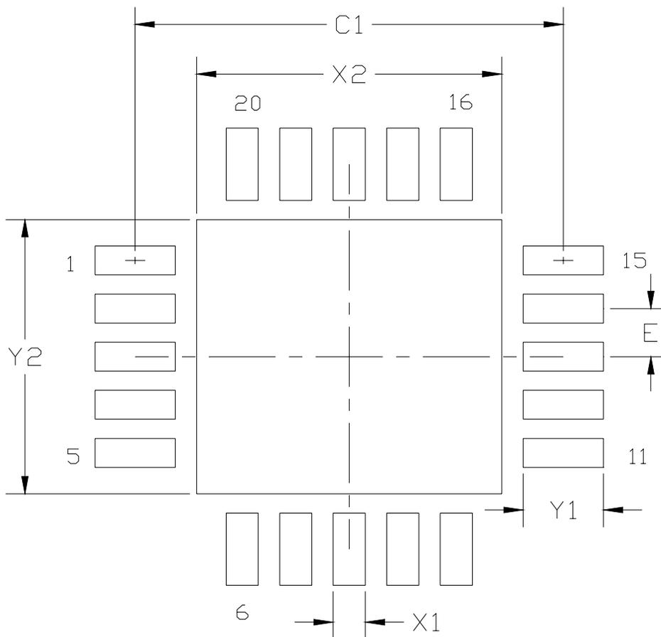
**Figure 4.6. QFN-20 Landing Diagram**
