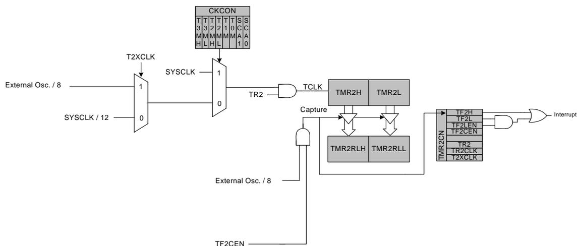
Figure 19.6. Timer 2 Capture Mode Block Diagram
