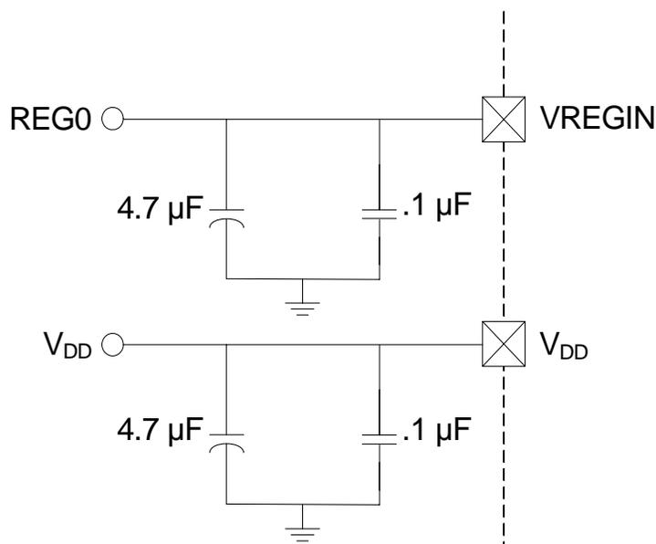
Figure 7.1. External Capacitors for Voltage Regulator Input/Output
