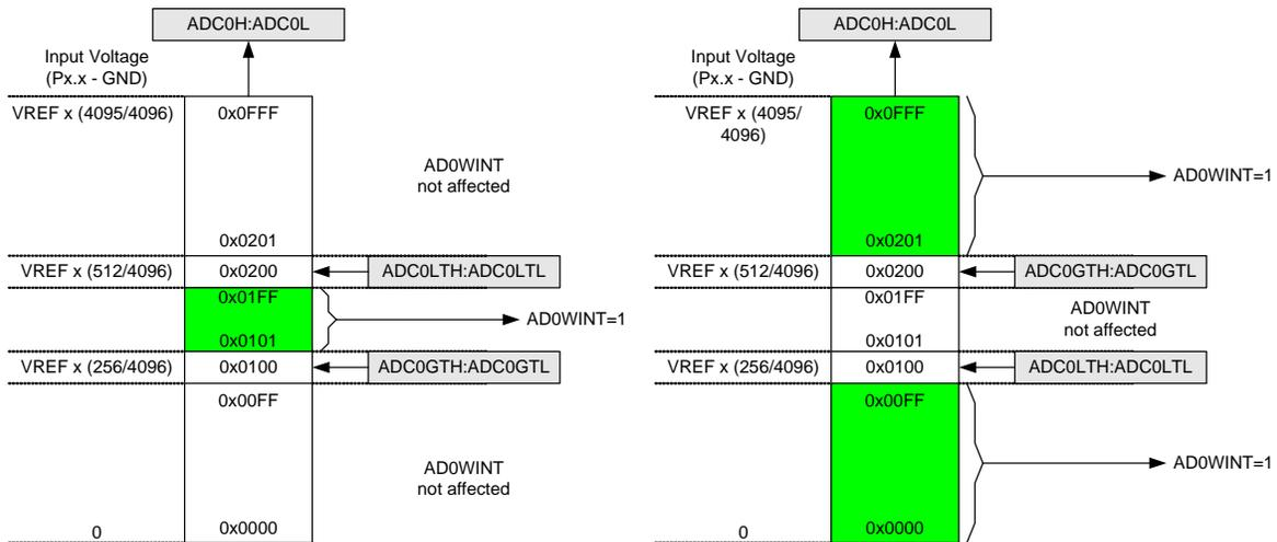
Figure 5.7. ADC Window Compare Example: Right-Justified Single-Ended Data
