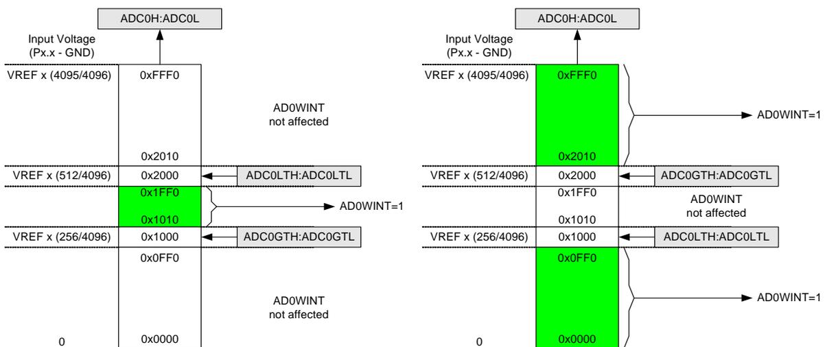
Figure 5.8. ADC Window Compare Example: Left-Justified Single-Ended Data
