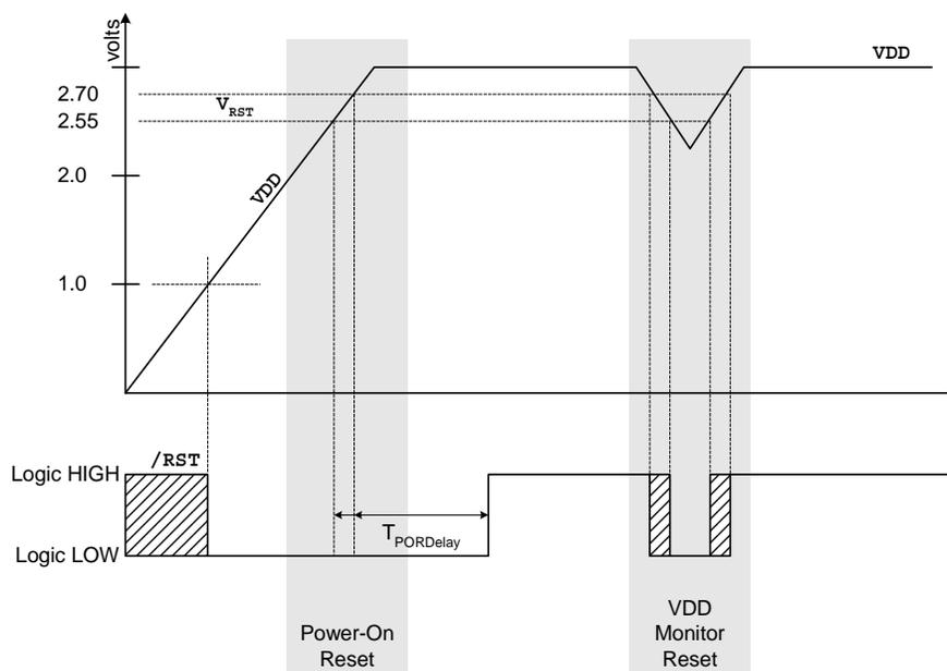
Figure 14.2. Power-On and  $V_{\text{DD}}$  Monitor Reset Timing
