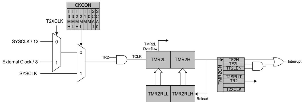
Figure 22.4. Timer 2 16-Bit Mode Block Diagram
