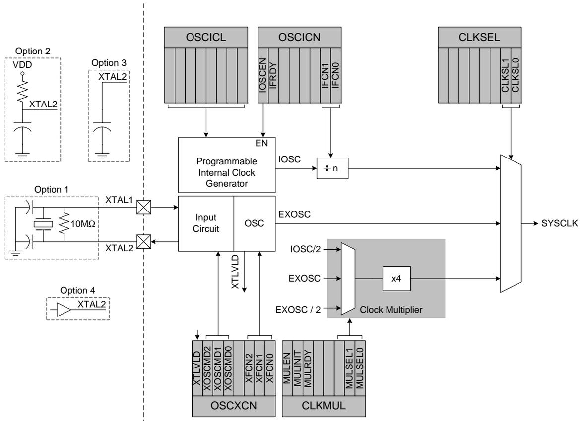
**Figure 17.1. Oscillator Diagram**
