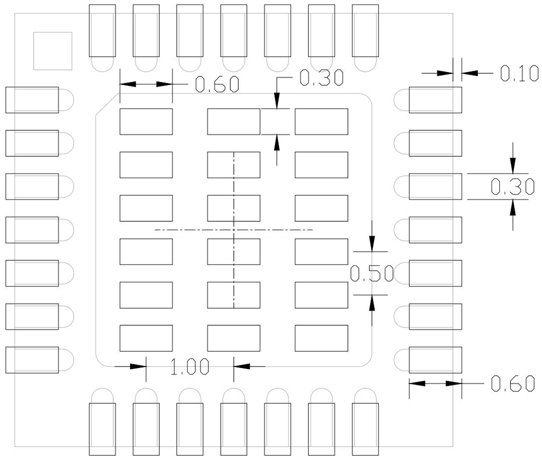
Figure 4.6. Typical QFN-28 Solder Paste Diagram
