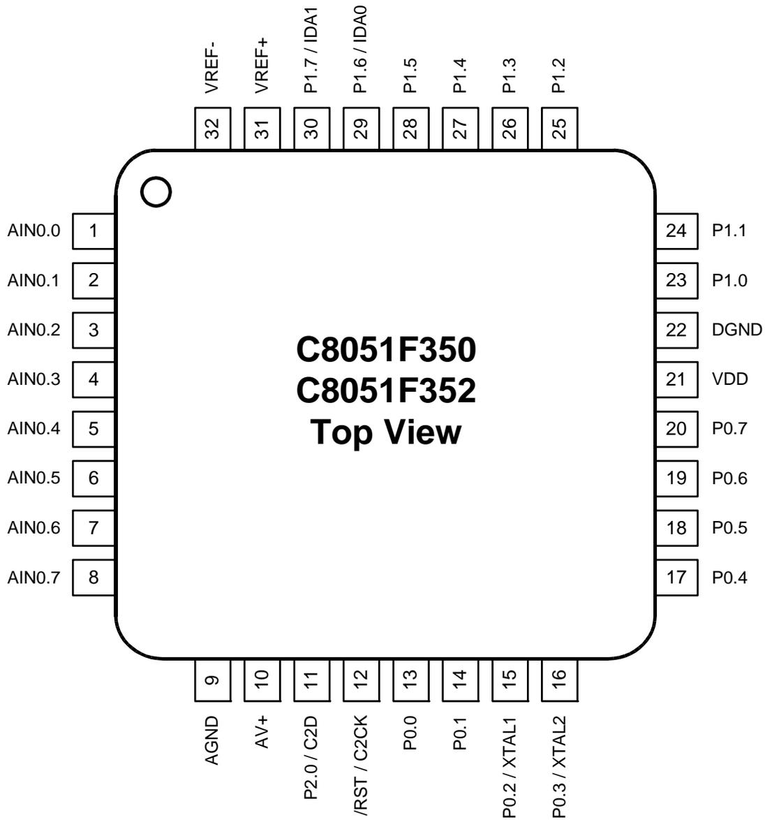
Figure 4.1. LQFP-32 Pinout Diagram (Top View)
