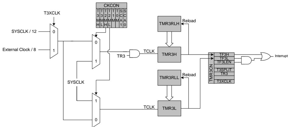
Figure 22.7. Timer 3 8-Bit Mode Block Diagram
