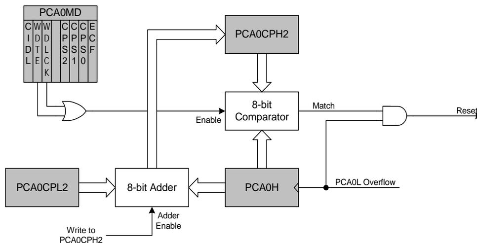
**Figure 23.10. PCA Module 2 with Watchdog Timer Enabled**
