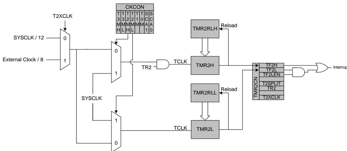
Figure 22.5. Timer 2 8-Bit Mode Block Diagram
