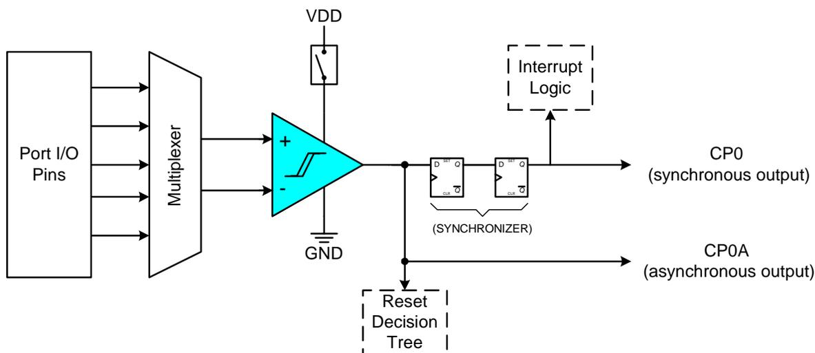
Figure 1.9. Comparator0 Block Diagram
