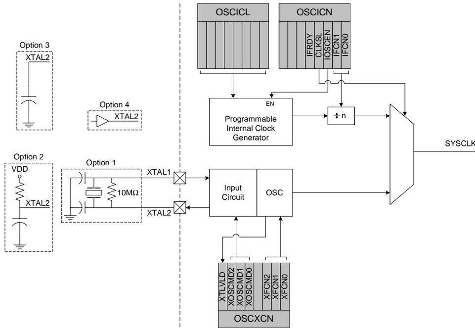
**Figure 11.1. Oscillator Diagram**
