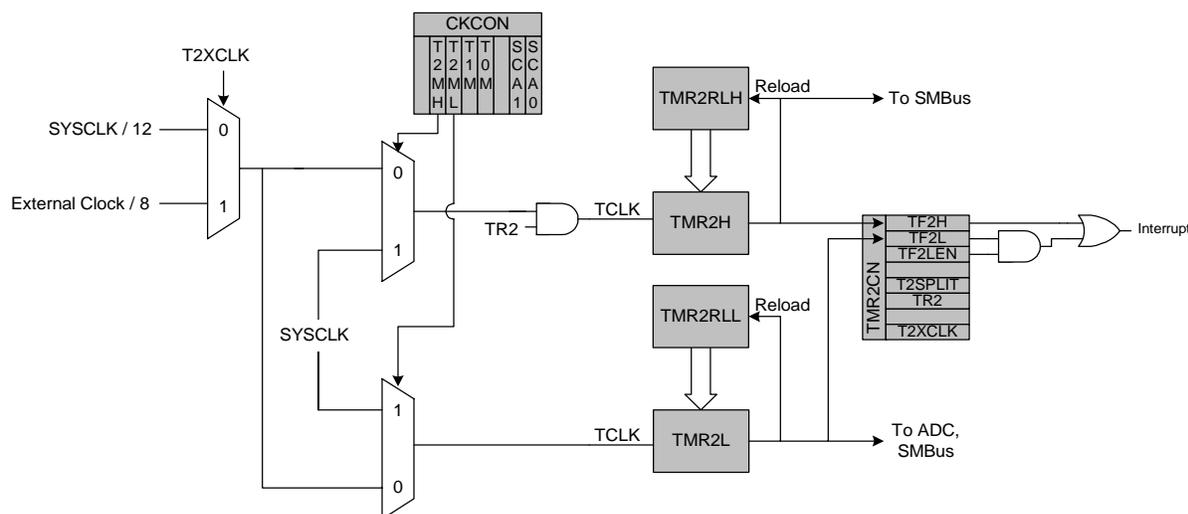
Figure 15.5. Timer 2 8-Bit Mode Block Diagram
