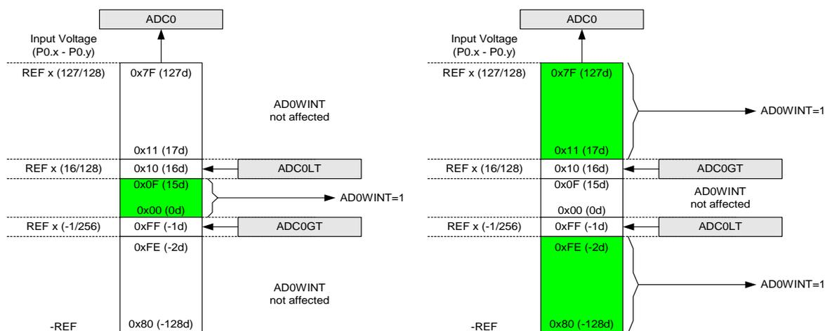
Figure 5.7. ADC Window Compare Examples, Differential Mode
