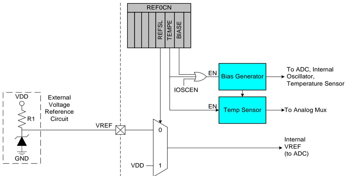
Figure 6.1. Voltage Reference Functional Block Diagram
