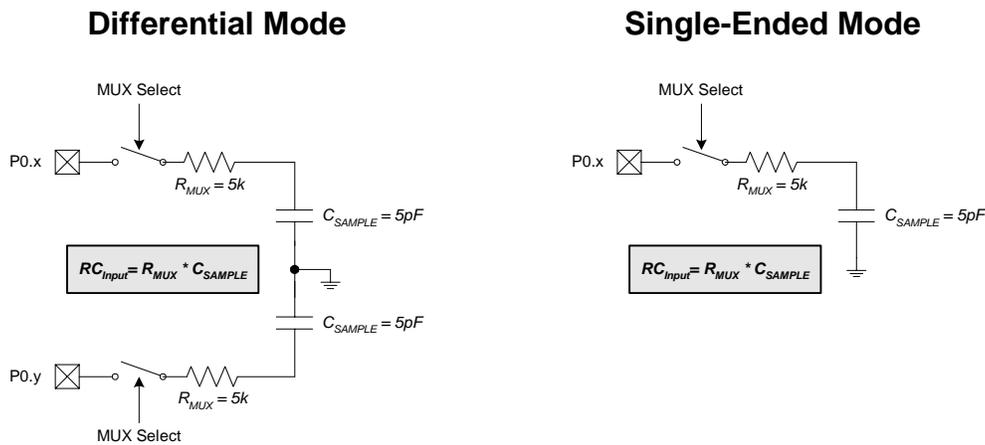
Note: When the PGA gain is set to 0.5,  $C_{SAMPLE} = 3pF$
