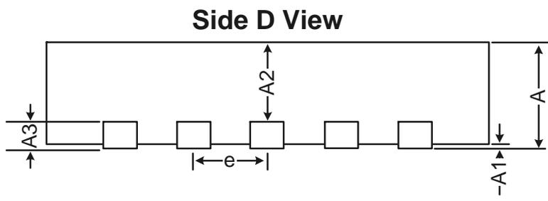
**Figure 4.2. QFN-11 Package Drawing**
