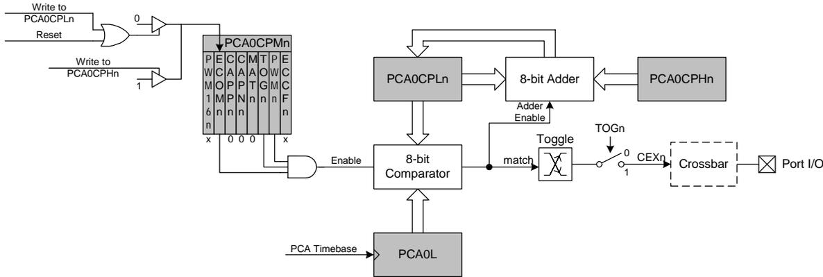
Figure 16.7. PCA Frequency Output Mode
