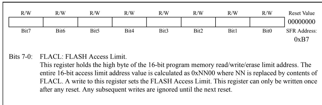
**Figure 15.3. FLSCL: FLASH Memory Control**
