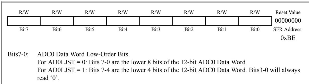
**Figure 5.11. ADC0 Data Word Example (C8051F020/1)**
