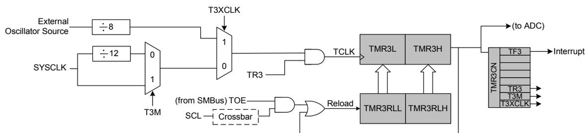
**Figure 22.20. TMR3CN: Timer 3 Control Register**
