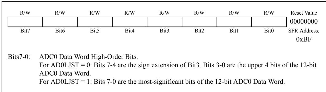
**Figure 5.10. ADC0L: ADC0 Data Word LSB Register (C8051F020/1)**
