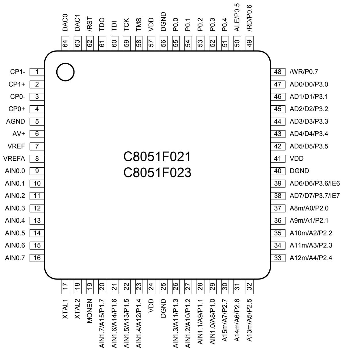
Figure 4.4. TQFP-64 Package Drawing
