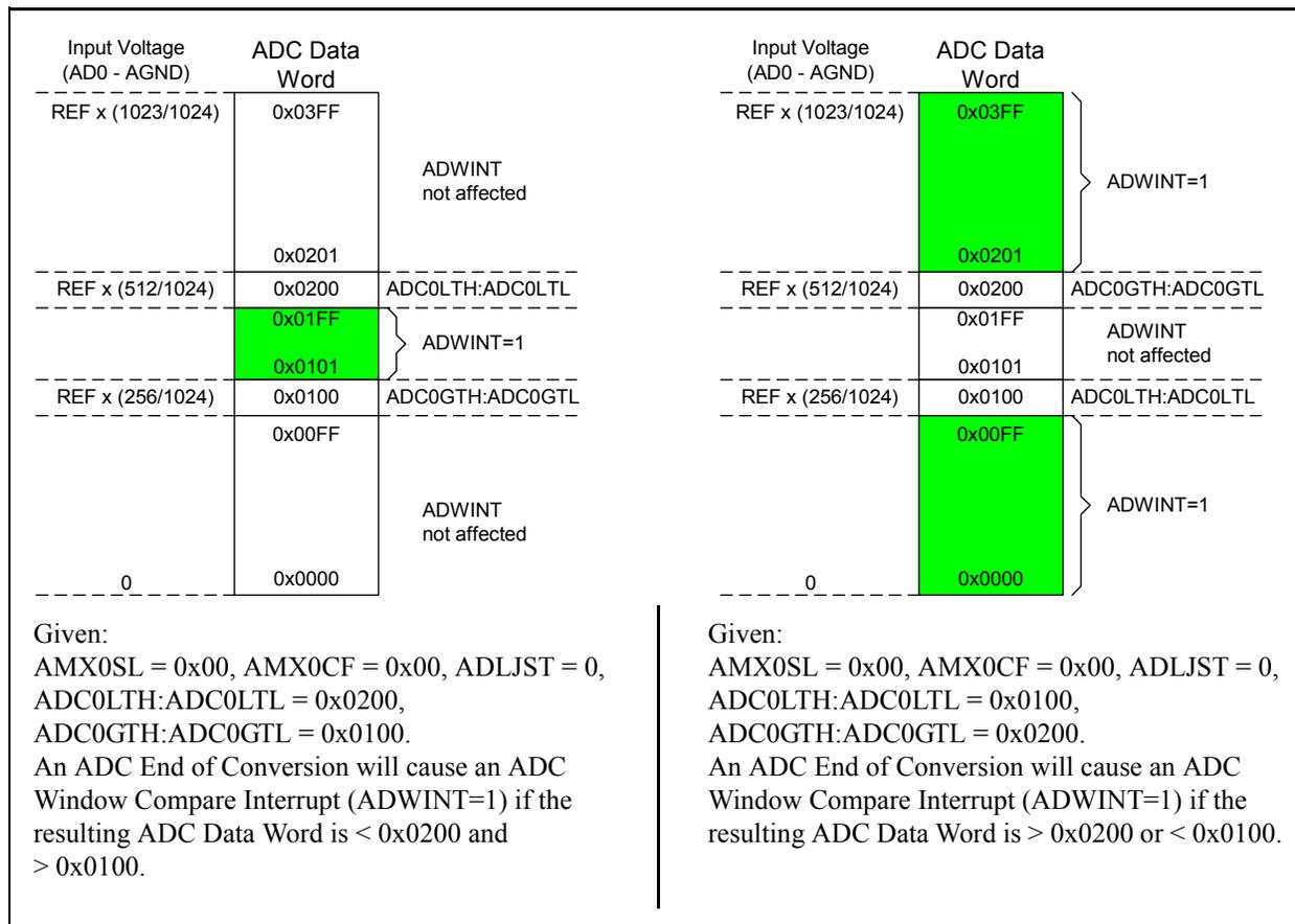
**Figure 6.17. 10-Bit ADC0 Window Interrupt Example: Right Justified Differential Data**
