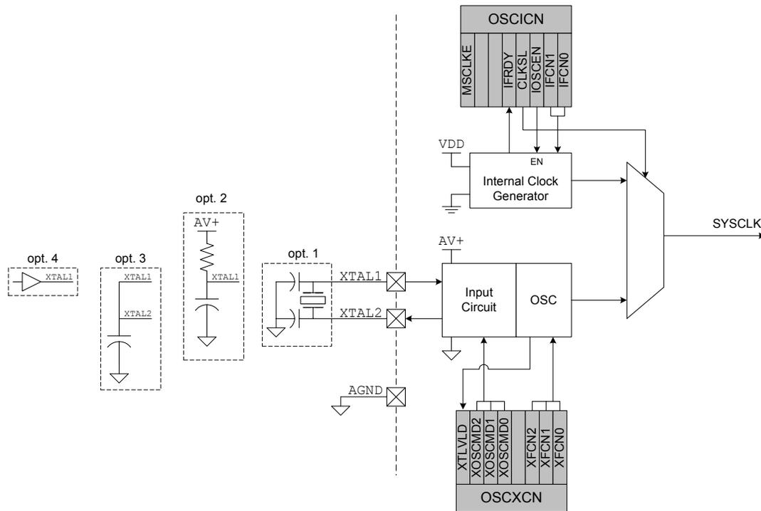
**Figure 14.2. OSCICN: Internal Oscillator Control Register**
