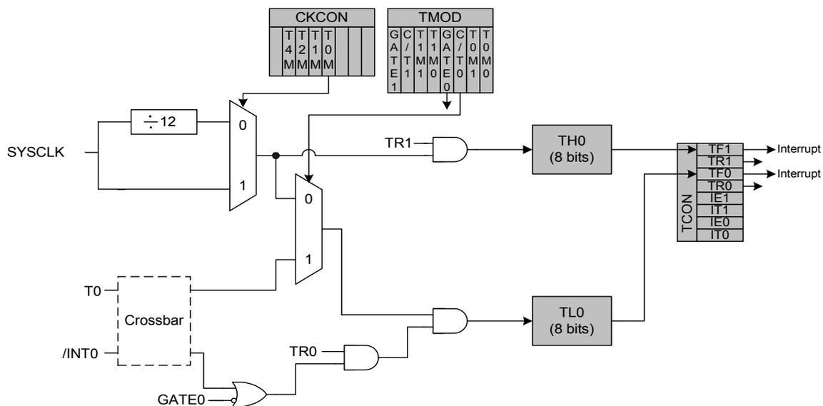
**Figure 22.5. TCON: Timer Control Register**
