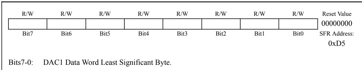
**Figure 8.7. DAC1CN: DAC1 Control Register**
