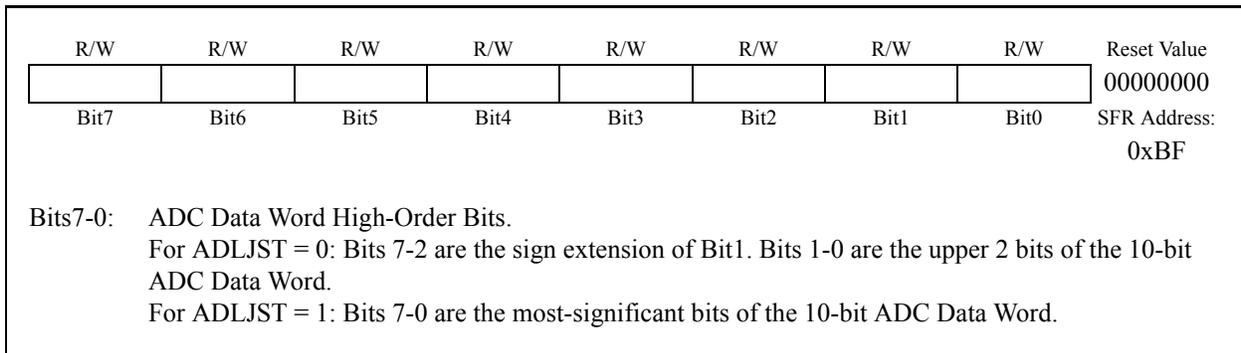
**Figure 6.10. ADC0L: ADC0 Data Word LSB Register (C8051F022/3)**
