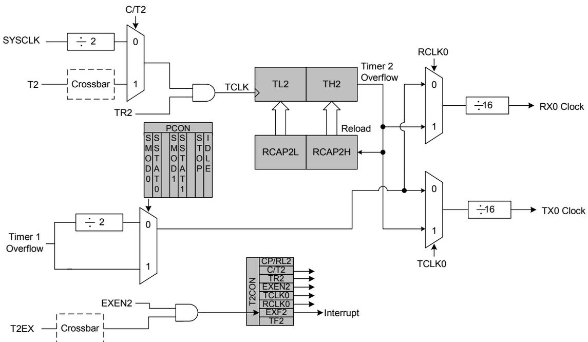
**Figure 22.14. T2CON: Timer 2 Control Register**
