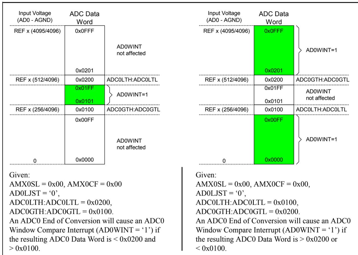
**Figure 5.17. 12-Bit ADC0 Window Interrupt Example: Right Justified Differential Data**
