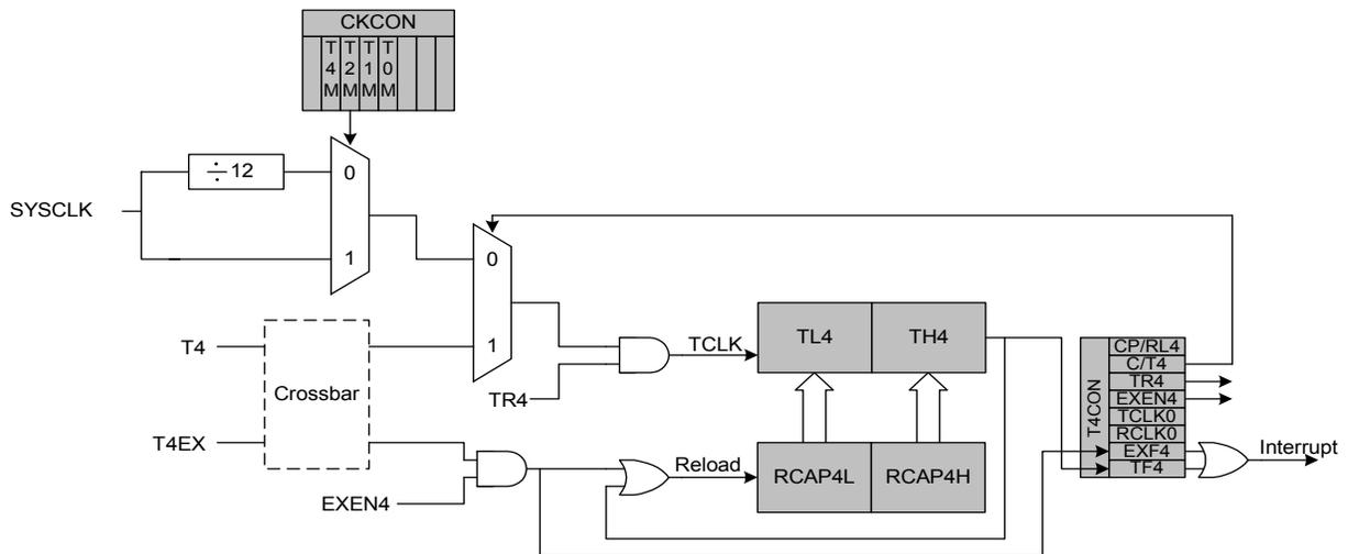
**Figure 22.28. T4CON: Timer 4 Control Register**
