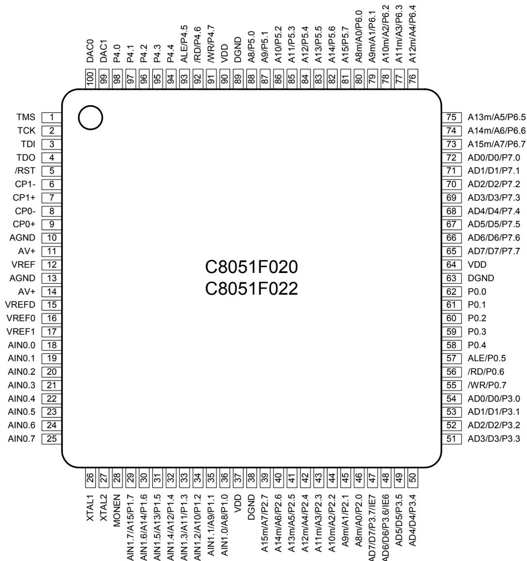
Figure 4.2. TQFP-100 Package Drawing
