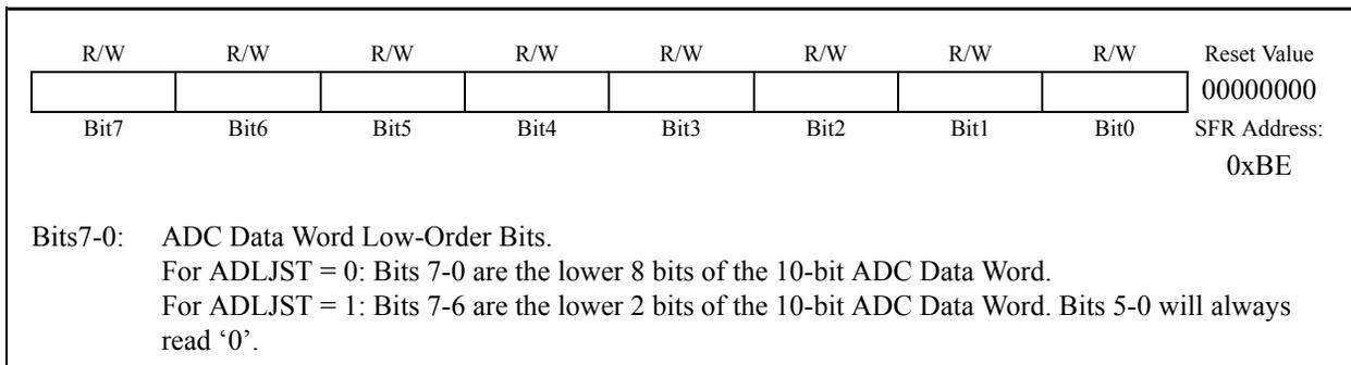
**Figure 6.11. ADC0 Data Word Example (C8051F022/3)**
