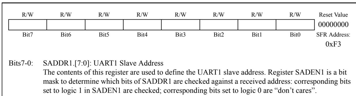
**Figure 21.11. SADEN1: UART1 Slave Address Enable Register**
