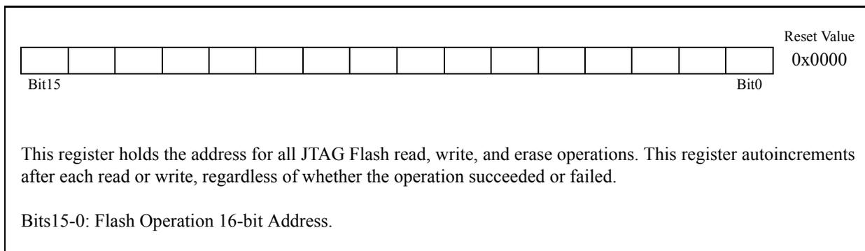
**Figure 24.5. FLASHDAT: JTAG Flash Data Register**
