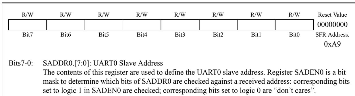
**Figure 20.11. SADEN0: UART0 Slave Address Enable Register**
