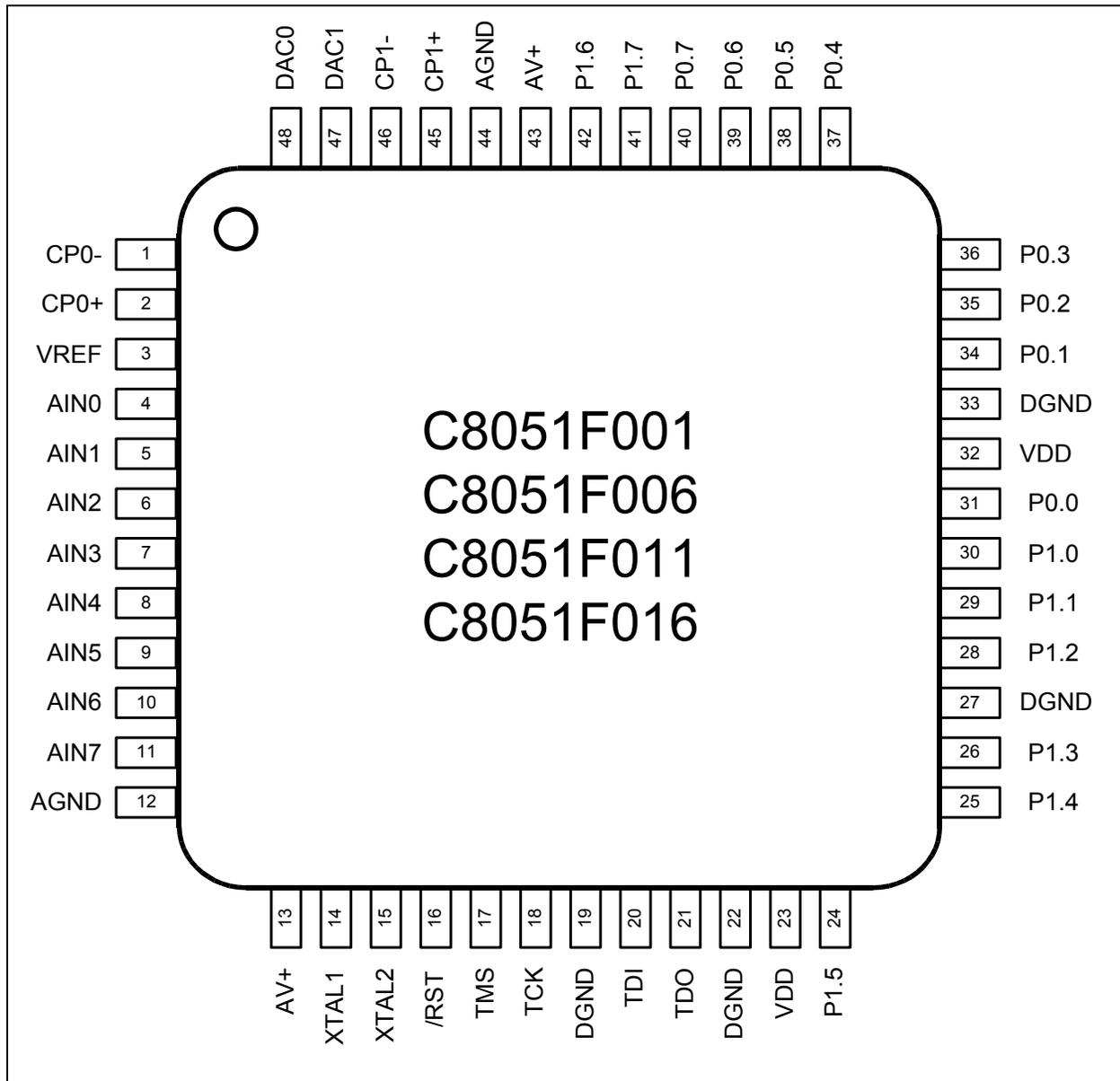
Figure 4.4. TQFP-48 Package Drawing
