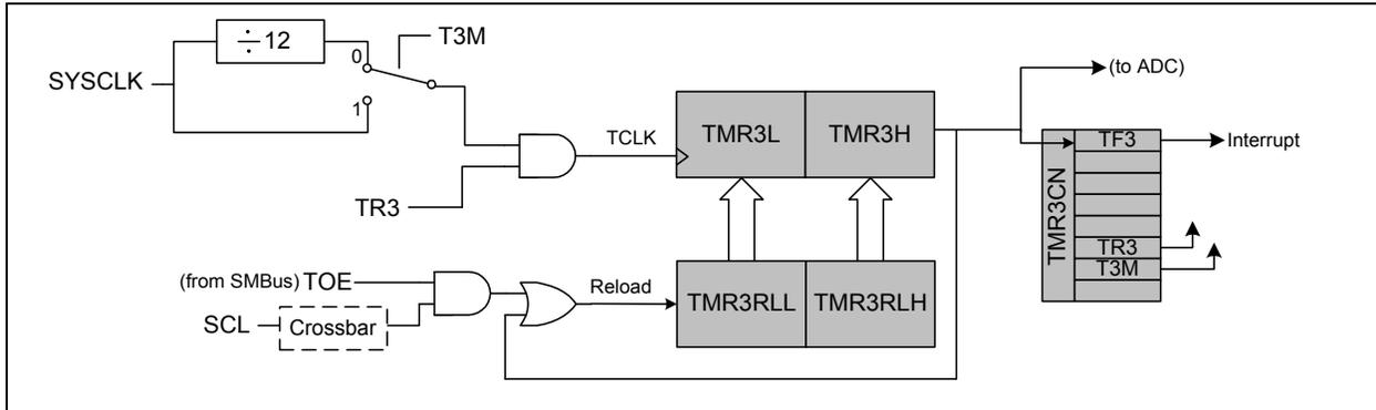
**Figure 19.20. TMR3CN: Timer 3 Control Register**
