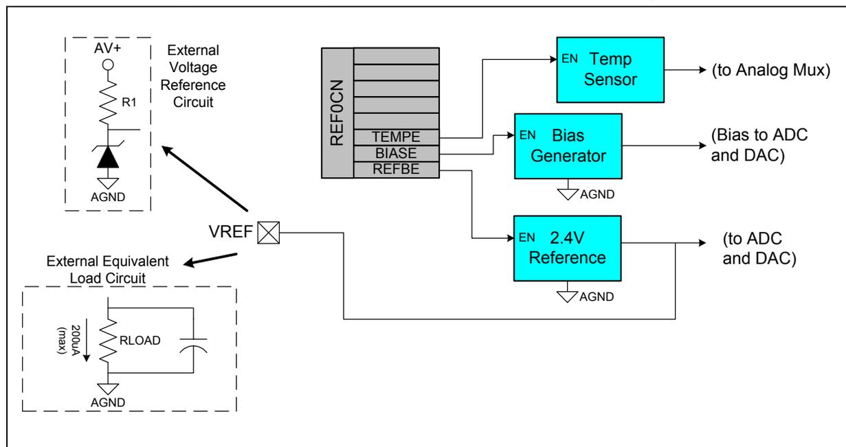
**Figure 9.2. REF0CN: Reference Control Register**
