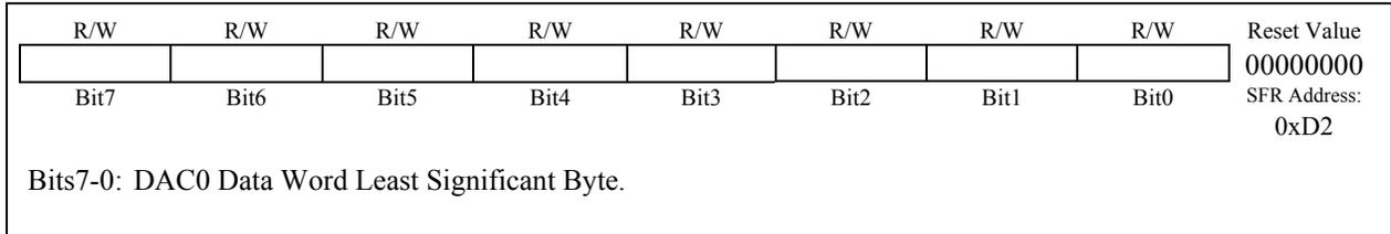
**Figure 7.4. DAC0CN: DAC0 Control Register**
