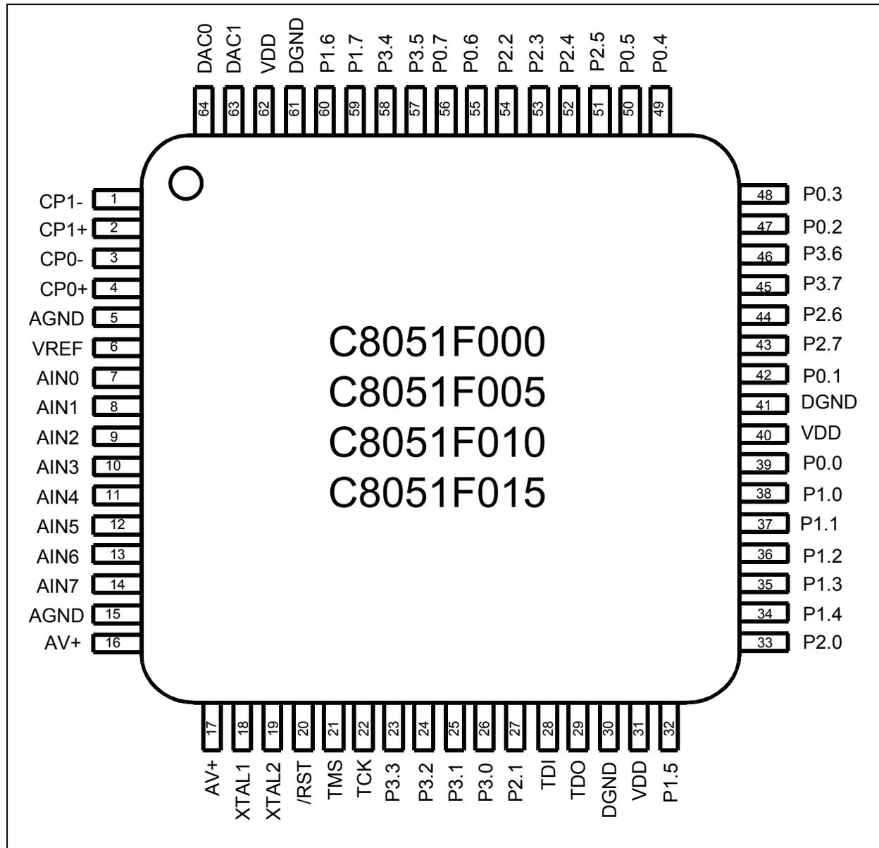
Figure 4.2. TQFP-64 Package Drawing
