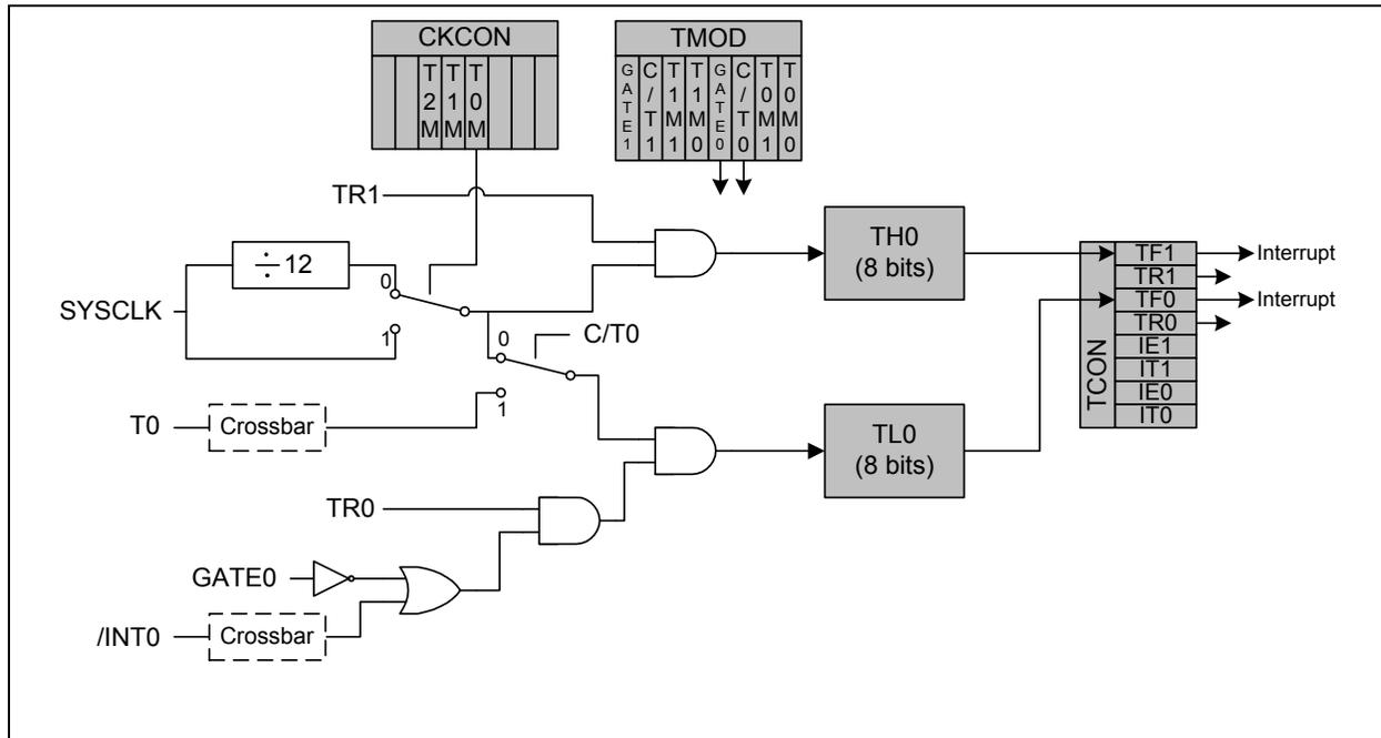
**Figure 19.4. TCON: Timer Control Register**
