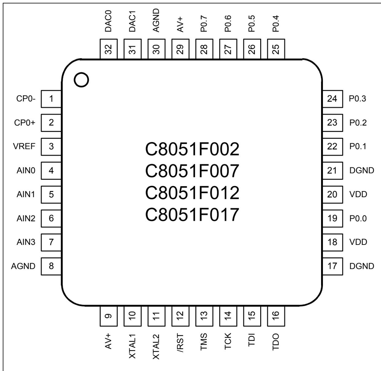
Figure 4.6. LQFP-32 Package Drawing
