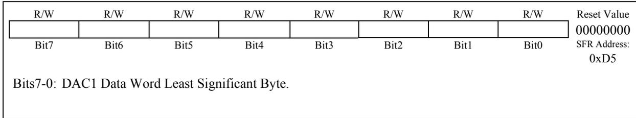
**Figure 7.7. DAC1CN: DAC1 Control Register**
