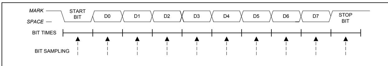
The baud rate generated in Mode 1 is a function of timer overflow. The UART can use Timer 1 operating in *8-bit Counter/Timer with Auto-Reload Mode*, or Timer 2 operating in *Baud Rate Generator Mode* to generate the baud rate (note that the TX and RX clock sources are selected separately). On each timer overflow event (a rollover from all ones (0xFF for Timer 1, 0xFFFF for Timer 2) to zero), a clock is sent to the baud rate logic.
