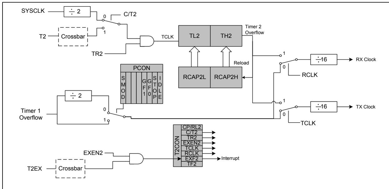
**Figure 19.14. T2CON: Timer 2 Control Register**
