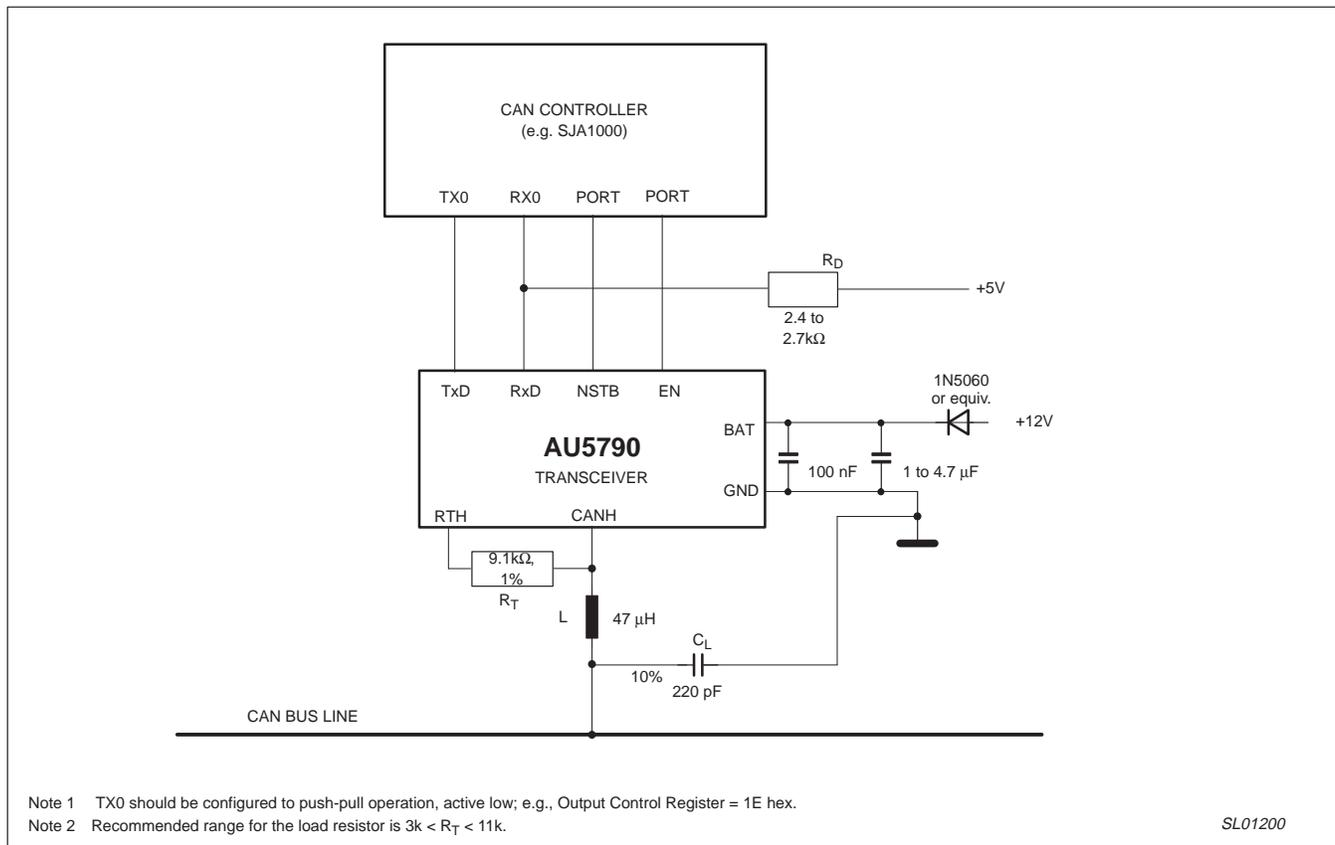
Figure 4. Application circuit example for the AU5790
