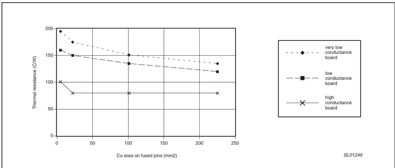
Figure 5. SO-8 Thermal Resistance vs. PCB Configuration, Note 1, 2, 3
