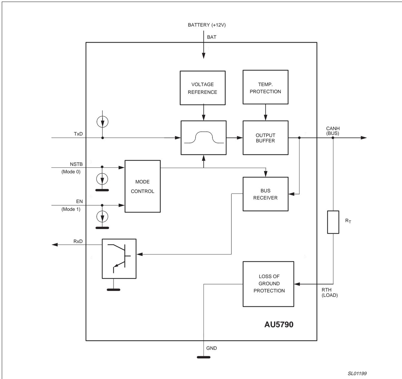
Figure 1. Block Diagram
