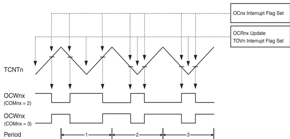
The Timer/Counter Overflow Flag (TOV1) is set each time the counter reaches BOTTOM. The Interrupt Flag can be used to generate an interrupt each time the counter reaches the BOTTOM value.
