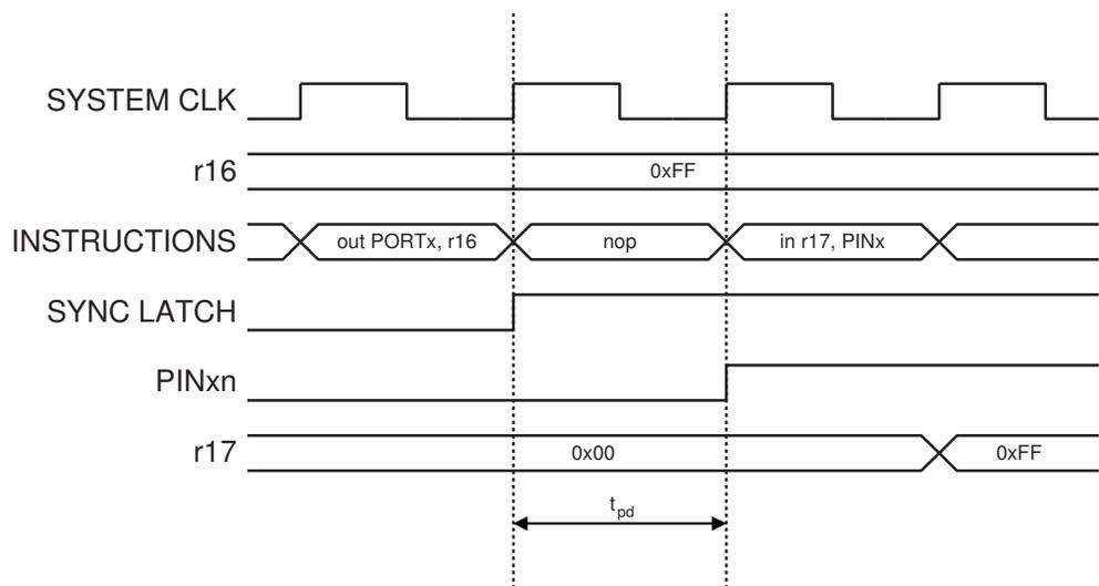
The following code example shows how to set port B pins 0 and 1 high, 2 and 3 low, and define the port pins from 4 to 5 as input with a pull-up assigned to port pin 4. The resulting pin values are read back again, but as previously discussed, a *nop* instruction is included to be able to read back the value recently assigned to some of the pins.
