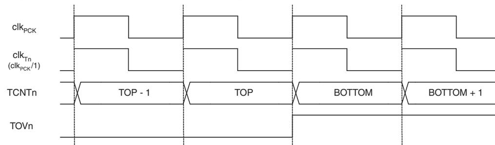
**Figure 16-15.** Timer/Counter Timing Diagram, with Prescaler ( $f_{clkT1}/8$ )
