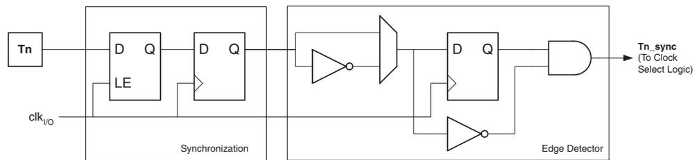
The synchronization and edge detector logic introduces a delay of 2.5 to 3.5 system clock cycles from an edge has been applied to the T0 pin to the counter is updated.
