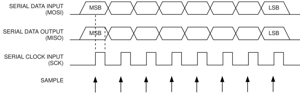
**Figure 23-7.** Serial Programming Timing
