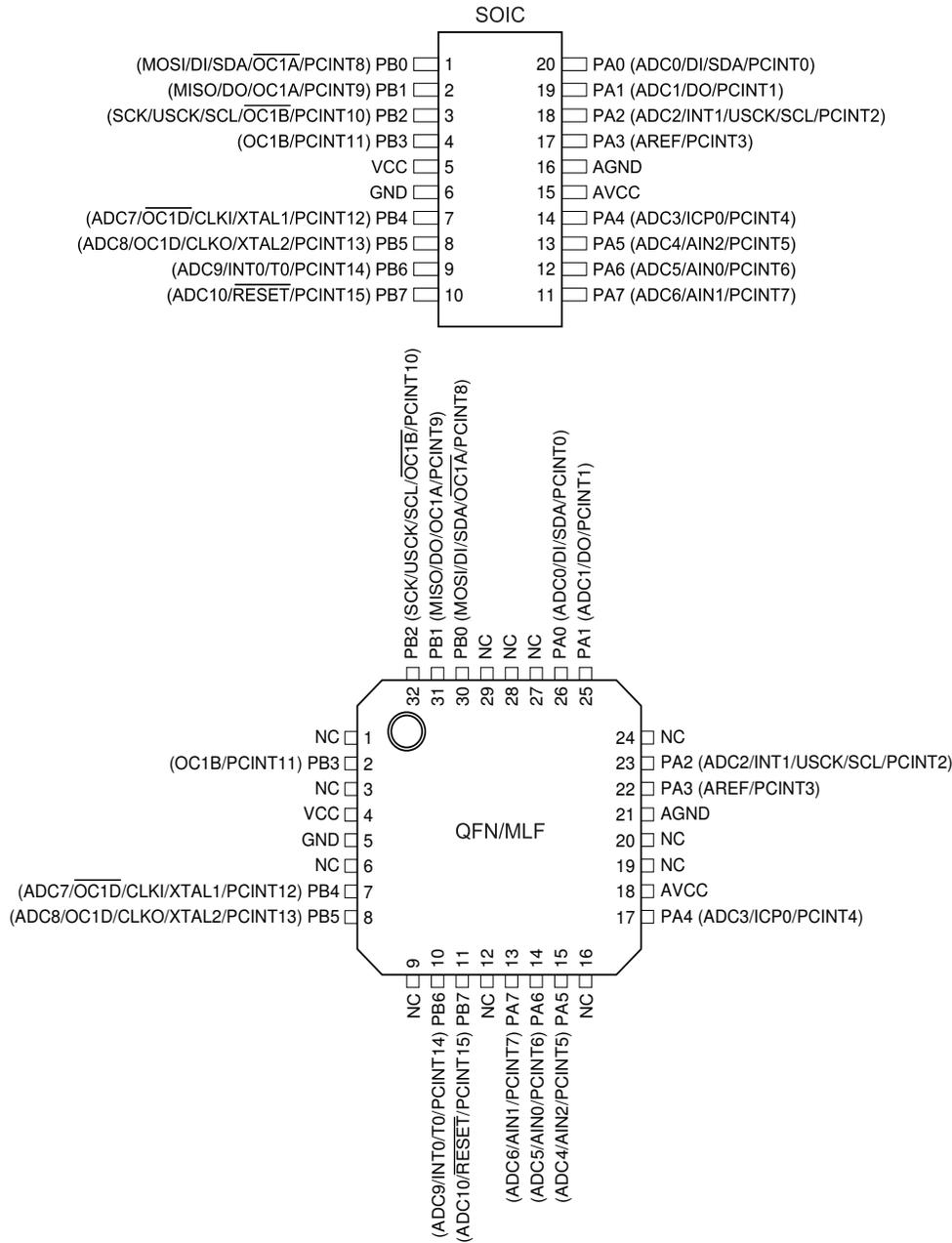
Note: The large center pad underneath the QFN/MLF package should be soldered to ground on the board to ensure good mechanical stability.
