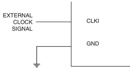
When this clock source is selected, start-up times are determined by the SUT Fuses as shown in [Table 7-3](#).
