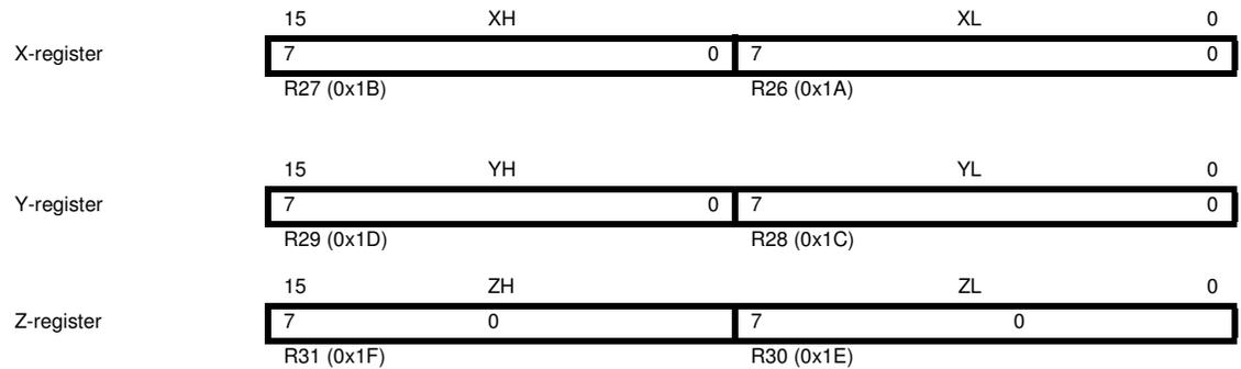
In the different addressing modes these address registers have functions as fixed displacement, automatic increment, and automatic decrement (see the instruction set reference for details).
