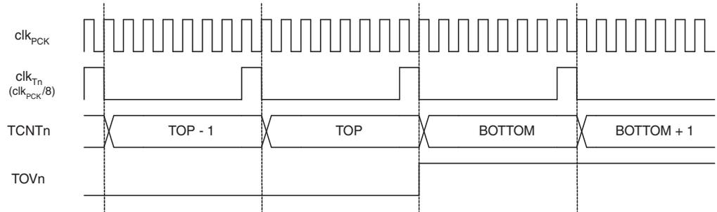
**Figure 16-16.** Timer/Counter Timing Diagram, Setting of OCF1x, with Prescaler ( $f_{clkT1}/8$ )
