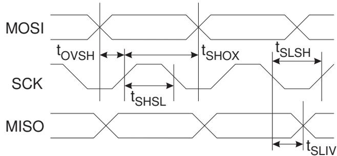
**Table 23-7.** Serial Programming Characteristics,  $T_A = -40^\circ\text{C}$  to  $125^\circ\text{C}$ ,  $V_{CC} = 2.7 - 5.5\text{V}$  (Unless Otherwise Noted)
