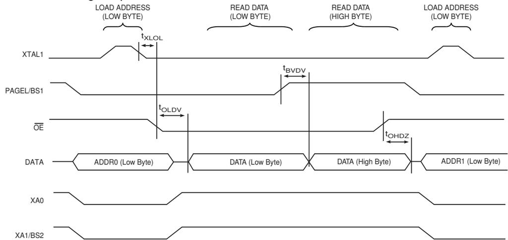
Note: 1. The timing requirements shown in Figure 23-3 (i.e.,  $t_{DVXH}$ ,  $t_{XHXL}$ , and  $t_{XLDX}$ ) also apply to reading operation.
