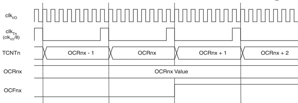
shows the setting of OCF0A and the clearing of TCNT0 in CTC mode.
