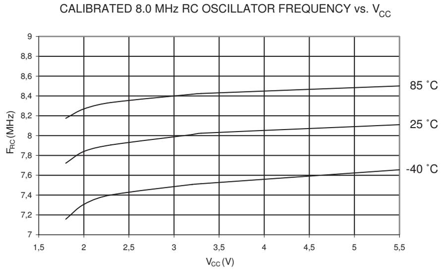
**Figure 24-32.** Calibrated 8.0 MHz RC Oscillator Frequency vs. Temperature
