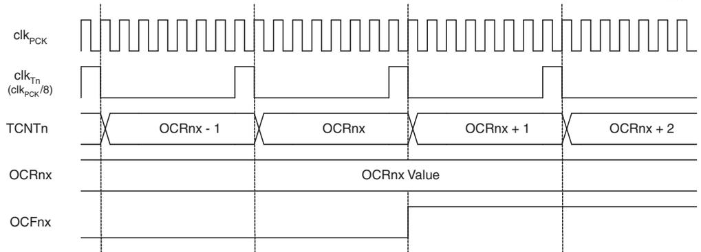
**Figure 16-17.** Timer/Counter Timing Diagram, with Prescaler ( $f_{clkT1}/8$ )
