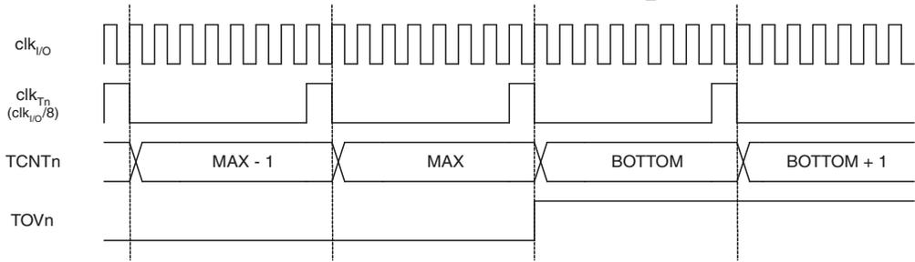
Figure 14-7 shows the setting of OCF0A and OCF0B in Normal mode.
