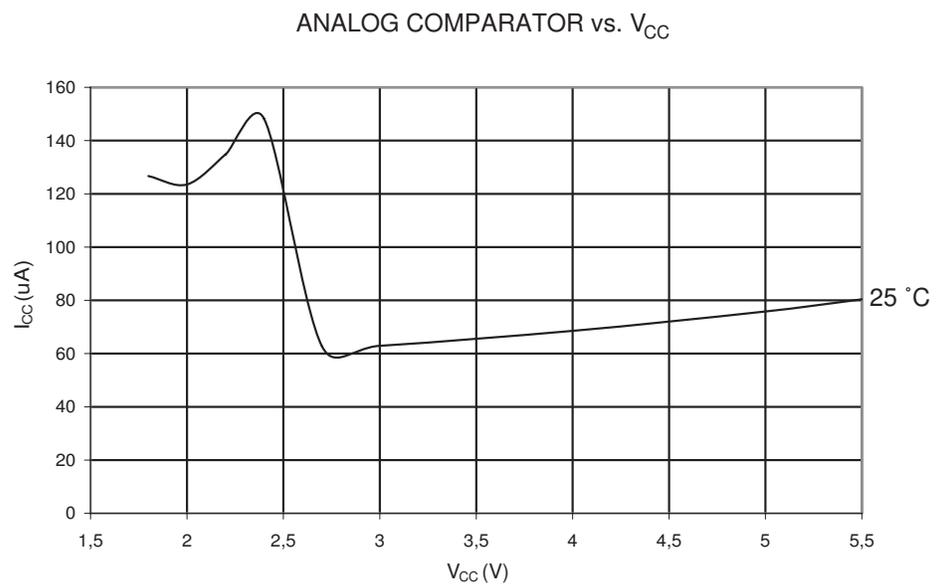
**Figure 24-37.** Brownout Detector Current vs.  $V_{CC}$
