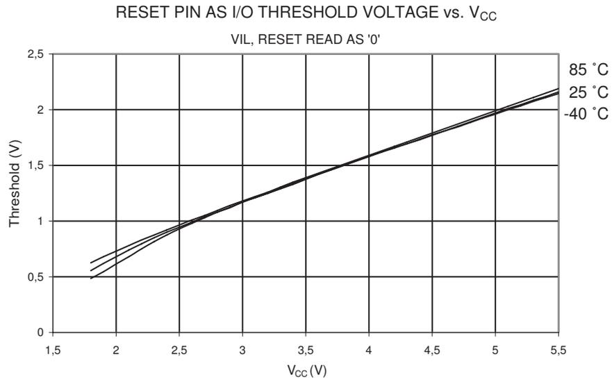
**Figure 24-26.** Reset Pin input Hysteresis vs.  $V_{CC}$
