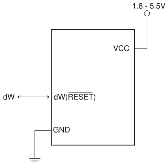
Figure 20-1 shows the schematic of a target MCU, with debugWIRE enabled, and the emulator connector. The system clock is not affected by debugWIRE and will always be the clock source selected by the CKSEL Fuses.
