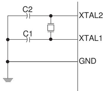
The Oscillator can operate in three different modes, each optimized for a specific frequency range. The operating mode is selected by the fuses CKSEL3..1 as shown in [Table 7-10](#).
