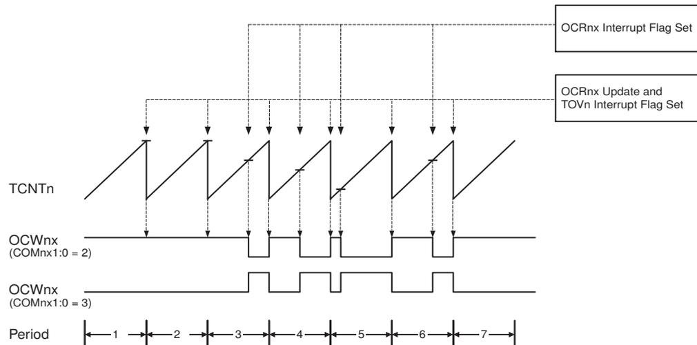
The Timer/Counter Overflow Flag (TOV1) is set each time the counter reaches TOP. If the interrupt is enabled, the interrupt handler routine can be used for updating the compare value.
