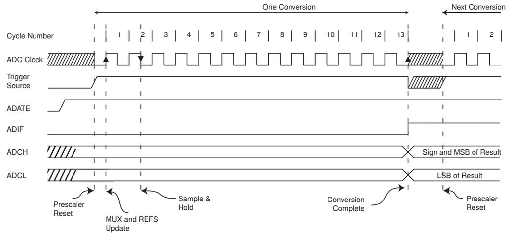
**Figure 19-7.** ADC Timing Diagram, Free Running Conversion
