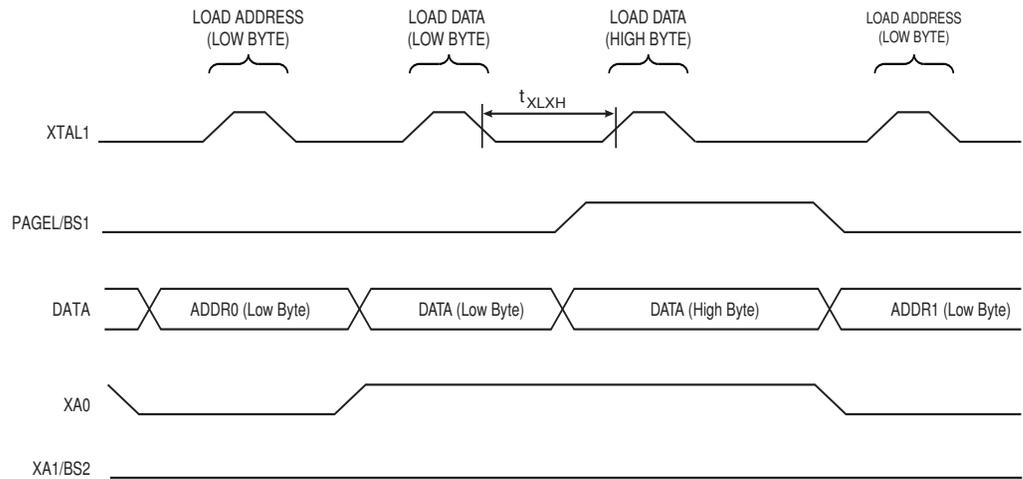
Note: 1. The timing requirements shown in Figure 23-3 (i.e.,  $t_{DVXH}$ ,  $t_{XHL}$ , and  $t_{XLDX}$ ) also apply to loading operation.
