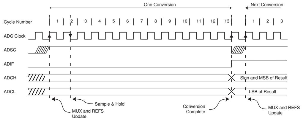
**Figure 19-6.** ADC Timing Diagram, Auto Triggered Conversion
