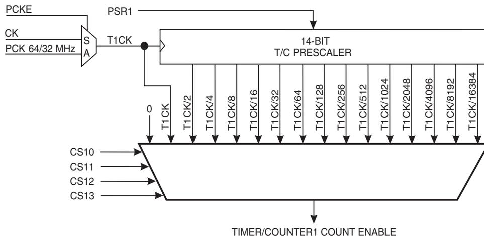
In the asynchronous clocking mode the clock selections are from PCK to PCK/16384 and stop, and in the synchronous clocking mode the clock selections are from CK to CK/16384 and stop. The clock options are described in Table 15-1 on page 91 and the Timer/Counter1 Control Register, TCCR1B.
