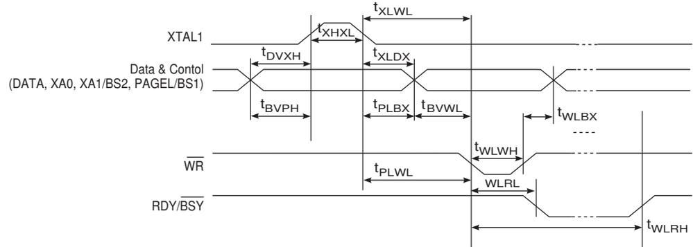
**Figure 23-4.** Parallel Programming Timing, Loading Sequence with Timing Requirements<sup>(1)</sup>
