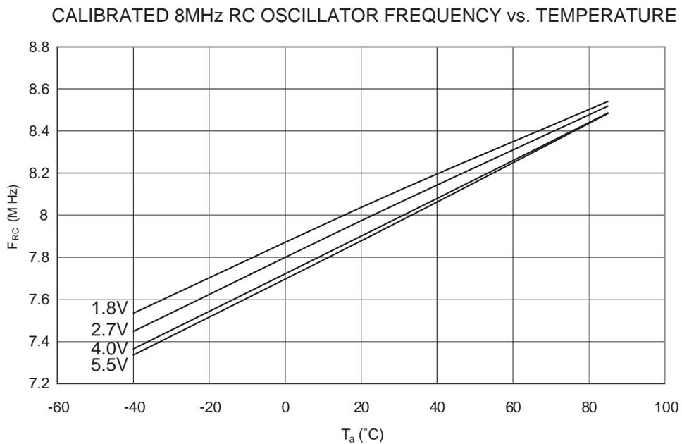
**Figure 27-56.** Calibrated 8 MHz RC Oscillator Frequency vs.  $V_{CC}$
