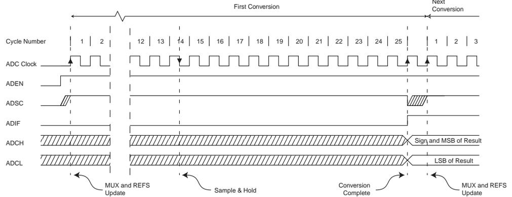
**Figure 21-5.** ADC Timing Diagram, Single Conversion
