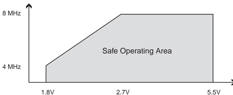
Figure 26-2. Maximum Frequency vs.  $V_{CC}$ , ATmega165P
