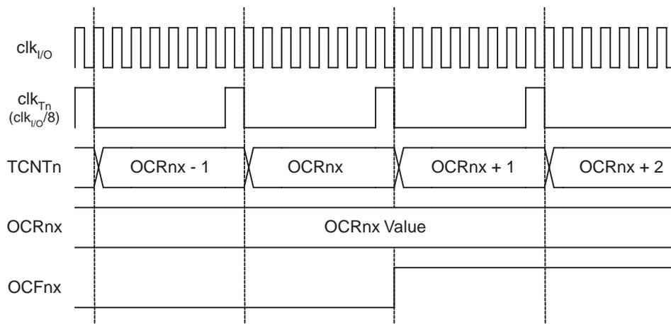
[Figure 14-12](#) shows the count sequence close to TOP in various modes. When using phase and frequency correct PWM mode the OCR1x Register is updated at BOTTOM. The timing diagrams
