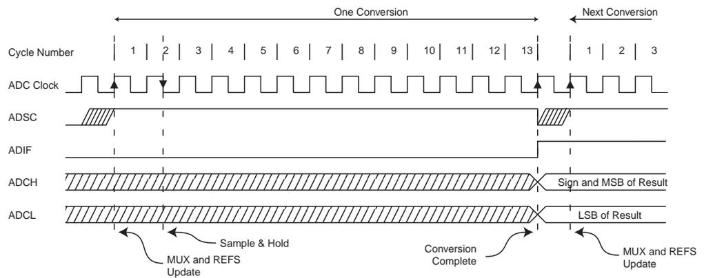
**Figure 21-6.** ADC Timing Diagram, Auto Triggerred Conversion
