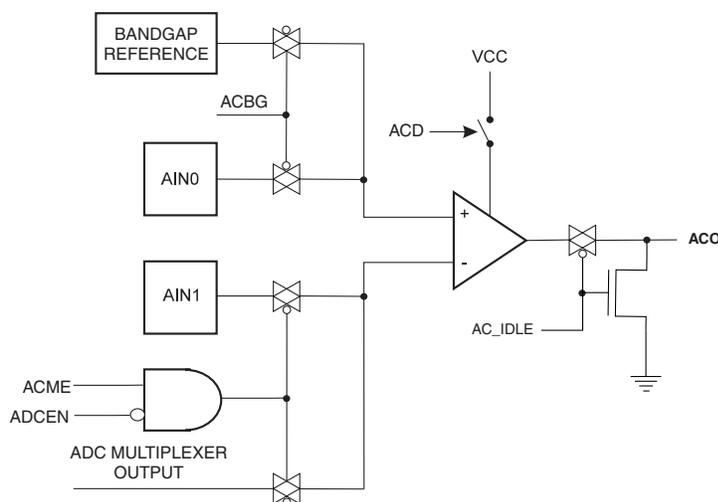
**Figure 23-8.** General Boundary-scan cell Used for Signals for Comparator and ADC
