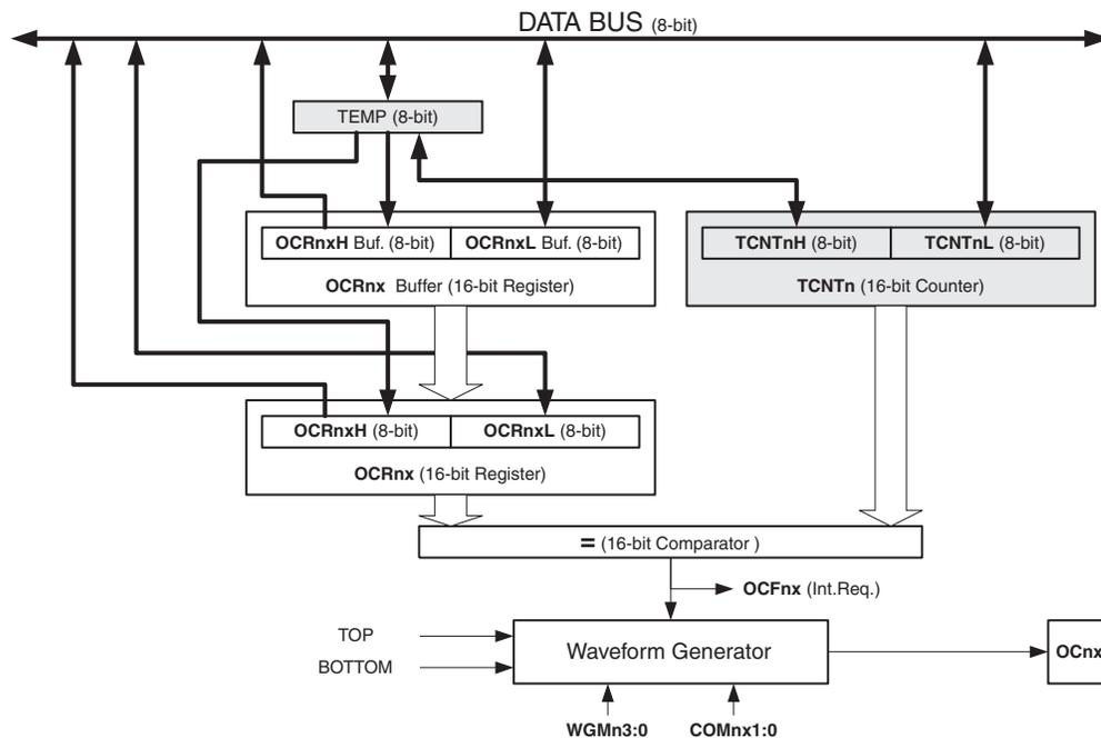
The OCR1x Register is double buffered when using any of the twelve *Pulse Width Modulation* (PWM) modes. For the Normal and *Clear Timer on Compare* (CTC) modes of operation, the double buffering is disabled. The double buffering synchronizes the update of the OCR1x Compare Register to either TOP or BOTTOM of the counting sequence. The synchronization
