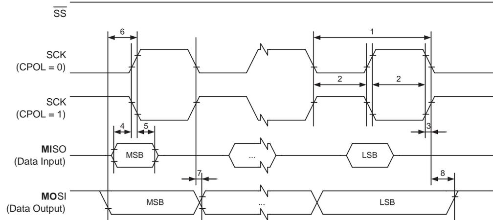
**Figure 26-8. SPI Interface Timing Requirements (Slave Mode)**
