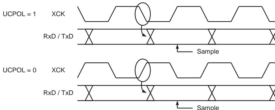
The UCPOLn bit in UCSRNc selects which XCK clock edge is used for data sampling and which is used for data change. As [Figure 18-3](#) shows, when UCPOLn is zero the data will be changed at rising XCK edge and sampled at falling XCK edge. If UCPOLn is set, the data will be changed at falling XCK edge and sampled at rising XCK edge.
