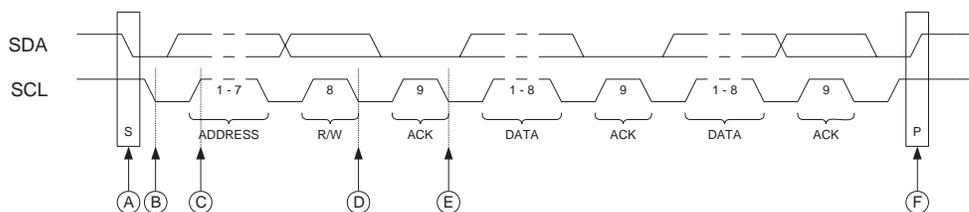
Referring to the timing diagram (Figure 19-5.), a bus transfer involves the following steps:
