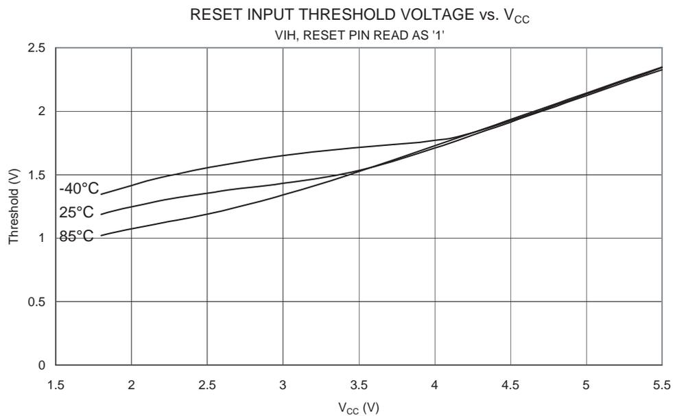
Figure 27-46. Reset Input Pin Hysteresis vs.  $V_{CC}$
