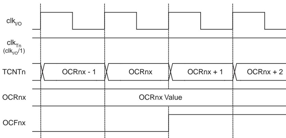
[Figure 14-11](#) shows the same timing data, but with the prescaler enabled.
