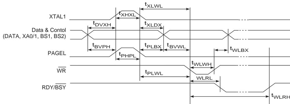
**Figure 26-5.** Parallel Programming Timing, Loading Sequence with Timing Requirements<sup>(1)</sup>
