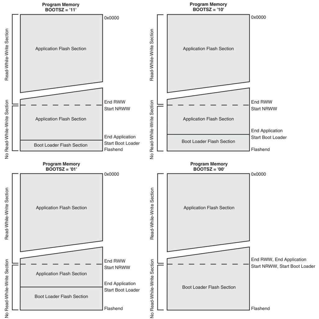
Note: 1. The parameters in the figure above are given in [Table 24-6 on page 266](#).
