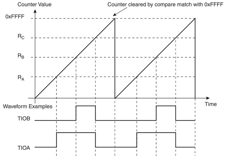
**Figure 32-8.** WAVSEL= 00 with trigger
