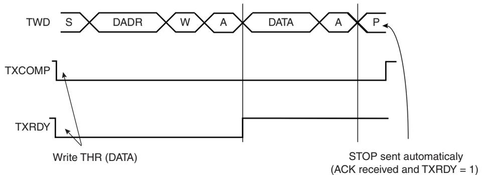
**Figure 29-6.** Master Write with Multiple Data Byte
