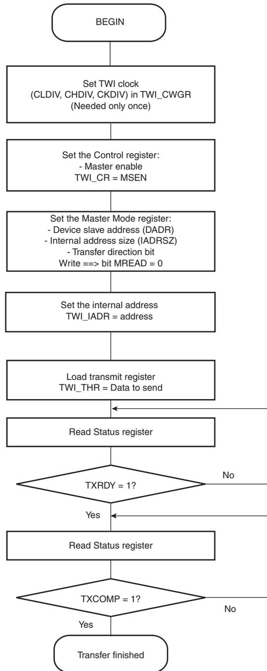
**Figure 29-15. TWI Write Operation with Multiple Data Bytes with or without Internal Address**
