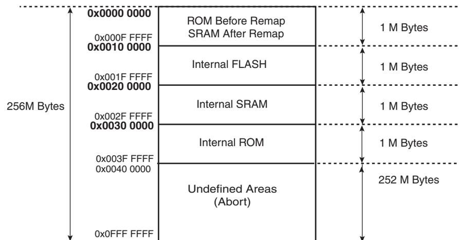
**Figure 8-3.** Internal Memory Mapping with GPNVM Bit 2 = 1
