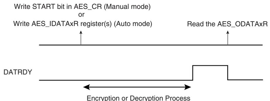
If the user does not want to read the output data registers between each encryption/decryption, the DATRDY flag will not be cleared. If the DATRDY flag is not cleared, the user cannot know the end of the following encryptions/decryptions.
