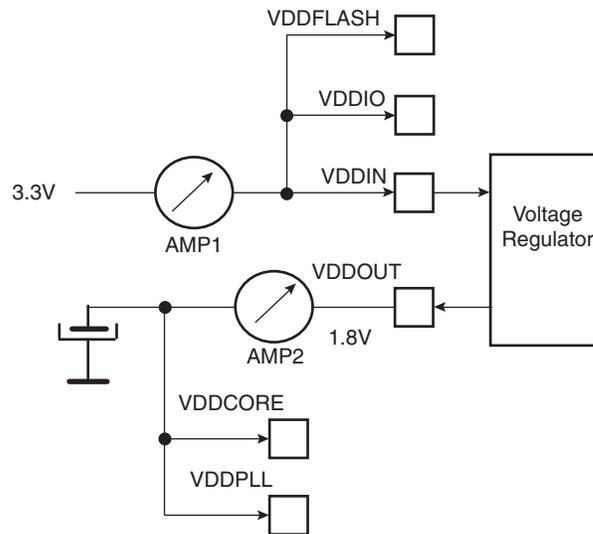
These figures represent the power consumption typically measured on the power supplies..
