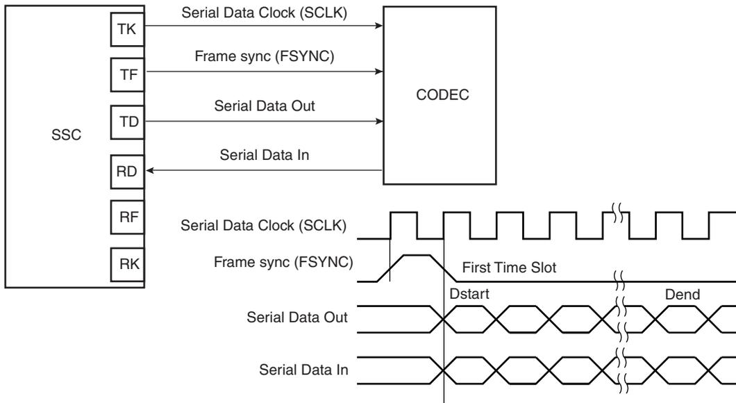
**Figure 30-19.** Time Slot Application Block Diagram
