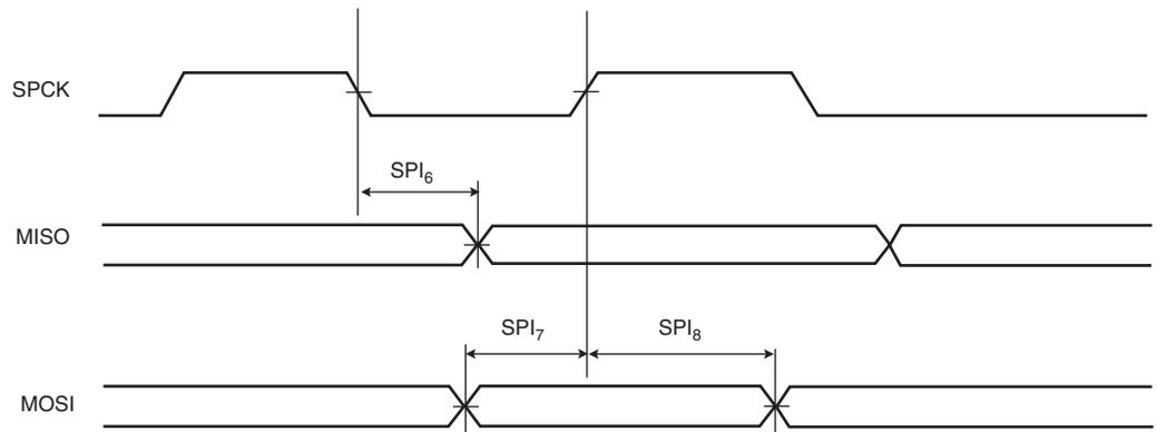
**Figure 40-7.** SPI Slave mode with (CPOL = NCPHA = 0) or (CPOL= NCPHA= 1)
