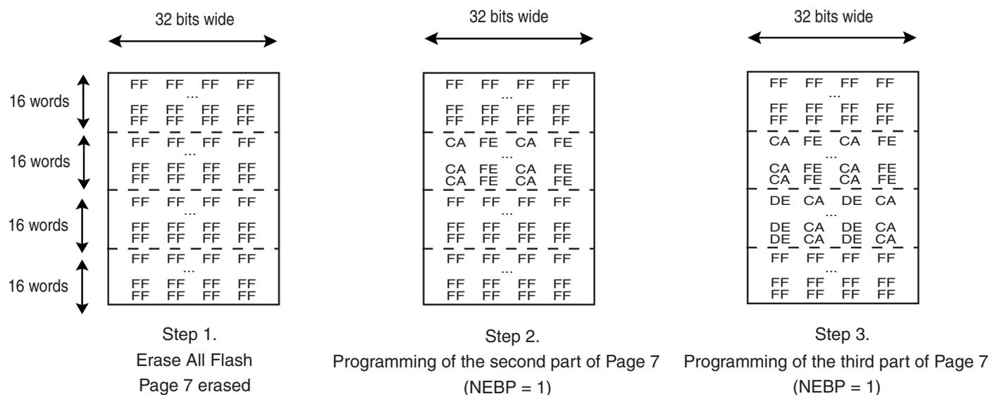
After programming, the page (the whole lock region) can be locked to prevent miscellaneous write or erase sequences. The lock bit can be automatically set after page programming using WPL.
