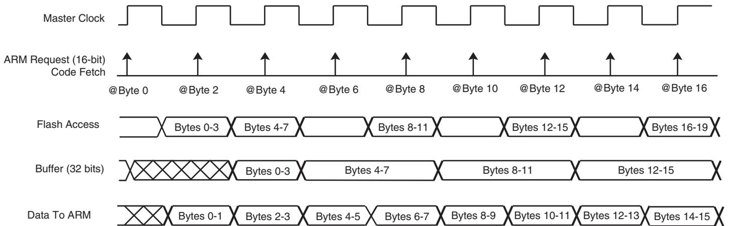
Note: When FWS is equal to 0, all accesses are performed in a single-cycle access.
