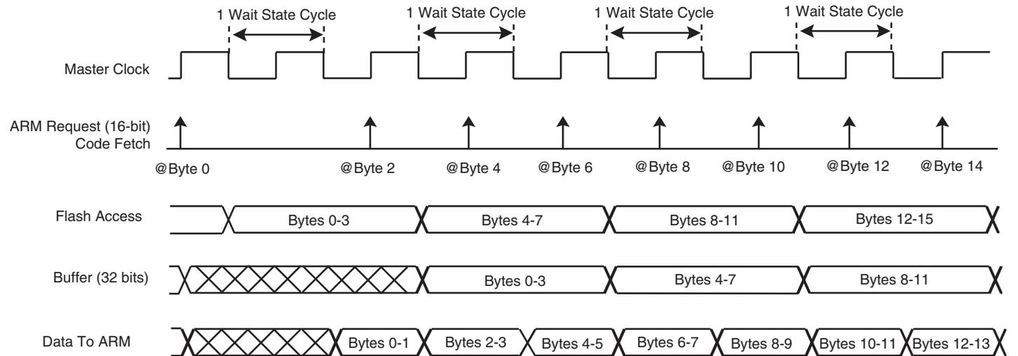
Note: When FWS is equal to 1, in case of sequential reads, all the accesses are performed in a single-cycle access (except for the first one).
