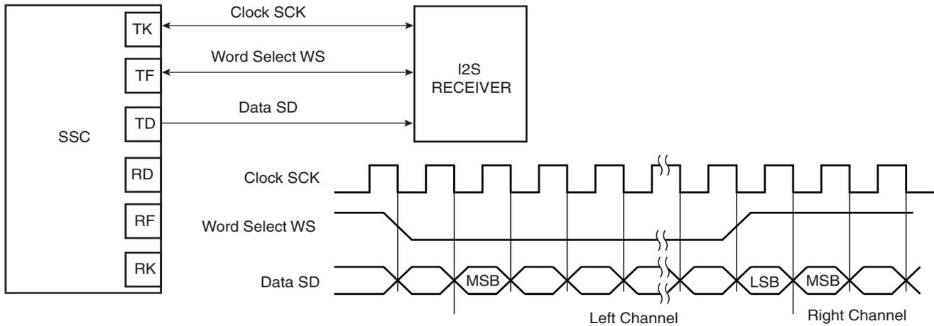
**Figure 30-18.** Codec Application Block Diagram
