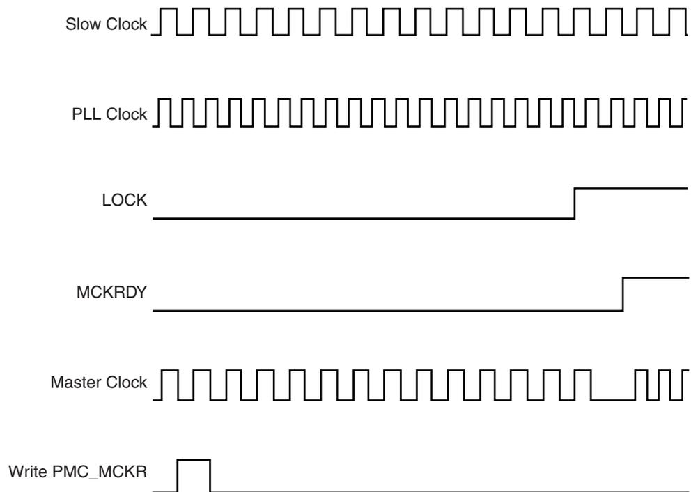
**Figure 26-4.** Switch Master Clock from Main Clock to Slow Clock
