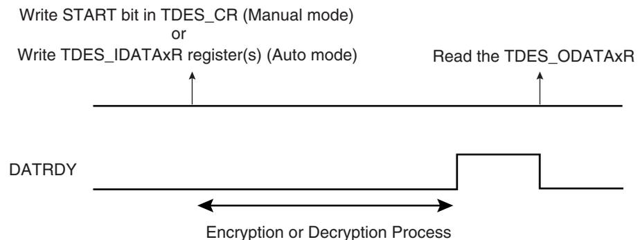
If the user does not want to read the output data registers between each encryption/decryption, the DATRDY flag will not be cleared. If the DATRDY flag is not cleared, the user will not be informed of the end of the encryptions/decryptions that follow.
