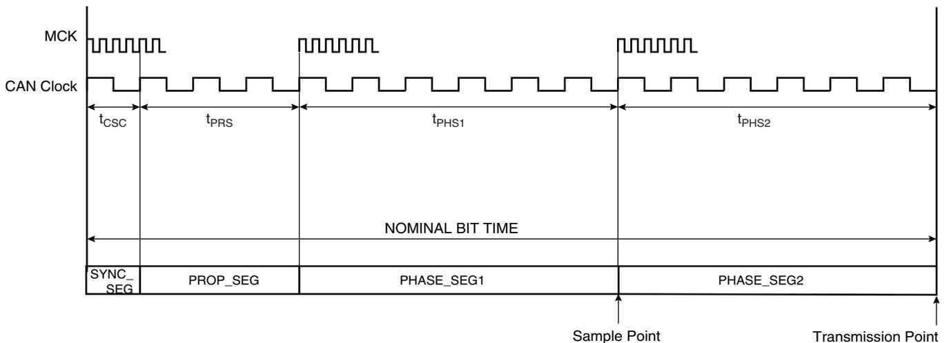
Example of bit timing determination for CAN baudrate of 500 Kbit/s:
