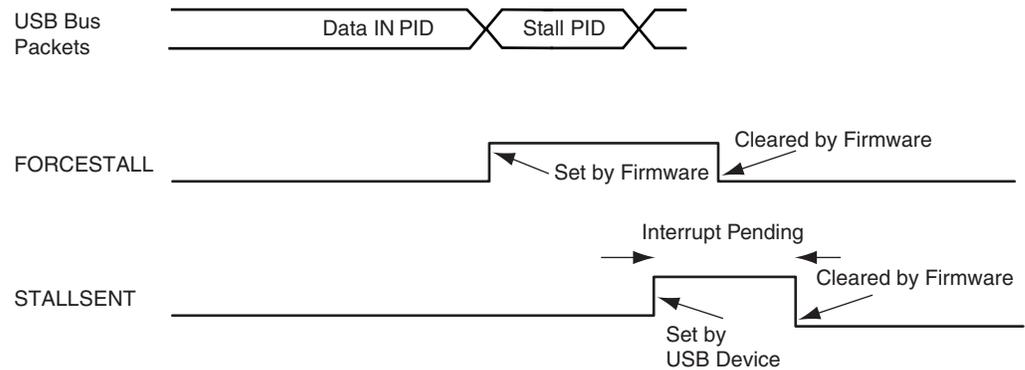
**Figure 34-13.** Stall Handshake (Data OUT Transfer)
