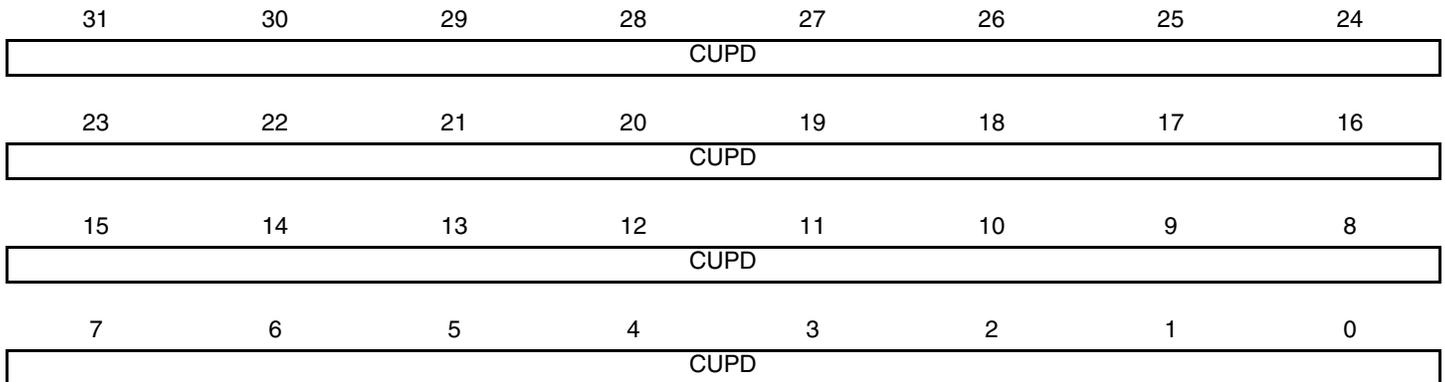
This register acts as a double buffer for the period or the duty cycle. This prevents an unexpected waveform when modifying the waveform period or duty-cycle.
