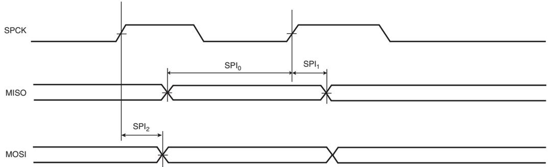
**Figure 40-5.** SPI Master mode with (CPOL=0 and NCPHA=1) or (CPOL=1 and NCPHA=0)
