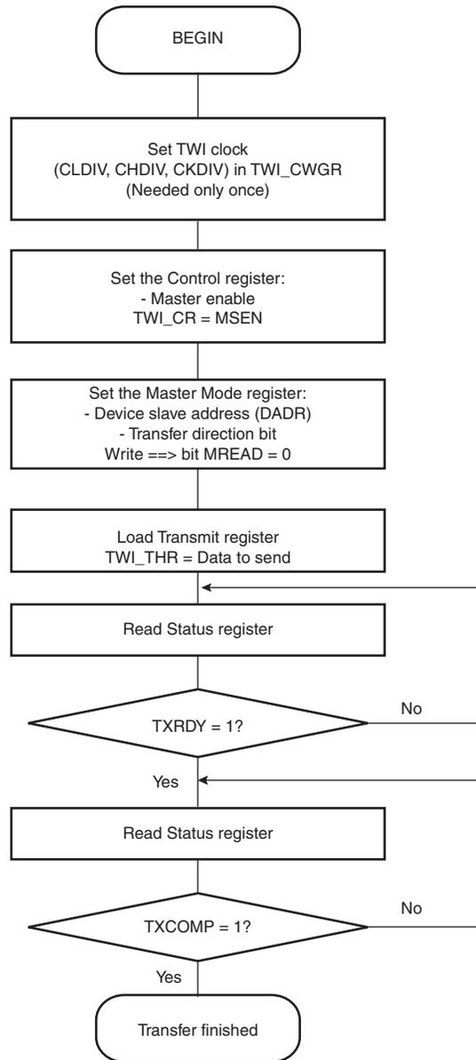
**Figure 29-14. TWI Write Operation with Single Data Byte and Internal Address**
