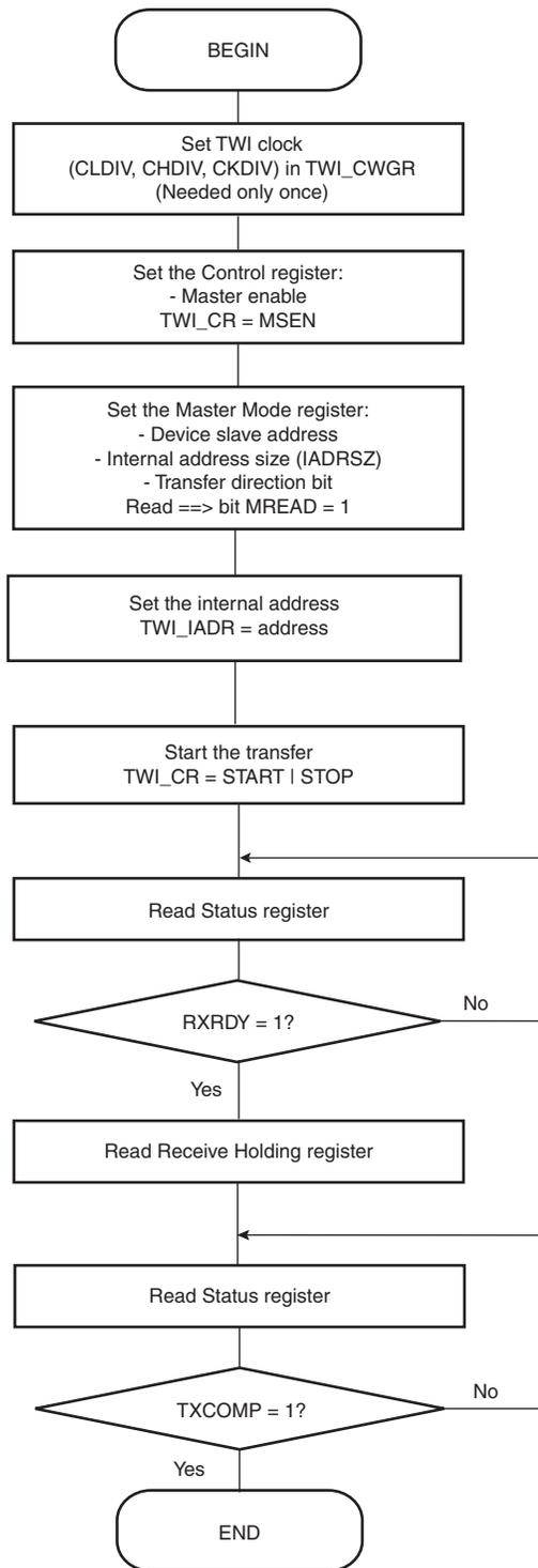
**Figure 29-18. TWI Read Operation with Multiple Data Bytes with or without Internal Address**
