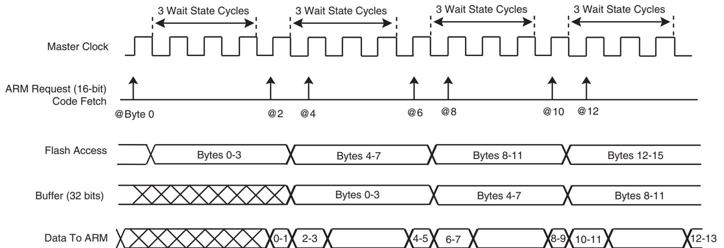
**Note:** When FWS is equal to 2 or 3, in case of sequential reads, the first access takes FWS cycles, the second access one cycle, the third access FWS cycles, the fourth access one cycle, etc.
