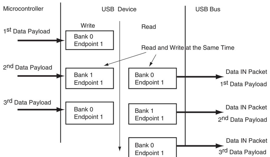
When using a ping-pong endpoint, the following procedures are required to perform Data IN transactions:
