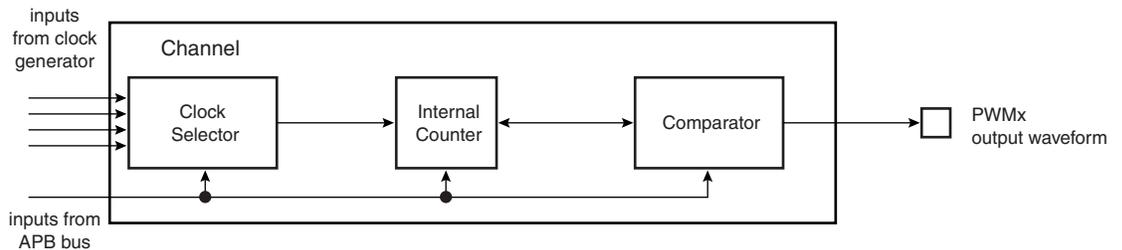
Each of the 4 channels is composed of three blocks:
