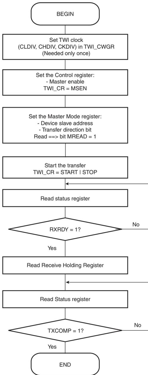
**Figure 29-17. TWI Read Operation with Single Data Byte and Internal Address**
