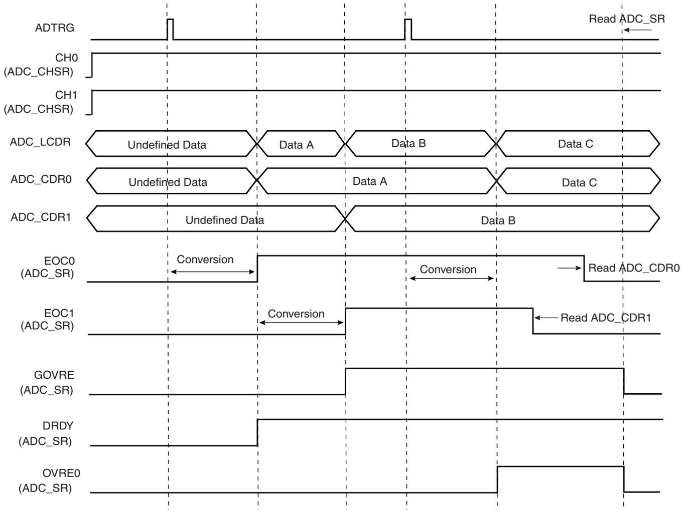
**Warning:** If the corresponding channel is disabled during a conversion or if it is disabled and then reenabled during a conversion, its associated data and its corresponding EOC and OVRE flags in ADC\_SR are unpredictable.
