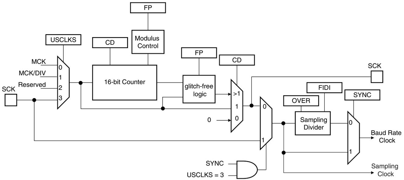
**31.6.1.4** *Baud Rate in Synchronous Mode*
