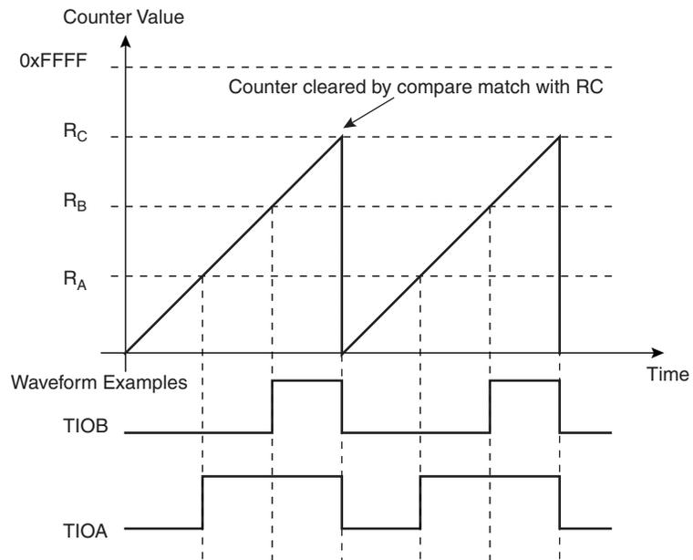
**Figure 32-10. WAVSEL = 10 With Trigger**
