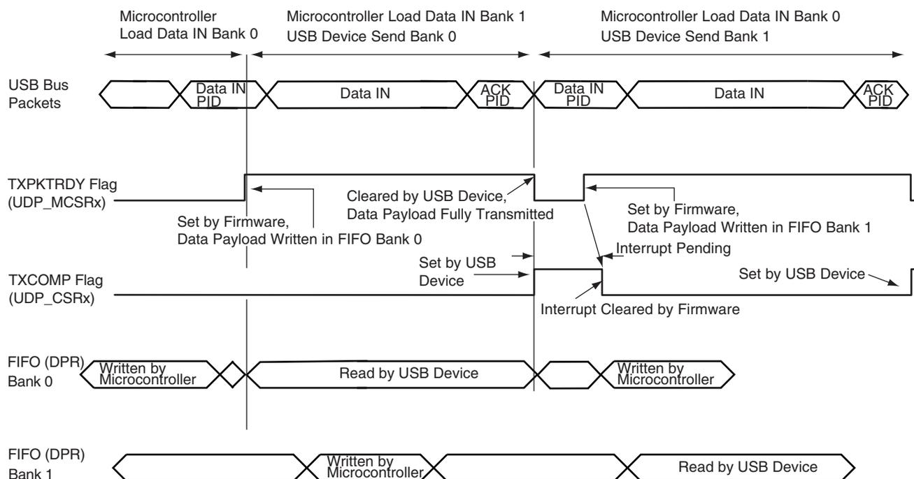
**Warning:** There is software critical path due to the fact that once the second bank is filled, the driver has to wait for TX\_COMP to set TX\_PKTRDY. If the delay between receiving TX\_COMP is set and TX\_PKTRDY is set is too long, some Data IN packets may be NACKed, reducing the bandwidth.
