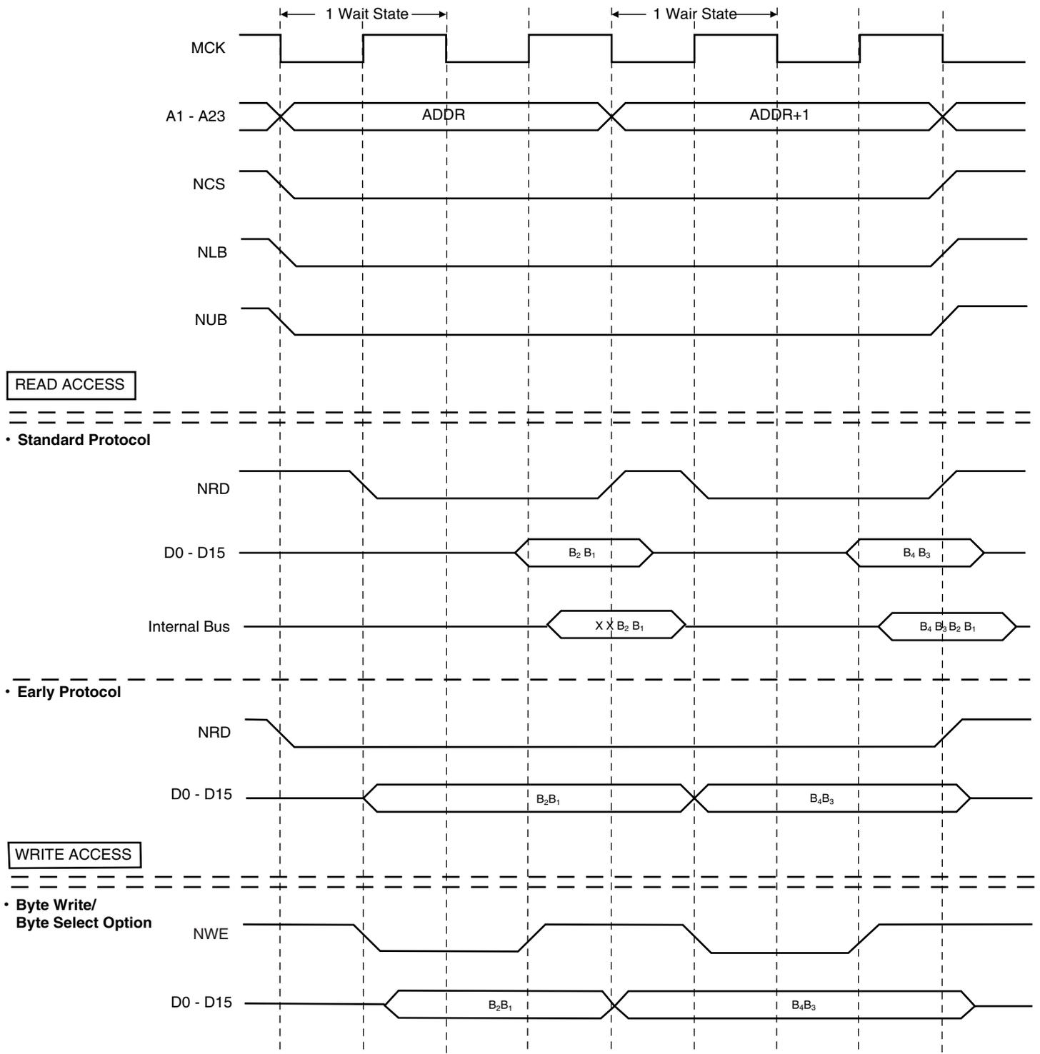
**Figure 28.** 1 Wait State, 16-bit Bus Width, Half-word Transfer
