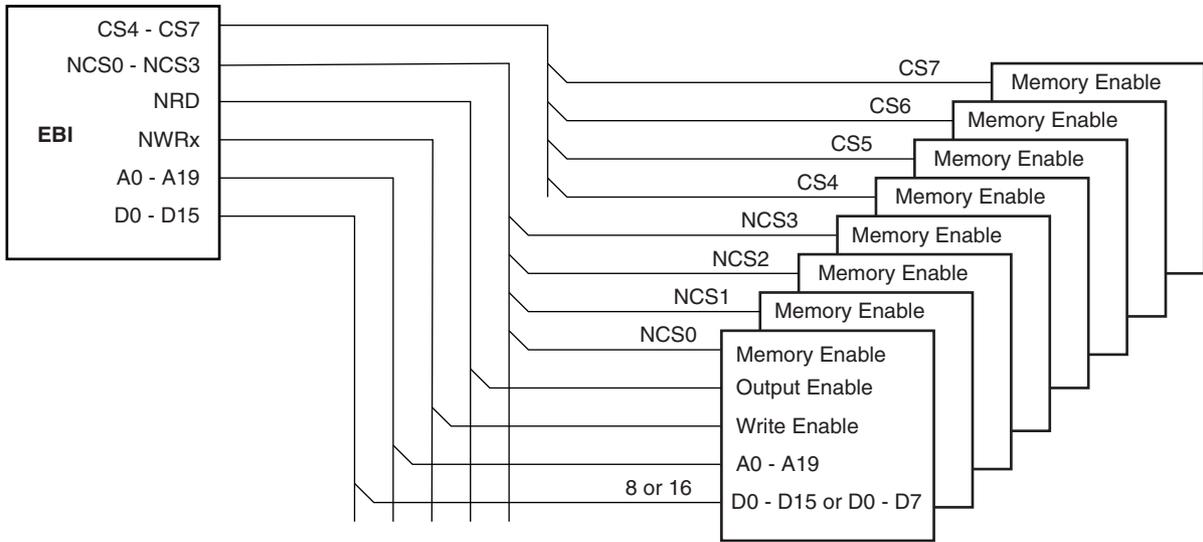
Note: For eight external devices, the maximum address space per device is 1M byte.
