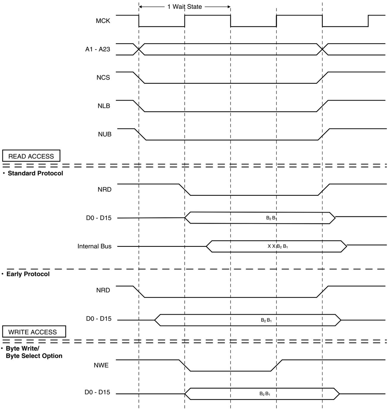
**Figure 29. 0 Wait States, 8-bit Bus Width, Word Transfer**
