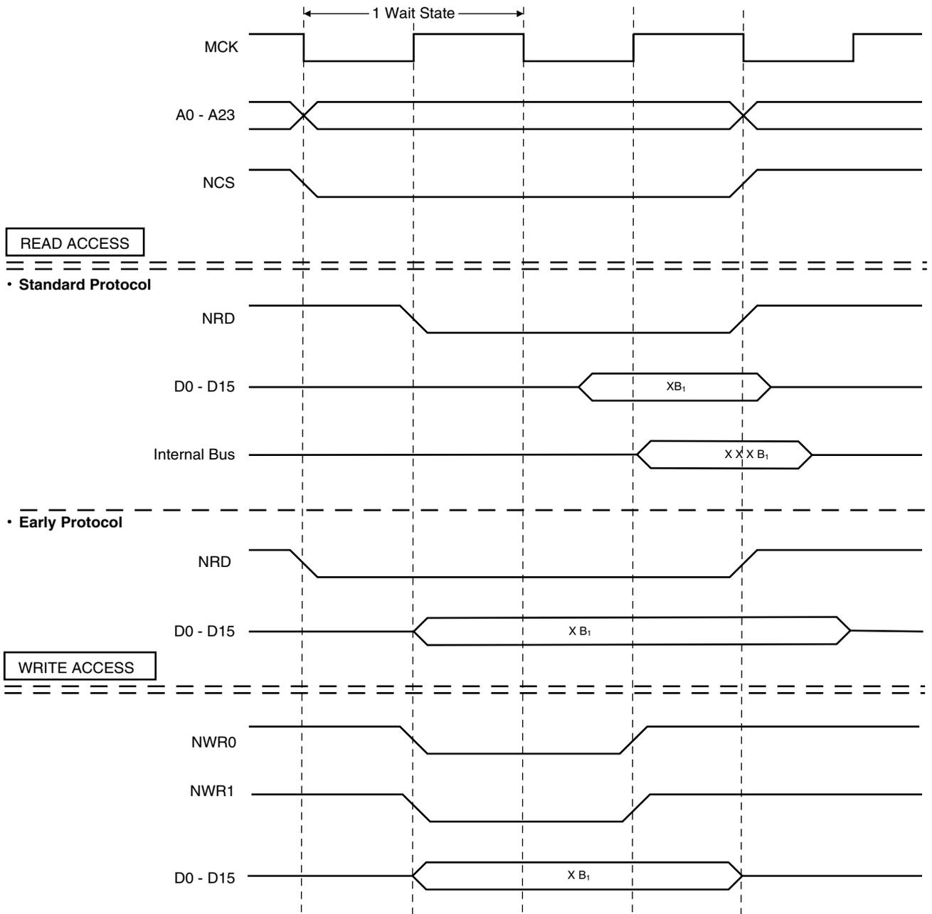
**Figure 32. 0 Wait States, 16-bit Bus Width, Byte Transfer**
