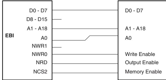
Figure 10 shows how to connect a 512K x 16-bit memory on NCS2.
