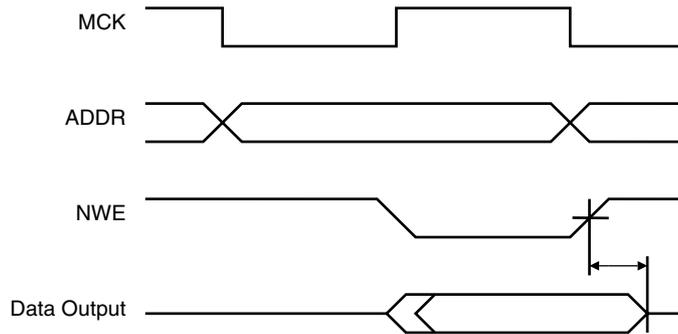
In early read protocol the data can remain valid longer than in standard read protocol due to the additional wait cycle which follows a write access.
