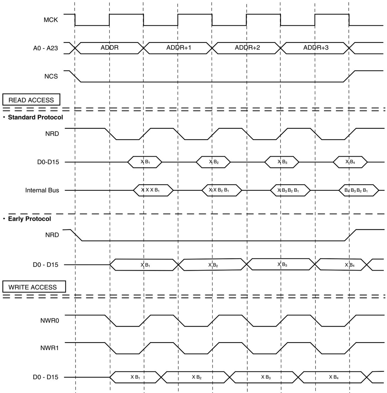
**Figure 30.** 1 Wait State, 8-bit Bus Width, Half-word Transfer
