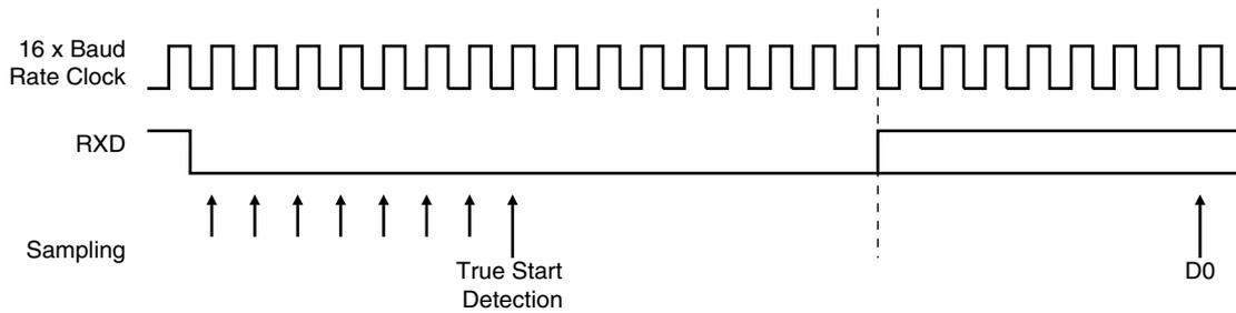
Figure 39. Asynchronous Mode: Character Reception
