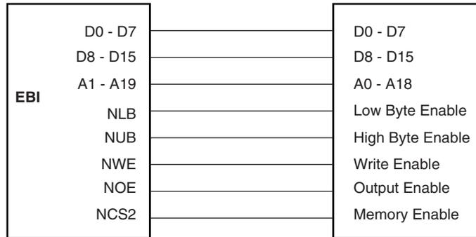
Figure 13 shows how to connect a 16-bit device without byte access (e.g. Flash) on NCS2.
