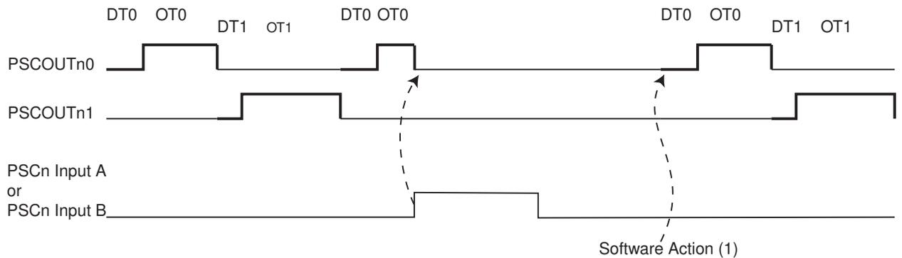
Note: 1. Software action is the setting of the PRUNn bit in PCTLn register.
