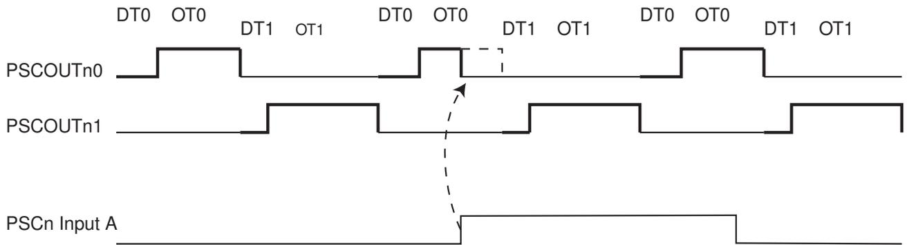
The output frequency is not modified by the occurrence of significant edge of retriggering input. Only the output is deactivated when significant edge on retriggering input occurs.
