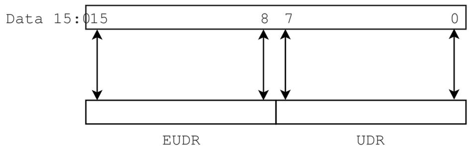
For 17 bit character the seventeenth bit is located in RxB8 or TxB8 register. In transmitter mode, the data should be written MSB first. The data transmission starts when the UDR register is written.
