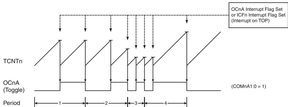
An interrupt can be generated at each time the counter value reaches the TOP value by either using the OCFnA or ICFn Flag according to the register used to define the TOP value. If the
