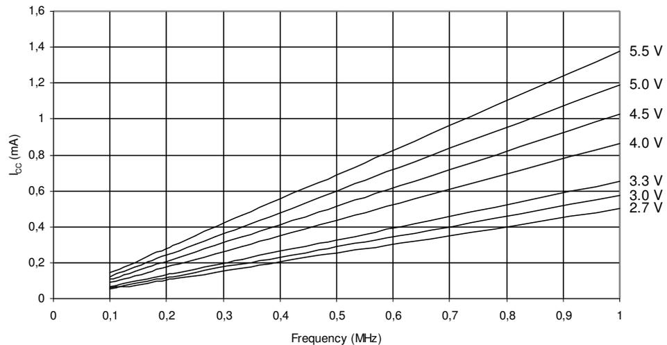
**Figure 27-2.** Active Supply Current vs. Frequency (1 - 24 MHz)
