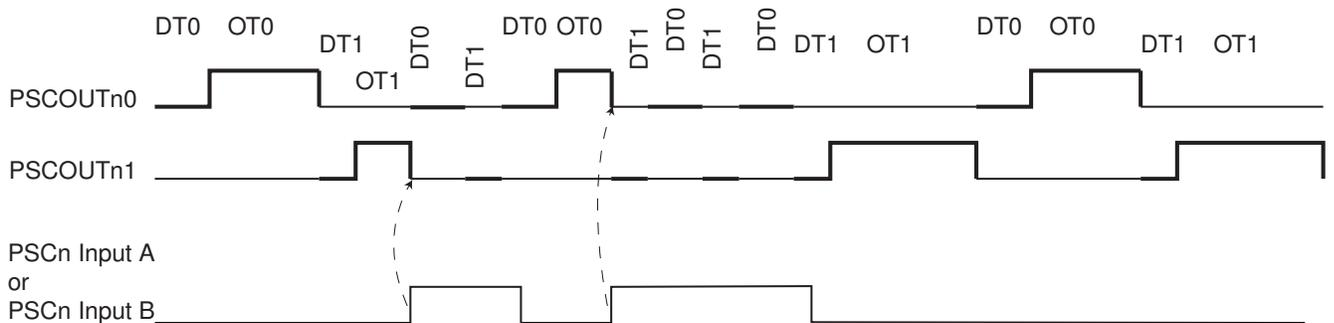
Used in Fault mode 5, PSCn Input A or PSCn Input B act indifferently on On-Time0/Dead-Time0 or on On-Time1/Dead-Time1.
