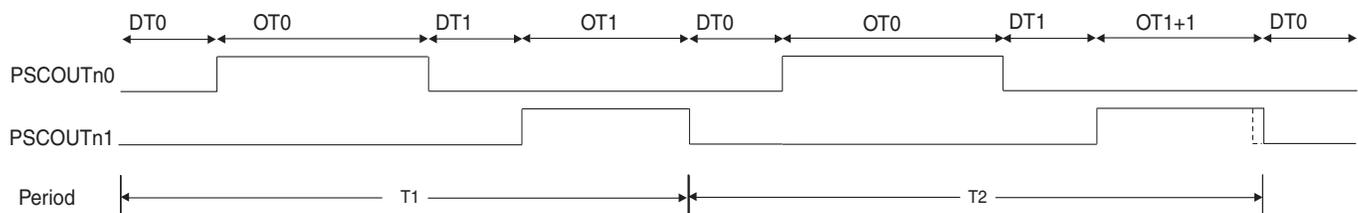
The supplementary step in counting to generate  $f_{b2}$  is added on the PSCn0 signal while needed in the frame according to the fractional divider. See [Table 49, "Distribution of fb2 in the modulated frame," on page 140](#).
