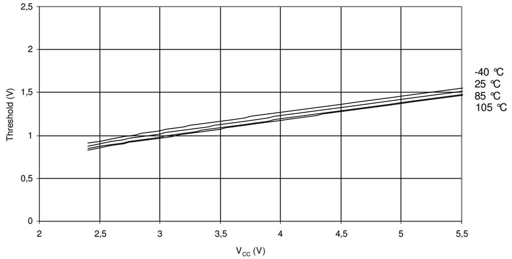
**Figure 27-22.** Reset Input Threshold Voltage vs.  $V_{CC}$  (VIH, Reset Pin Read As '1')
