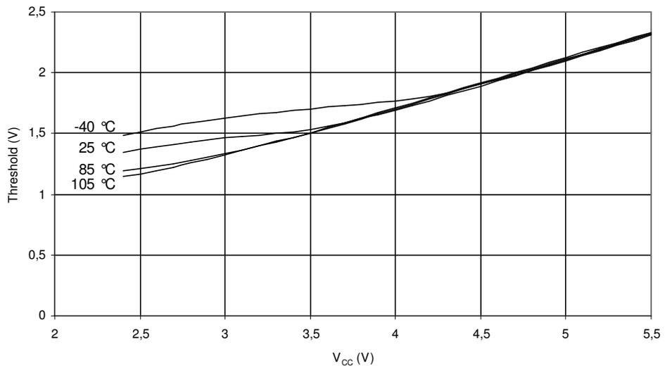
**Figure 27-23.** Reset Input Threshold Voltage vs.  $V_{CC}$  (VIL, Reset Pin Read As '0')
