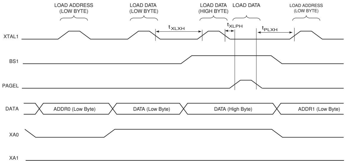
Note: 1. The timing requirements shown in Figure 26-5 (i.e.,  $t_{DVXH}$ ,  $t_{XHXL}$ , and  $t_{XLDX}$ ) also apply to loading operation.
