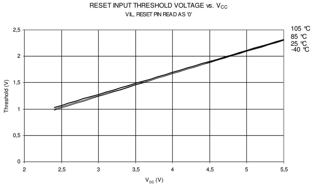
**Figure 27-24.** Reset Input Pin Hysteresis vs.  $V_{CC}$
