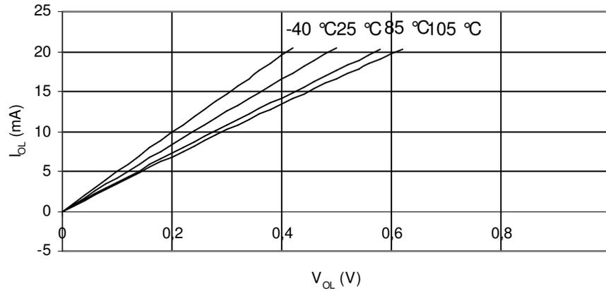
**Figure 27-19.** I/O Pin Sink Current vs. Output Voltage ( $V_{CC} = 2.7V$ )
