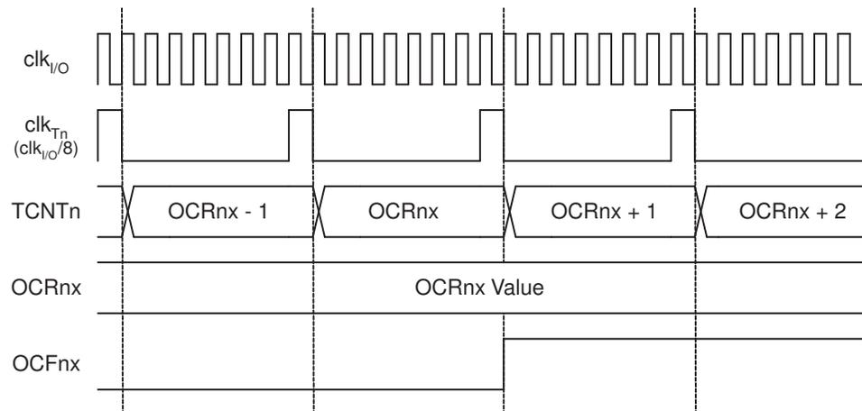
[Figure 15-12](#) shows the count sequence close to TOP in various modes. When using phase and frequency correct PWM mode the OCRnx Register is updated at BOTTOM. The timing diagrams will be the same, but TOP should be replaced by BOTTOM, TOP-1 by BOTTOM+1 and so on. The same renaming applies for modes that set the TOVn Flag at BOTTOM.
