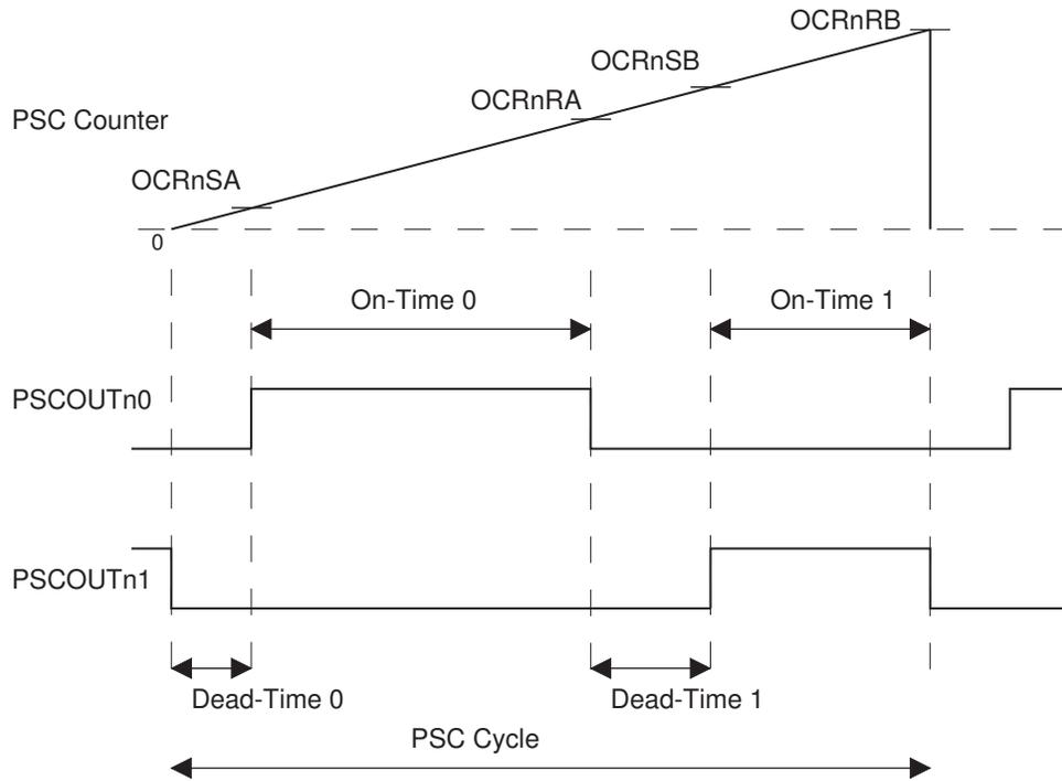
$$\text{On-Time 0} = (\text{OCRnRAH/L} - \text{OCRnSAH/L}) * 1/\text{Fclkpsc}$$
