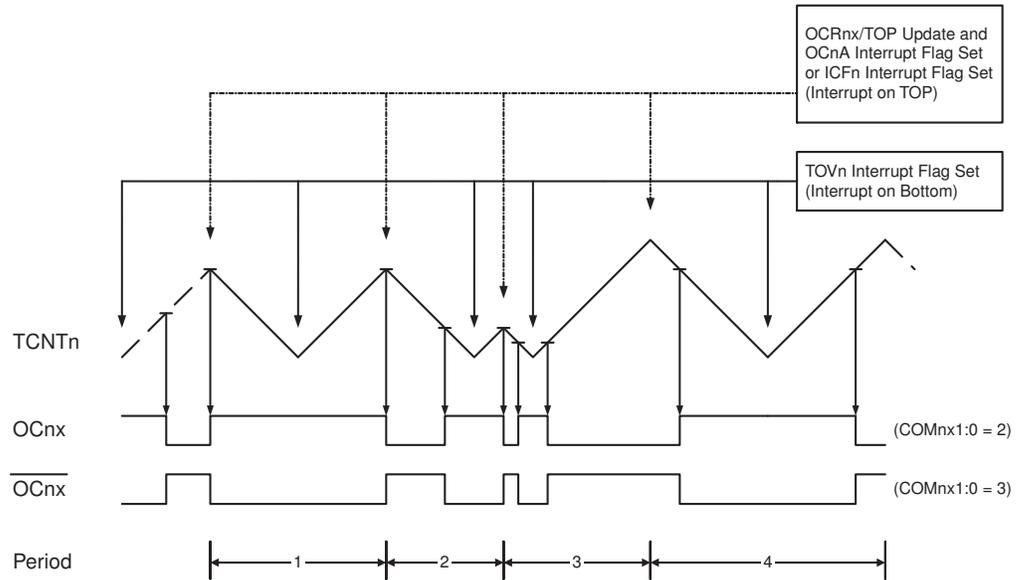
The Timer/Counter Overflow Flag (TOVn) is set each time the counter reaches BOTTOM. When either OCRnA or ICFn is used for defining the TOP value, the OCnA or ICFn Flag is set accordingly at the same timer clock cycle as the OCRnx Registers are updated with the double buffer value (at TOP). The Interrupt Flags can be used to generate an interrupt each time the counter reaches the TOP or BOTTOM value.
