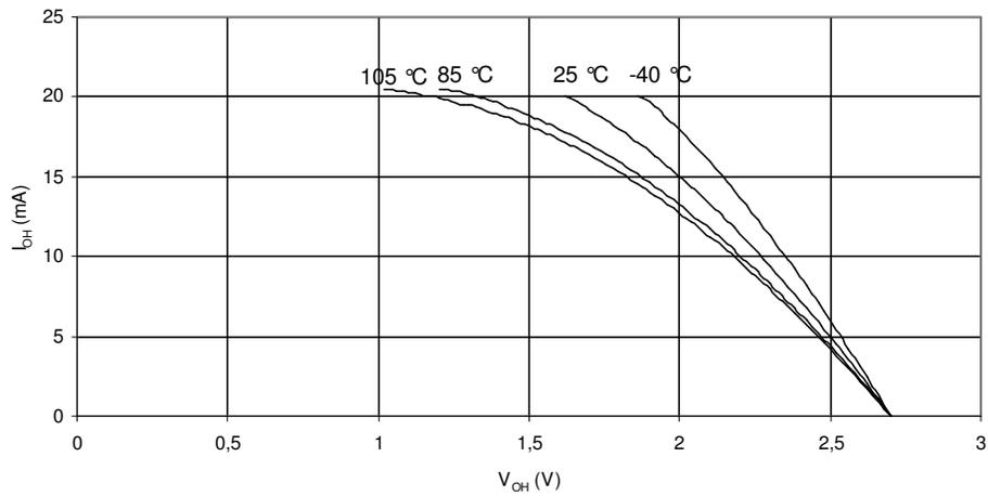
**Figure 27-18.** I/O Pin Sink Current vs. Output Voltage ( $V_{CC} = 5V$ )
