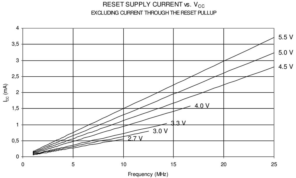
**Figure 27-46.** Reset Supply Current vs.  $V_{CC}$  (Clock Stopped, Excluding Current through the Reset Pull-up)
