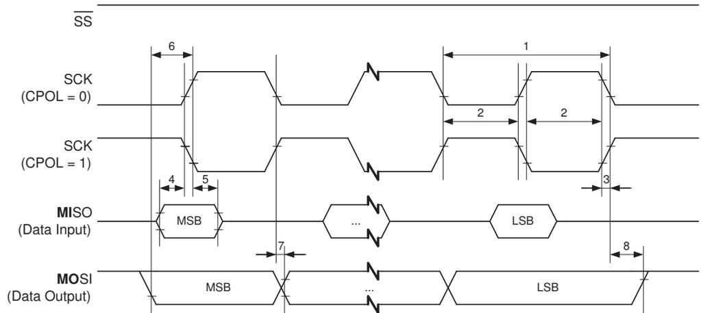
Figure 26-4. SPI Interface Timing Requirements (Slave Mode)
