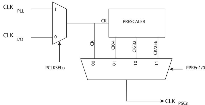
PCLKSEL<sub>n</sub> bit in PSC n Configuration register (PCNF<sub>n</sub>) is used to select the clock source.
