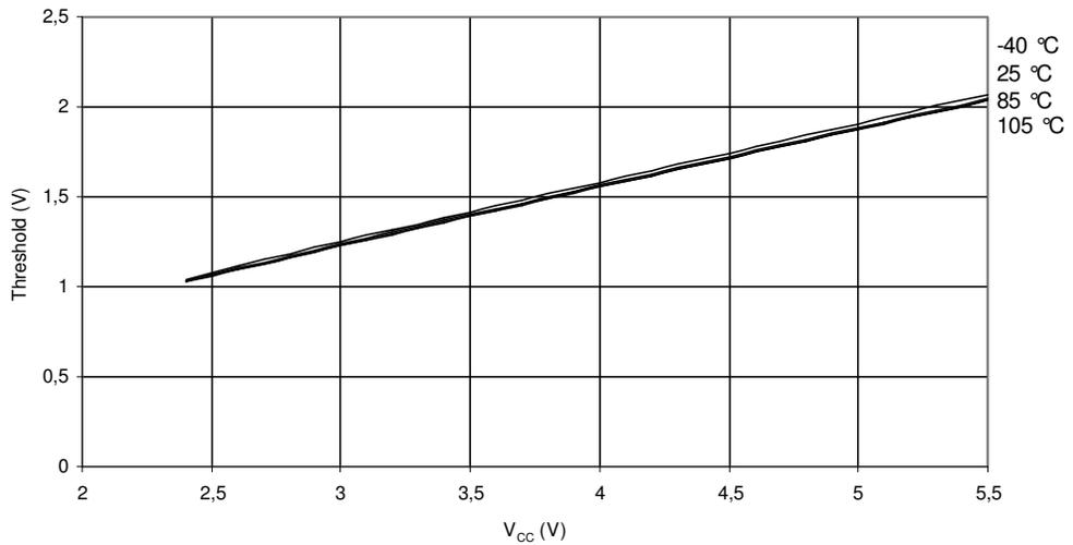
**Figure 27-21.** I/O Pin Input Threshold Voltage vs.  $V_{CC}$  (VIL, I/O Pin Read As '0')
