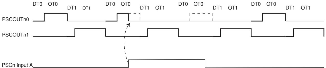
The output frequency is not modified by the occurrence of significant edge of retriggering input.
