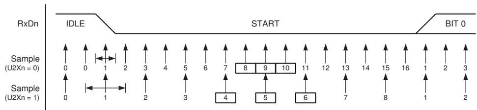
When the clock recovery logic detects a high (idle) to low (start) transition on the RxD line, the start bit detection sequence is initiated. Let sample 1 denote the first zero-sample as shown in the figure. The clock recovery logic then uses samples 8, 9, and 10 for Normal mode, and samples 4, 5, and 6 for Double Speed mode (indicated with sample numbers inside boxes on the figure), to decide if a valid start bit is received. If two or more of these three samples have logical
