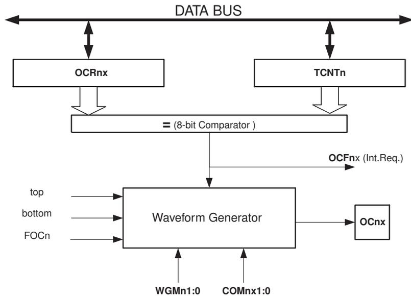
The OCR0x Registers are double buffered when using any of the Pulse Width Modulation (PWM) modes. For the normal and Clear Timer on Compare (CTC) modes of operation, the double buffering is disabled. The double buffering synchronizes the update of the OCR0x Compare Registers to either top or bottom of the counting sequence. The synchronization prevents the occurrence of odd-length, non-symmetrical PWM pulses, thereby making the output glitch-free.
