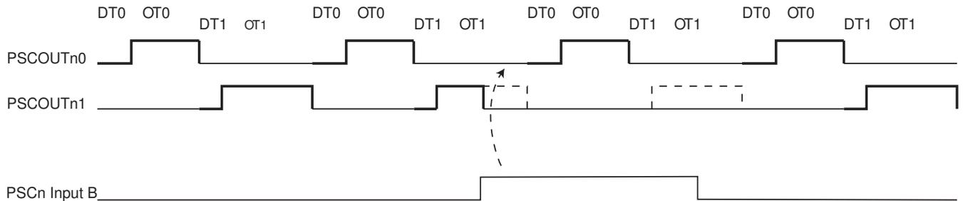
The output is deactivated while retriggering input is active.
