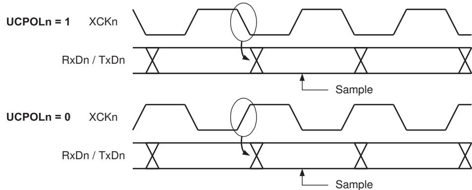
The UCPOL bit UCRSnC selects which XCK clock edge is used for data sampling and which is used for data change. As [Figure 18-3](#) shows, when UCPOL is zero the data will be changed at rising XCK edge and sampled at falling XCK edge. If UCPOL is set, the data will be changed at falling XCK edge and sampled at rising XCK edge.
