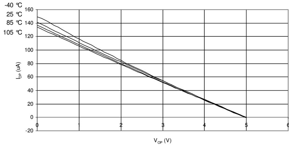
**Figure 27-13.** I/O Pin Pull-Up Resistor Current vs. Input Voltage ( $V_{CC} = 2.7V$ )
