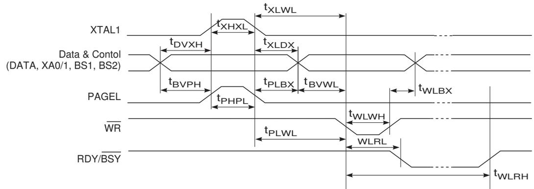
**Figure 26-6.** Parallel Programming Timing, Loading Sequence with Timing Requirements<sup>(1)</sup>
