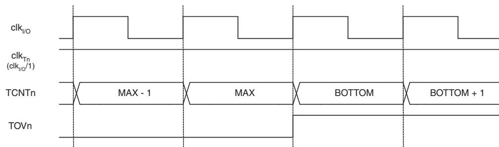
[Figure 14-9](#) shows the same timing data, but with the prescaler enabled.
