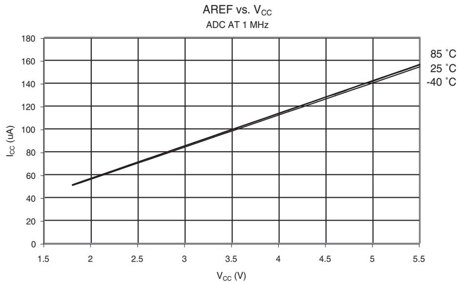
**Figure 27-42.** Analog Comparator Current vs.  $V_{CC}$
