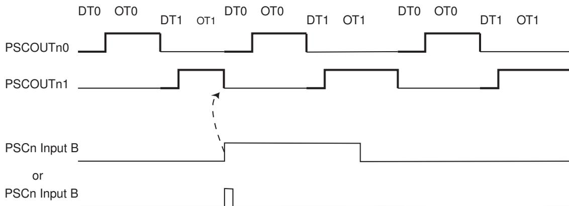
The output frequency is modulated by the occurrence of significant edge of retriggering input.
