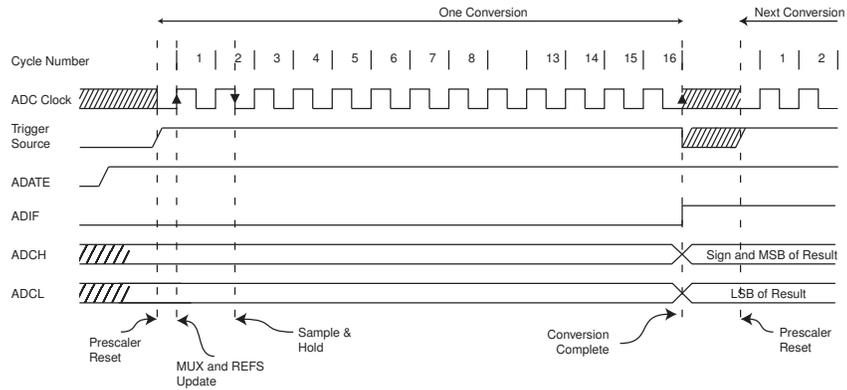
Figure 21-7. ADC Timing Diagram, Free Running Conversion
