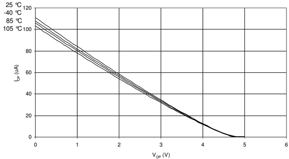
**Figure 27-15.** Reset Pull-Up Resistor Current vs. Reset Pin Voltage ( $V_{CC} = 2.7V$ )
