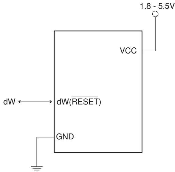
Figure 23-1 shows the schematic of a target MCU, with debugWIRE enabled, and the emulator connector. The system clock is not affected by debugWIRE and will always be the clock source selected by the CKSEL Fuses.
