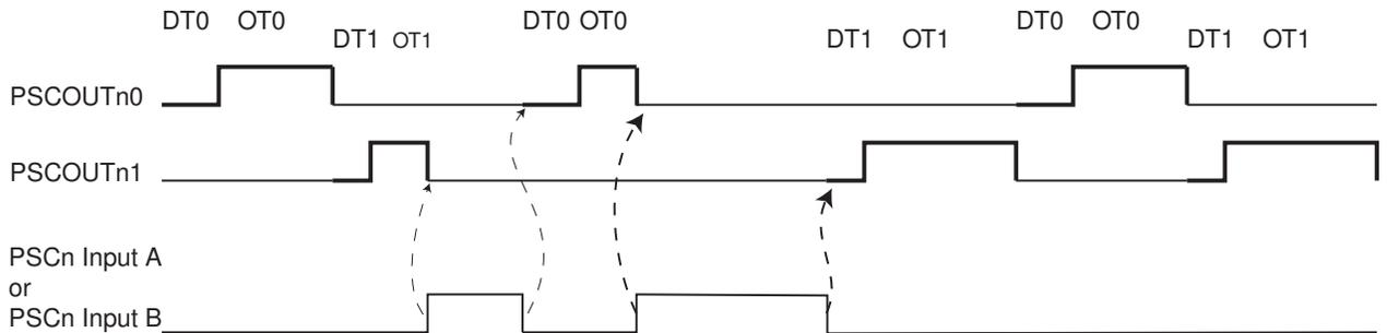
Used in Fault mode 6, PSCn Input A or PSCn Input B act indifferently on On-Time0/Dead-Time0 or on On-Time1/Dead-Time1.
