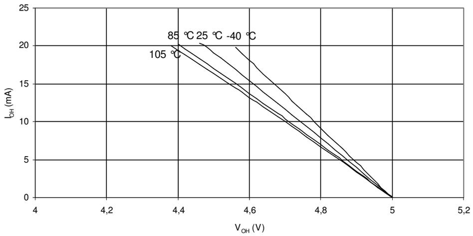
**Figure 27-17.** I/O Pin Source Current vs. Output Voltage ( $V_{CC} = 2.7V$ )
