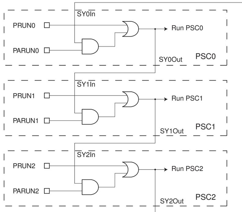
If the PSC<sub>m</sub> has its PARUN<sub>n</sub> bit set, then it can start at the same time than PSC<sub>n-1</sub>.
