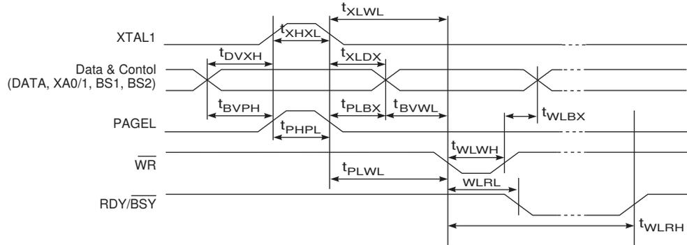
**Figure 25-8.** Parallel Programming Timing, Loading Sequence with Timing Requirements<sup>(1)</sup>
