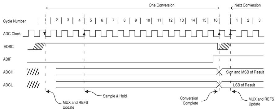
Figure 21-6. ADC Timing Diagram, Auto Triggered Conversion
