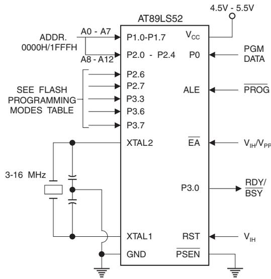
Figure 20-2. Verifying the Flash Memory (Parallel Mode)
