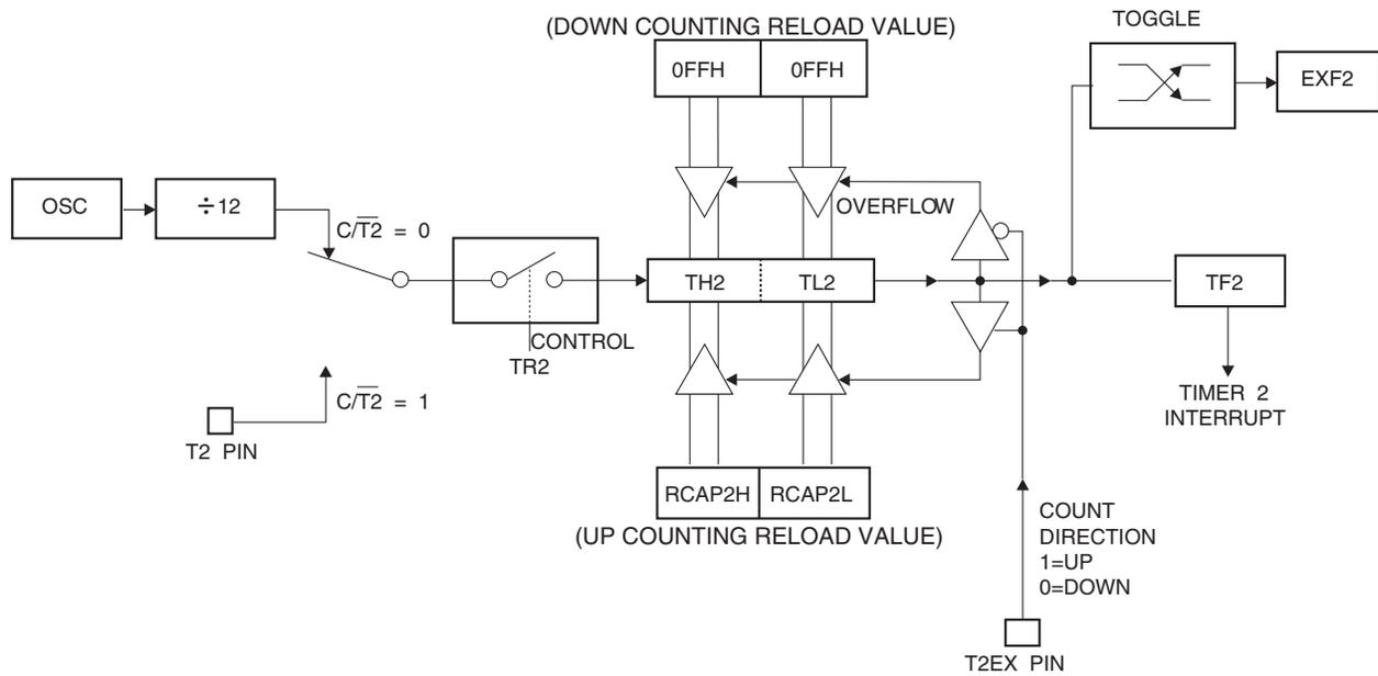
Figure 10-4. Timer 2 in Baud Rate Generator Mode
