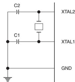
Note: C1, C2 = 30 pF  $\pm$  10 pF for Crystals
