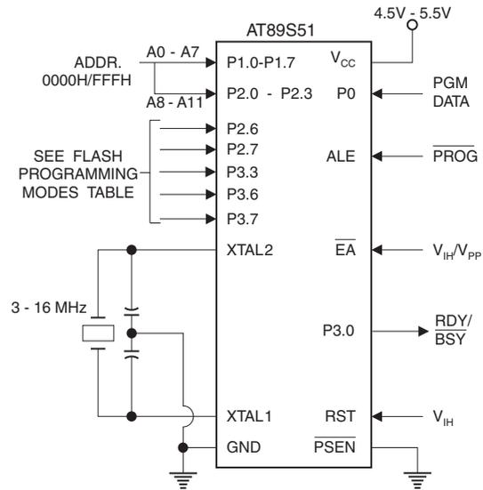
**Figure 17-2.** Verifying the Flash Memory (Parallel Mode)
