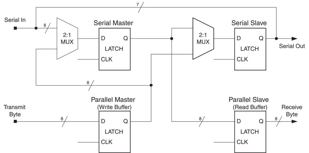
Figure 18-3. SPI Block Diagram
