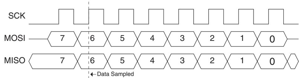
**Figure 23-10.** Serial Programming Interface Timing
