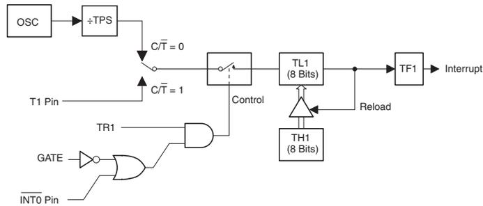
Note: RH1/RL1 are not required by Timer 1 during Mode 2 and may be used as temporary storage registers.
