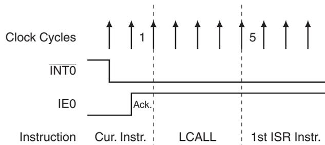
**Figure 12-2.** Maximum Interrupt Response Time
