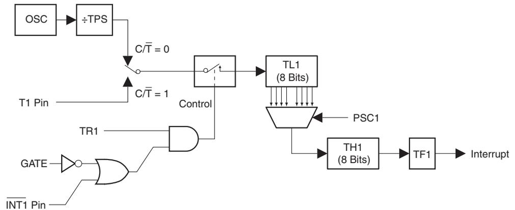
Mode 0 operation is the same for Timer 0 as for Timer 1, except that TR0, TF0 and  $\overline{\text{INT0}}$  replace the corresponding Timer 1 signals in Figure 14-1. There are two different GATE bits, one for Timer 1 (TMOD.7) and one for Timer 0 (TMOD.3). The  $\overline{\text{INT0}}$  and  $\overline{\text{INT1}}$  pins are shared with the XTAL oscillator. They may only be used for the GATE function when using the internal RC oscillator as the system clock.
