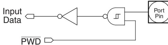
**Figure 13-3.** Input Only for P1.3, P3.2 and P3.3
