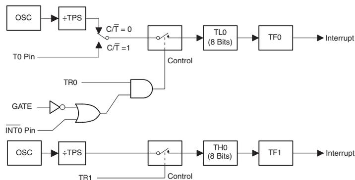
Note: RH0/RL0 are not required by Timer 0 during Mode 3 and may be used as temporary storage registers.
