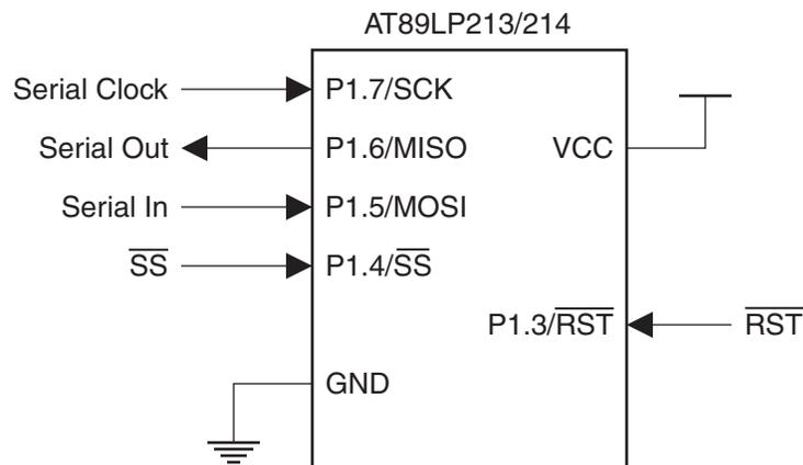
The In-System Programming Interface is the only means of externally programming the AT89LP213/214 microcontroller. The ISP Interface can be used to program the device both in-system and in a stand-alone serial programmer. The ISP Interface does not require any clock other than SCK and is not limited by the system clock frequency. During In-System programming the system clock source of the target device can operate normally.
