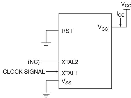
24.6.4  $I_{CC}$  Test Condition, Idle Mode, All Other Pins are Disconnected
