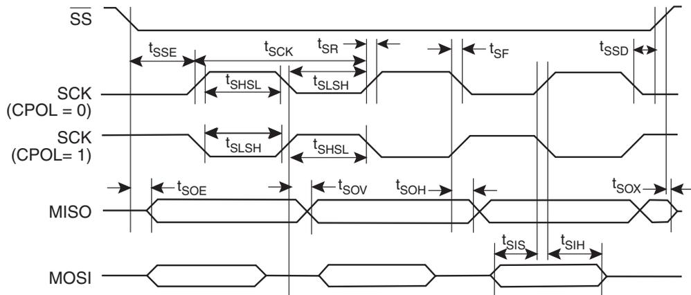
**Figure 24-3. SPI Master Timing (CPHA = 1)**
