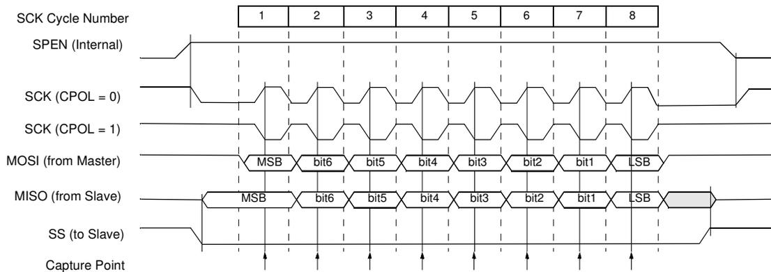
**Figure 47. Data Transmission Format (CPHA = 1)**
