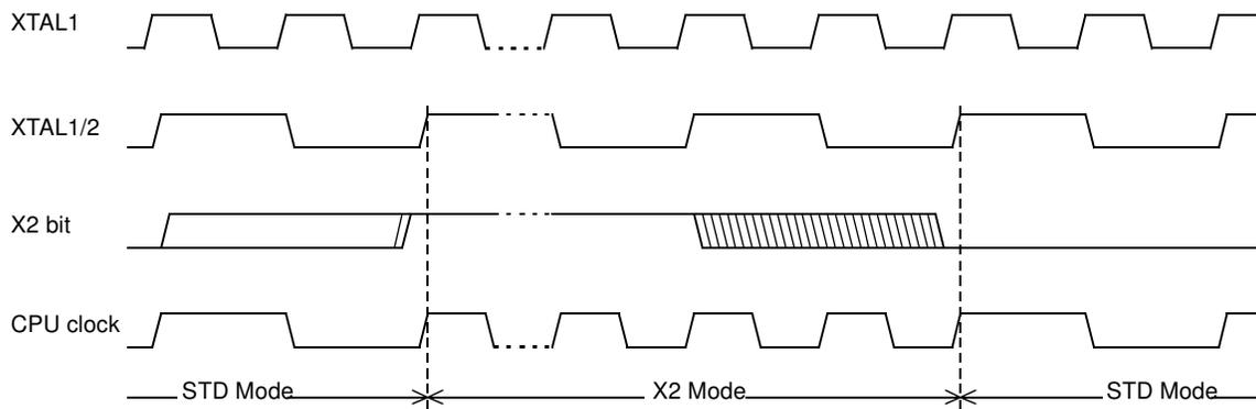
**Note:** In order to prevent any incorrect operation while operating in the X2 mode, users must be aware that all peripherals using the clock frequency as a time reference (UART, timers...) will have their time reference divided by two. For example a free running timer generating an interrupt every 20 ms will then generate an interrupt every 10 ms. A UART with a 4800 baud rate will have a 9600 baud rate.
