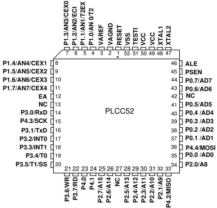
TESTI must be connected to VSS
