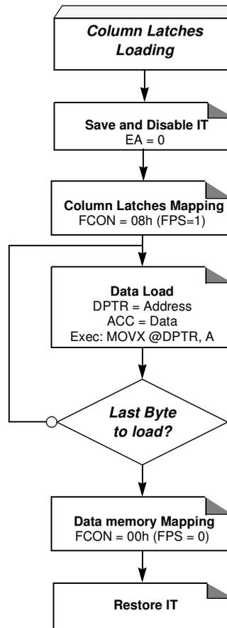
Note: The last page address used when loading the column latch is the one used to select the page programming address.
