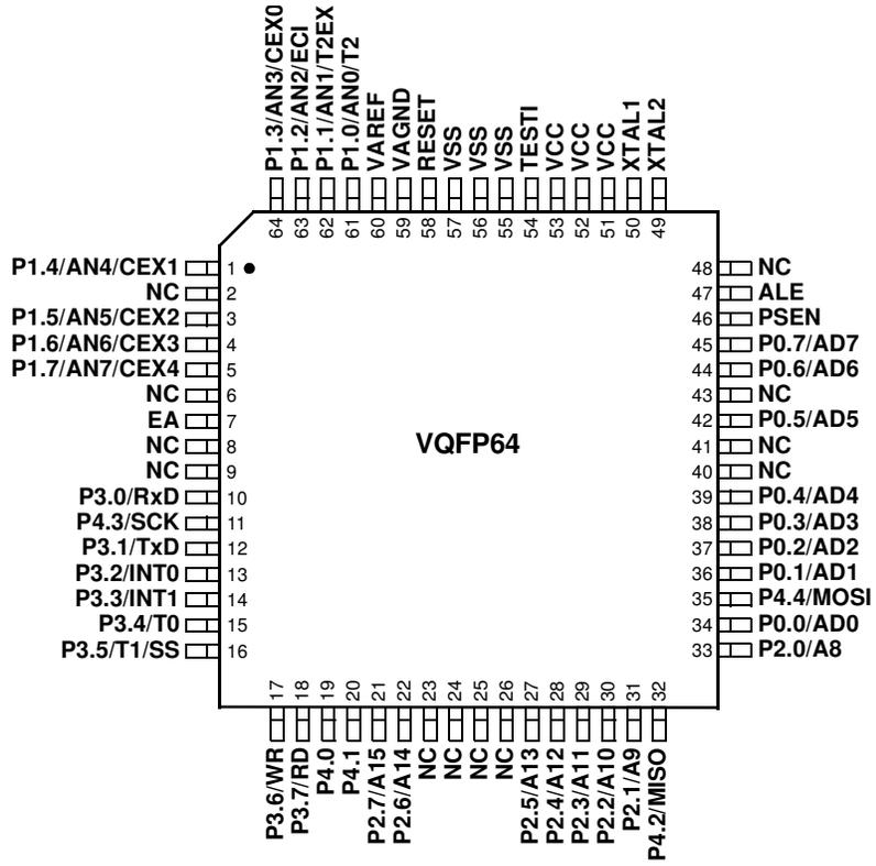
TESTI must be connected to VSS
