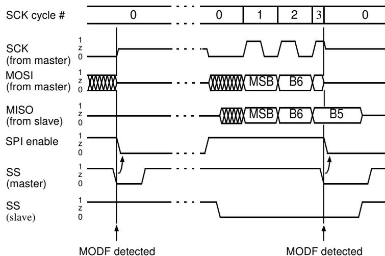
Note: When SS is discarded (SS disabled) it is not possible to detect a MODF error in master mode because the SPI is internally unselected and the SS pin is a general purpose I/O.
