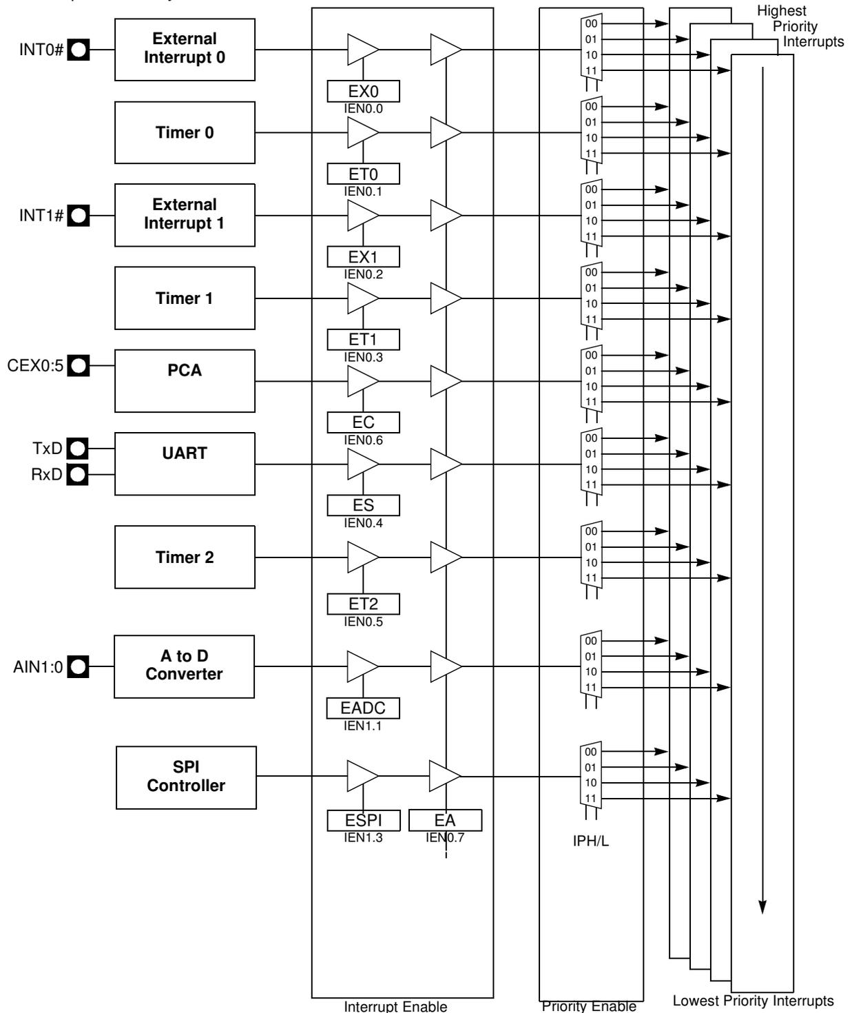
Each of the interrupt sources can be individually enabled or disabled by setting or clearing a bit in the Interrupt Enable register. This register also contains a global disable bit which must be cleared to disable all the interrupts at the same time.
