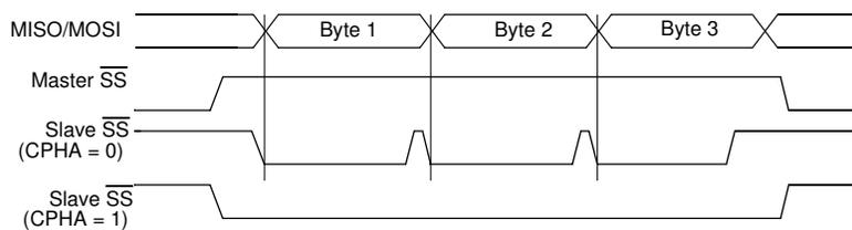
As shown in Figure 46, the first SCK edge is the MSB capture strobe. Therefore, the Slave must begin driving its data before the first SCK edge, and a falling edge on the  $\overline{SS}$  pin is used to start the transmission. The  $\overline{SS}$  pin must be toggled high and then low between each Byte transmitted (Figure 48).
