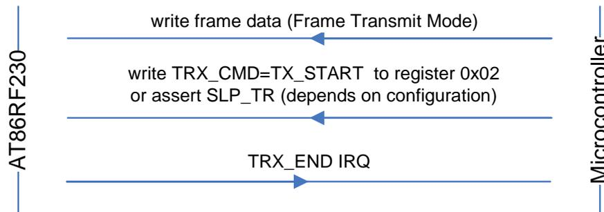
**Figure 6-9.** Packet Structure - Frame Transmit Mode
