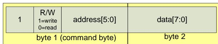
**Figure 6-4.** Example SPI Sequence - Register Access Mode
