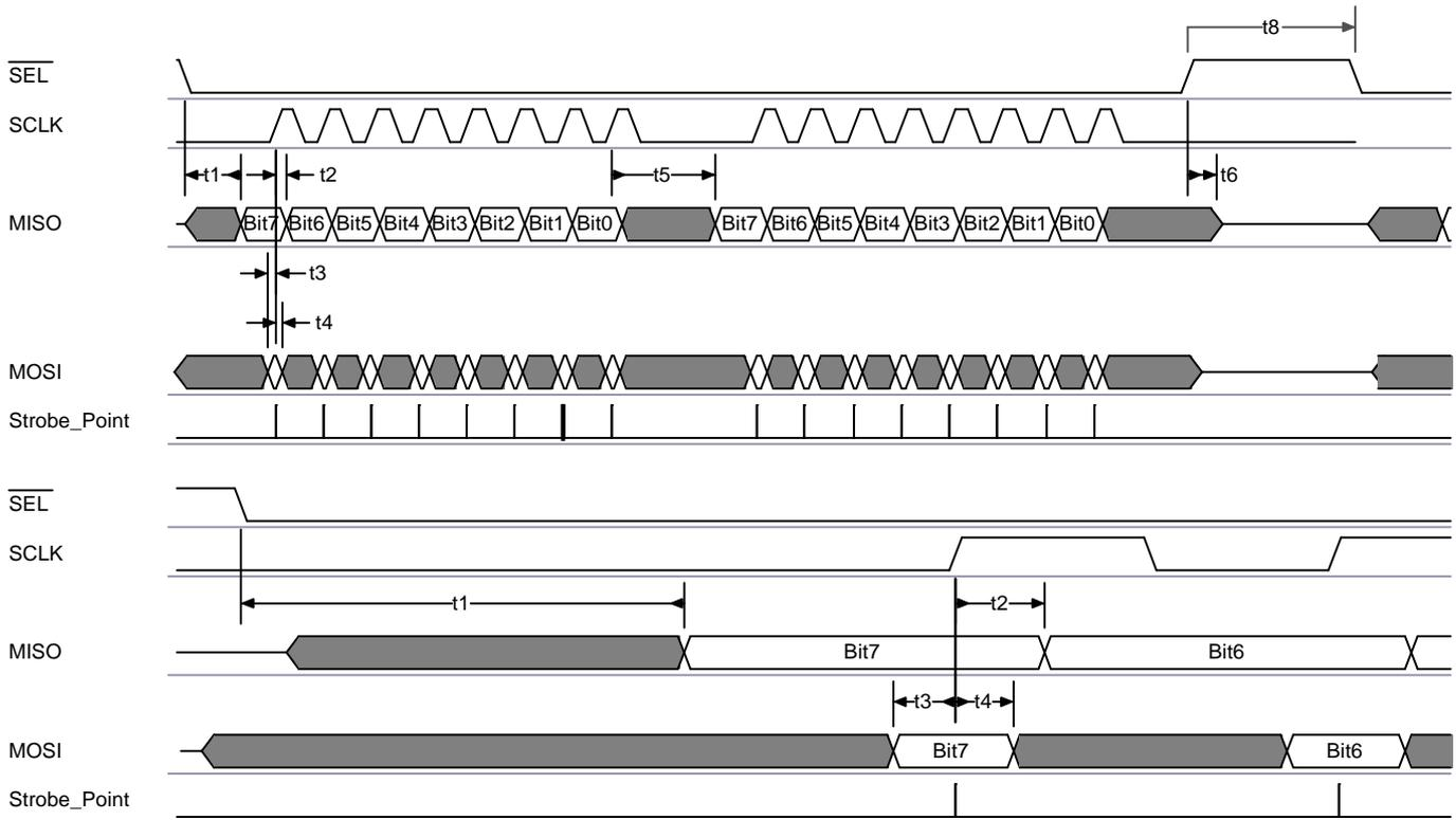
$\overline{\text{SEL}} = \text{L}$  enables the MISO output driver of the AT86RF230. If the driver is disabled, there is no internal pull-up resistor connected to it. Driving the appropriate signal level must be ensured by the master device or an external pull-up resistor.
