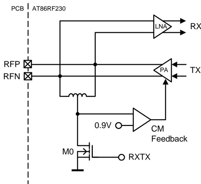
RF port DC values depend on the operating mode. In TRX\_OFF state (see section 7), the RF pins are pulled to ground, preventing a floating voltage larger than 1.8V which is not allowed for the internal circuitry. In receive mode, the RF input provides a low-impedance path to ground when transistor M0 (see **Figure 4-1**) pulls the inductor center tap to ground. A DC voltage drop of 20 mV across the on-chip inductor can be measured at the RF pins.
