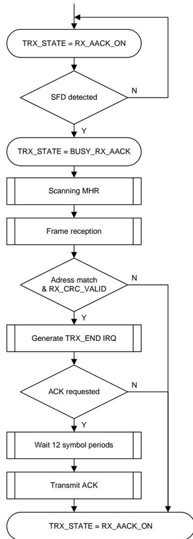
Figure 7-6. Example Timing of an RX\_AACK Transaction
