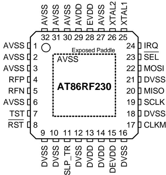
**Note:** The exposed paddle is electrically connected to the die inside the package. It shall be soldered to the board to ensure electrical and thermal contact and good mechanical stability.
