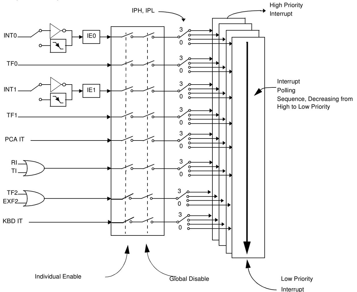
Each of the interrupt sources can be individually enabled or disabled by setting or clearing a bit in the Interrupt Enable register (Table 12-5 and Table 12-3). This register also contains a global disable bit, which must be cleared to disable all interrupts at once.
