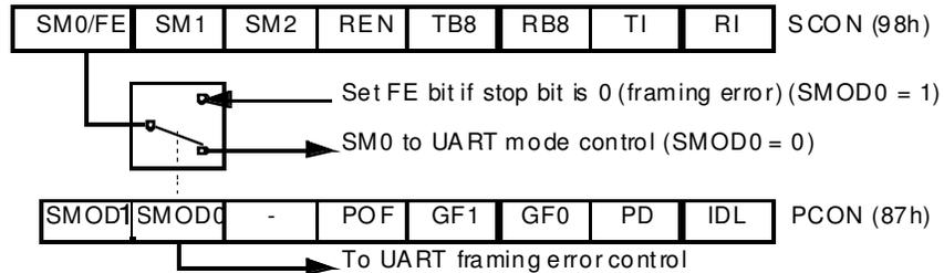
When this feature is enabled, the receiver checks each incoming data frame for a valid stop bit. An invalid stop bit may result from noise on the serial lines or from simultaneous transmission by two CPUs. If a valid stop bit is not found, the Framing Error bit (FE) in SCON register (see [Table 11-4](#)) bit is set.
