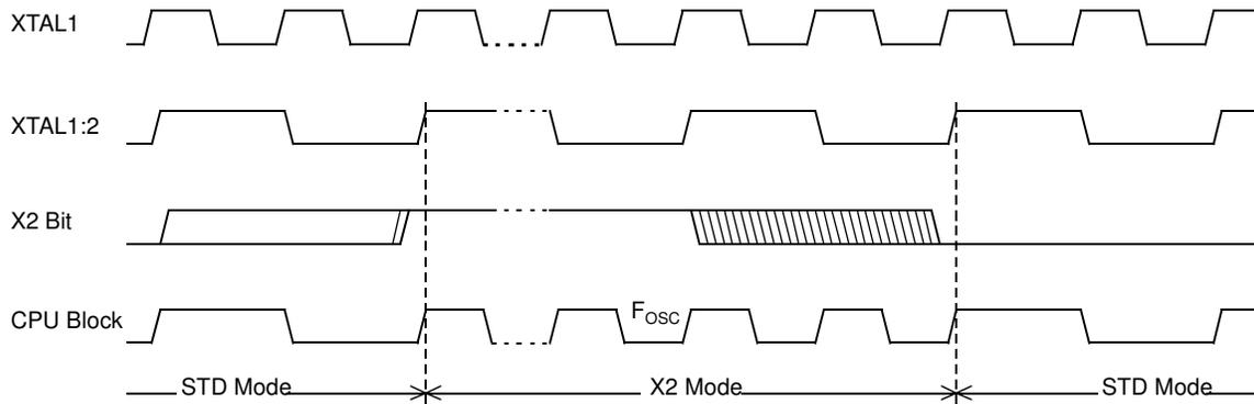
The X2 bit in the CKCON0 register (see Table 6-1) allows to switch from 12 clock periods per instruction to 6 clock periods and vice versa. At reset, the speed is set according to X2 bit of Hardware Config Byte (HCB). By default, Standard mode is activated. Setting the X2 bit activates the X2 feature (X2 mode).
