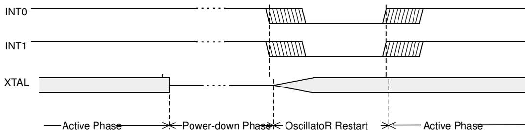
Exit from power-down by reset redefines all the SFRs, exit from power-down by external interrupt does not affect the SFRs.
