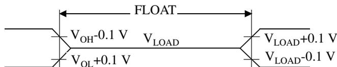
**Figure 14-12.** Float Waveforms
