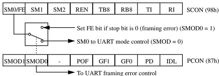
When this feature is enabled, the receiver checks each incoming data frame for a valid stop bit. An invalid stop bit may result from noise on the serial lines or from simultaneous transmission by two CPUs. If a valid stop bit is not found, the Framing Error bit (FE) in SCON register (See Table 9-3.) bit is set.
