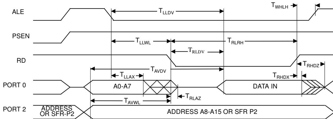
**Figure 14-8.** External Data Memory Read Cycle
