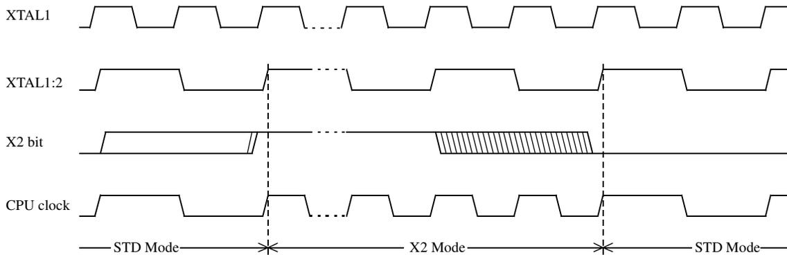
The X2 bit in the CKCON register (See Table 6-1.) allows to switch from 12 clock cycles per instruction to 6 clock cycles and vice versa. At reset, the standard speed is activated (STD mode). Setting this bit activates the X2 feature (X2 mode).
