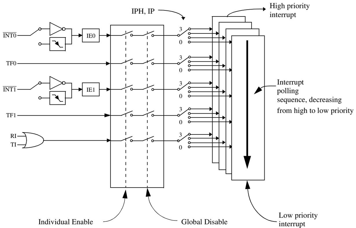
Each of the interrupt sources can be individually enabled or disabled by setting or clearing a bit in the Interrupt Enable register (See Table 10-2. Table 10-3.). This register also contains a global disable bit, which must be cleared to disable all interrupts at once.
